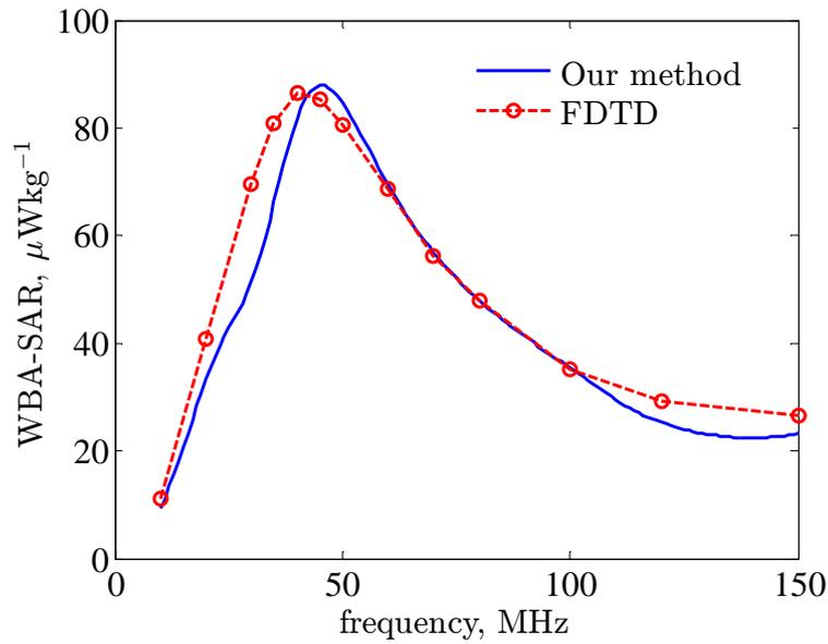
FIGURE 5.3: Comparison of the WBA-SAR calculated using the equivalent cylindrical antenna and using FDTD on the adult female voxel model for  $E_0 = 1 \text{ Vm}^{-1}$  r.m.s..
