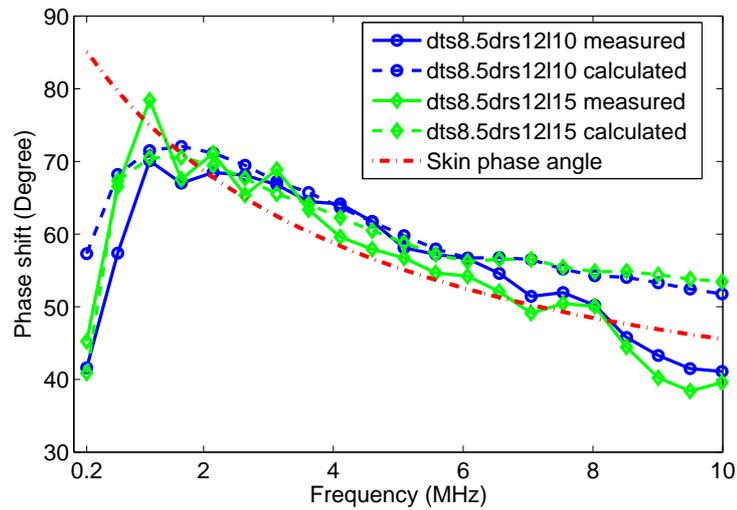
FIGURE 3.15: Phase shift measurement and corresponding calculation results on subject 1. The electrodes are placed on different location highlighting the relationship among different measurement parameters. The plot **dts8.5drs12l10** is phase shift for the case of  $d_{ts}=8.5$  cm,  $d_{rs}=12$  cm and  $l=10$  cm. And the plot **dts8.5drs12l15** is phase shift for the case of  $d_{ts}=8.5$  cm,  $d_{rs}=12$  cm, and  $l=15$  cm. The plot in broken line is impedance phase angle of skin.
