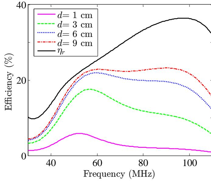
FIGURE 6.6: The theoretical radiation efficiency  $\eta_r$  and the total efficiency  $\eta_t$  for different thicknesses  $d$  of the dielectric slab ( $\epsilon=3$ , area=  $22 \times 30 \text{ cm}^2$ ) placed underneath the cylindrical monopole antenna representing a human subject of height  $h=1.76 \text{ m}$  and weight  $m=73 \text{ kg}$ .
