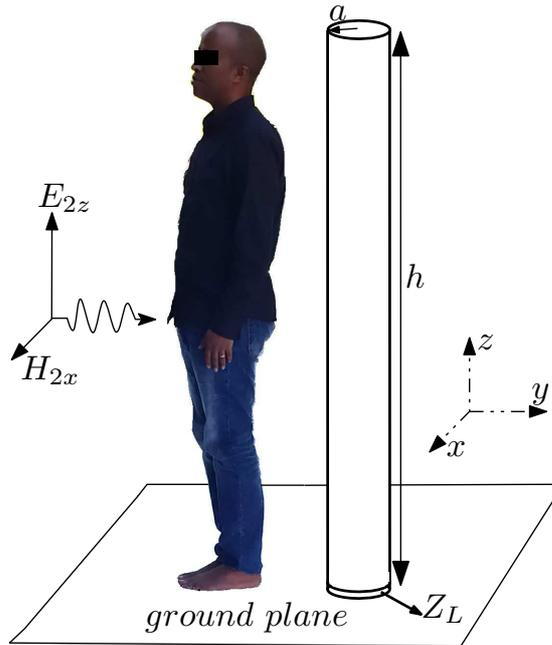
FIGURE 4.1: Cylindrical antenna model of the human body exposed to vertically polarised plane wave [53].
