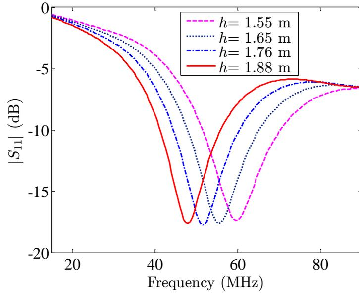
FIGURE 6.8: Comparison of the calculated reflection coefficients for cylindrical monopole antennas representing human subjects of different height and the same body-mass-index of 23.56.
