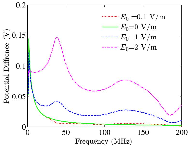
(b) Effect of  $|E_0|$  on the potential difference at  $z = h/2 - 0.3$  from the transmitter located at  $z = h/2$
