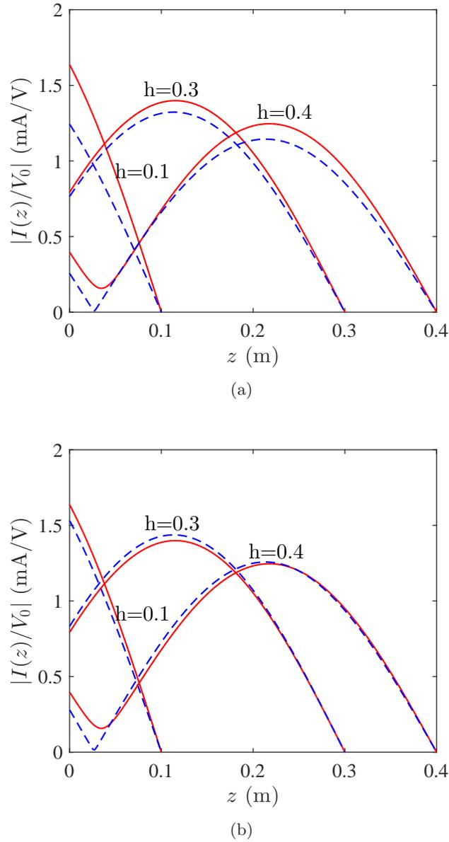
FIGURE A.1: Comparison of the proposed current expression with that of the three-term expression for a cylindrical dipole of radius  $a = 0.001$  cm and skin-depth to radius ratio of 0.1 at 400 MHz. (a) Compares the current in (A.36) (broken line) to the three-term expression (A.37) (solid line) for the half-length  $h$  of 0.4, 0.3 and 0.1 m. (b) Compares the first sinusoidal term (broken line) and the complete three-terms (solid line) in (A.37).
