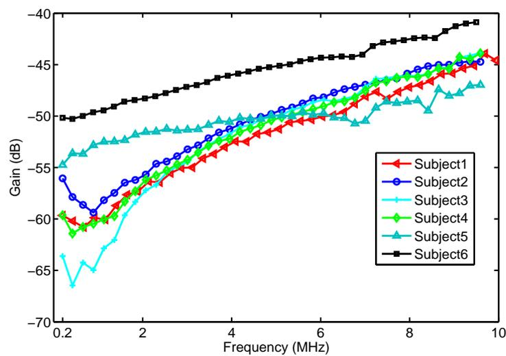
FIGURE 3.11: Measured gain (dB) as a function of frequency for six subjects.
