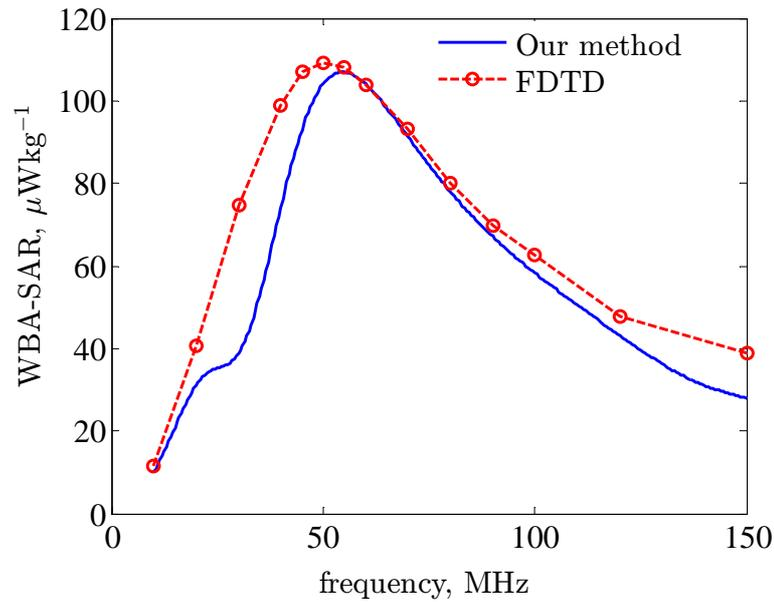
FIGURE 5.4: Comparison of the WBA-SAR calculated using the equivalent cylindrical antenna and using FDTD on the 10 years old child voxel model for  $E_0 = 1 \text{ Vm}^{-1}$  r.m.s..
