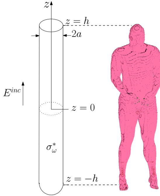
FIGURE B.1: The cylindrical antenna model of the human body exposed to vertically polarised plane wave.
