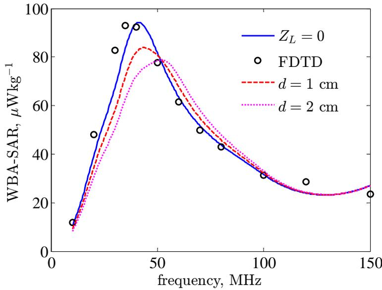
FIGURE 5.6: The effect of load due to inserting rubber of thickness  $d$  1 and 2 cm at the base of the equivalent cylindrical antenna representing NORMAN.
