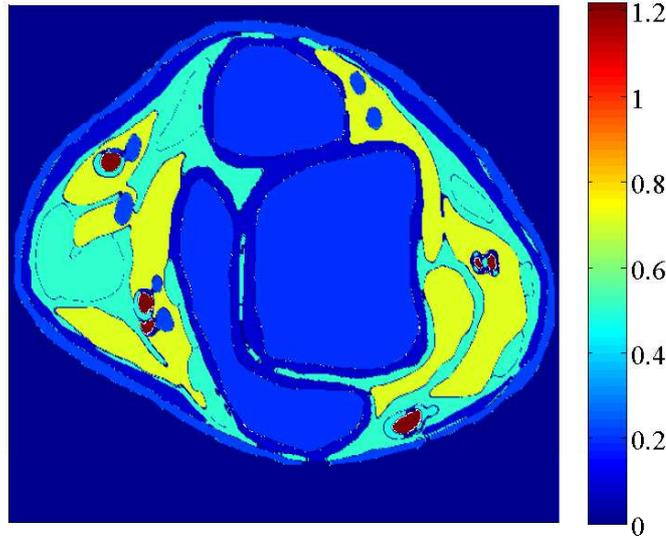
FIGURE 7.2: The magnitude of axial current density  $|J_z^n|$  (A/m<sup>2</sup>) in the cross-section of the ankle joint for an incident electric field  $E_0 = 1$  V/m r.m.s and the total cross-section area of the ankle was taken as 0.0154 m<sup>2</sup>.
