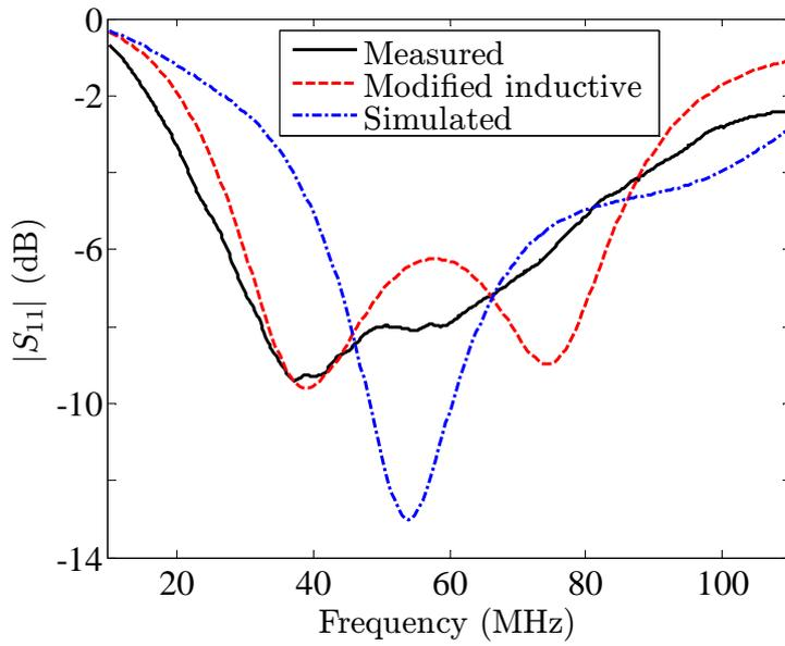
FIGURE 6.13: Comparison of the measured reflection coefficient with the simulation results. The modified simulation represents the reflection coefficient calculated after adding a series inductive reactance representing the unshielded Copper core. The thickness of rubber layer used was 9 cm.
