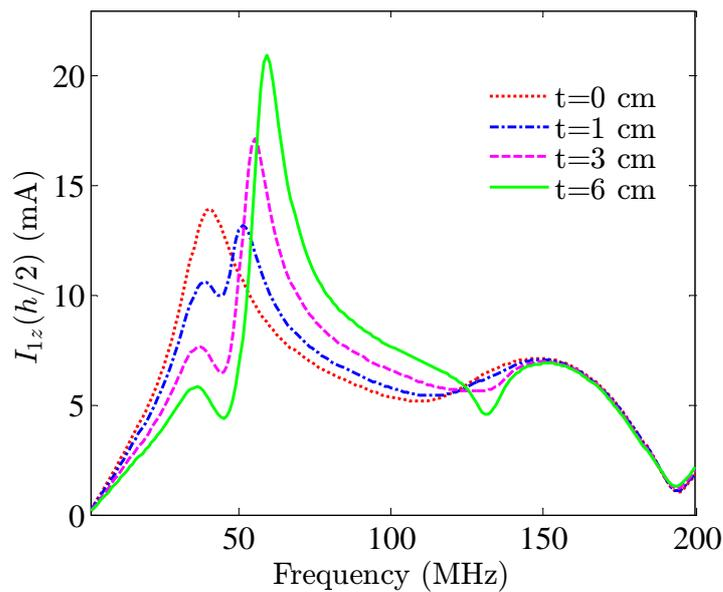
(b)  $I_{1z}(h/2)$  for different thickness of the rubber sole
