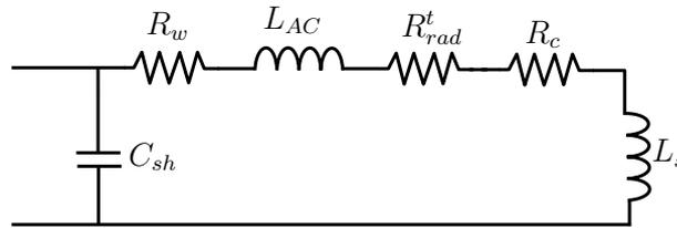
FIGURE 7.4: The equivalent circuit of the toroidal inductor.  $C_{sh}$  is the parasitic capacitance between turns;  $R_w$  represents the loss in winding wire;  $L_{AC}$  is the internal inductance of the wire;  $R_{rad}^t$  is the radiation resistance of the toroid;  $R_c$  represents the magnetic core loss; and  $L_s$  is the self-inductance.
