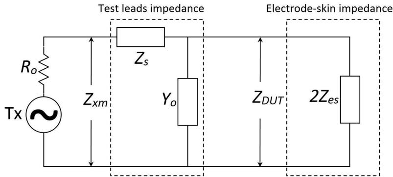
FIGURE 3.7: The circuit diagram proposed to calculate the electrode-skin impedance.  $Z_{xm}$  is impedance seen by the VNA port,  $Z_s$  and  $Y_o$  are series residual impedance and stray admittance of test leads;  $Z_{DUT}$  is input impedance of the arm with electrodes attached;  $Z_{es}$  is electrode-skin impedance; and  $R_o$  is the output impedance of the VNA.
