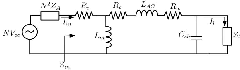
FIGURE 7.8: The simplified equivalent circuit of the implanted toroidal inductor in receiving mode.  $V_{oc}$  is the open-circuit voltage driving the current through the area enclosed by the toroid and  $Z_L$  is impedance of the load connected to the terminals of the toroid.
