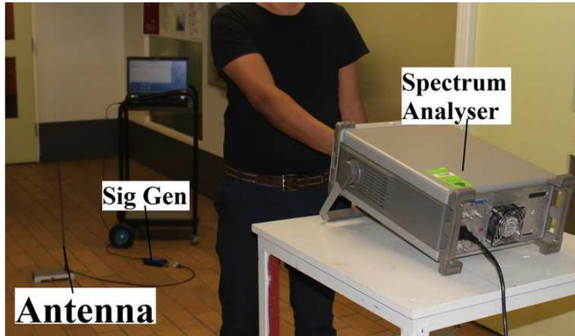
(a) Current measurement setup
