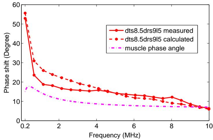
FIGURE 3.14: Phase shift measurement and corresponding calculation results on subject 1 for the case **dts8.5drs9l5**,  $d_{ts} > l$ , which is  $d_{ts}=8.5$  cm,  $d_{rs}=9$  cm and  $l=5$  cm. And the plot in broken line is impedance phase angle for muscle.
