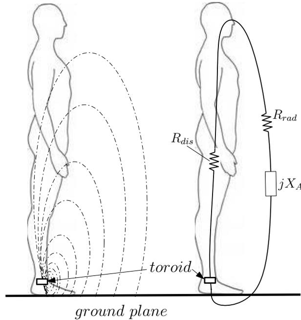
FIGURE 7.6: Visualisation of the lines of force in the human body forming the secondary loop, which is represented by the human antenna impedance,  $Z_A = R_{rad} + R_{dis} + jX_A$ , where  $R_{rad}$  characterizes the power radiated  $P_{rad}$ ;  $R_{dis}$  characterizes the power dissipated inside the human body due to ohmic and dielectric loss of tissues; and  $X_A$  characterizes the near-field reactive power oscillating in the vicinity of the human body.
