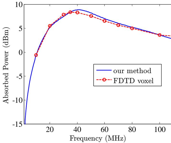
FIGURE 6.2: Comparison of the calculation results of the total absorbed RF power in the body of a grounded human subject of  $h=1.76$  m and weight  $m=73$  kg for an incident electric field  $E_0$  of 1 V/m r.m.s.
