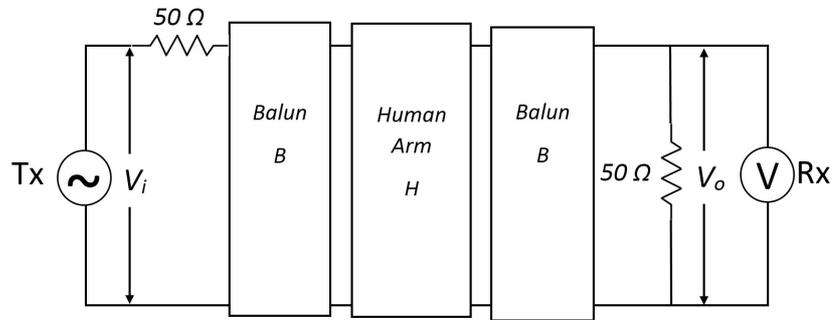
FIGURE 3.10: Block diagram of the measurement set-up.  $B$  is half of the measured insertion loss of the baluns and cables; and  $H$  is gain (in dB) of human arm and electrodes.  $V_i$  is the input voltage and  $V_o$  is the potential difference detected.
