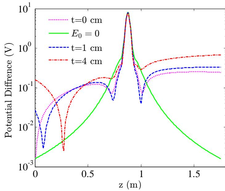
(a) Electric potential difference on the surface of the cylinder for different thickness of the rubber sole
