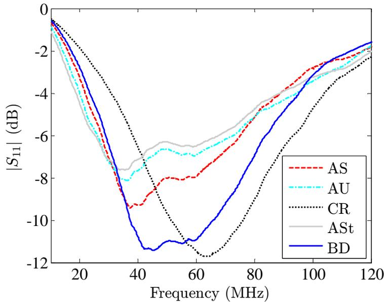
FIGURE 6.14: The measured reflection coefficient when the subject posed different postures. *AS*= arms by side, *AU*= arms raised up, *CR*= crouching, *ASt*= arms stretched out, and *BD*= bending down. The thickness of rubber layer used was 9 cm.
