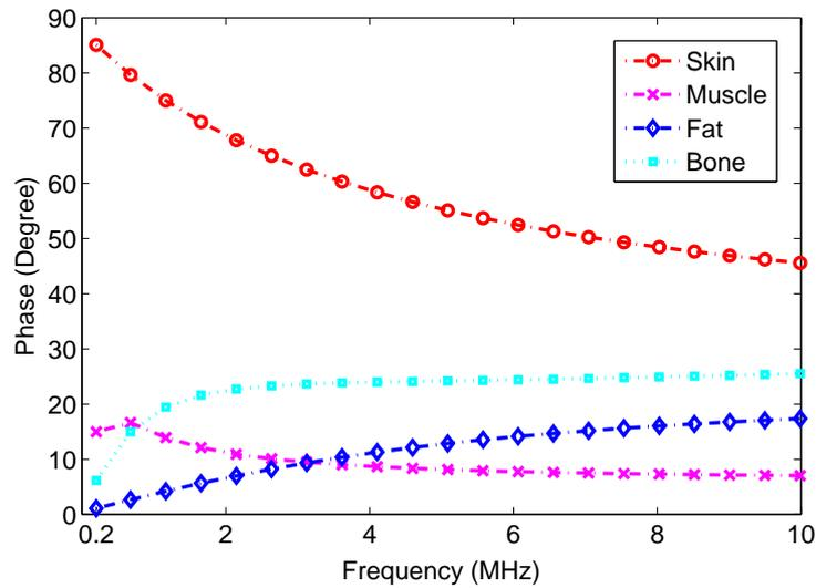
FIGURE 3.3: Impedance phase angle (degree) as function of frequency for tissues in the upper arm.
