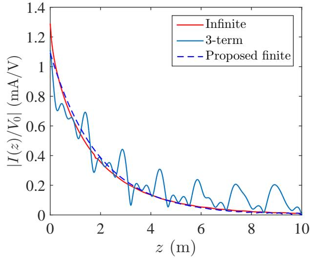
FIGURE A.3: Comparison of the proposed current for finite dipole (A.36), the three-term approximation (A.37) and the infinitely-long dipole (A.59). The finite dipole has a height  $h = 10$  m, radius  $a = 0.01$  cm and  $b = \delta_s/a = 1$ ; and the infinite dipole has the same radius and conductivity.
