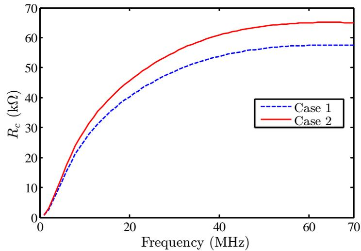
FIGURE 7.11: The magnetic core resistance  $R_c$  for the two cases. The toroid in Case 1 is smaller than that of Case 2.
