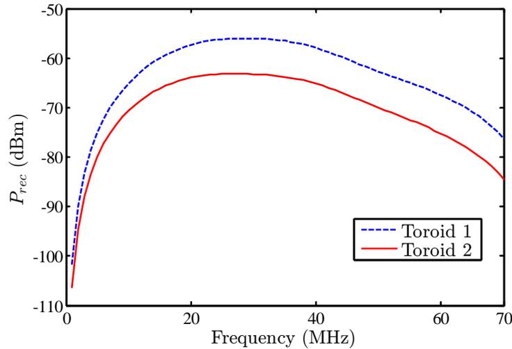
FIGURE 7.14: The calculated received power  $P_{rec}$  for the two cases for a source of 0 dBm EIRP located at a distance of  $d = \lambda/2\pi$  m.
