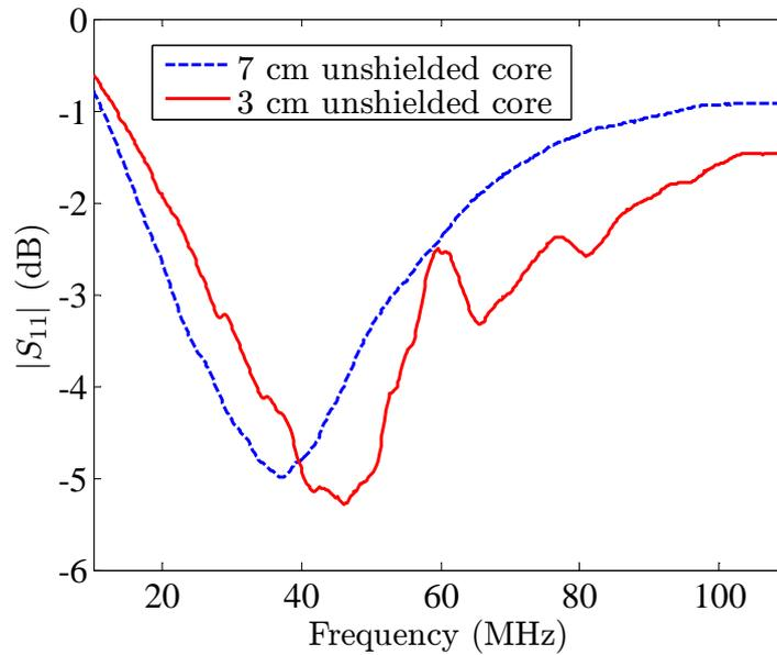
FIGURE 6.12: Comparison of the effect of varying the length of the unshielded Copper on the measured reflection coefficient. The thickness of the rubber layer used was 3 cm.
