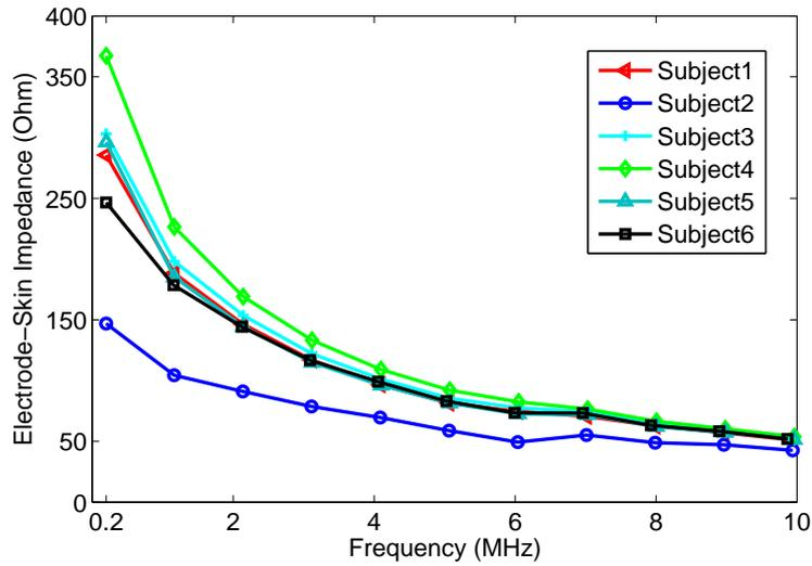
FIGURE 3.8: Normalized electrode-skin impedance modulus (for electrode area of  $1 \text{ cm}^2$ ), in  $\Omega$ , as a function of frequency, calculated based on impedance measurements on six subjects. The electrodes used are pregelled Ag/AgCl electrodes.
