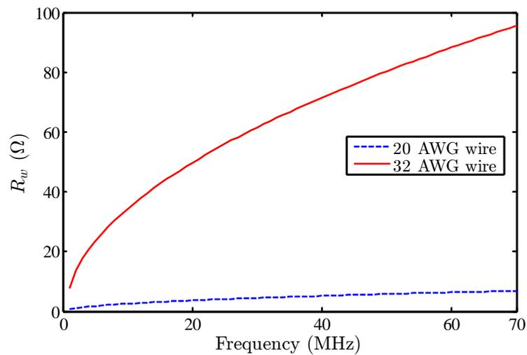
FIGURE 7.12: The wire resistance  $R_w$  for the case of two different wires of radius 0.1 mm (32 AWG) and 0.4 mm (20 AWG).
