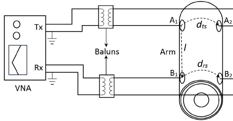
FIGURE 3.9: Measurement set-up for galvanic coupling IBC using the human upper arm as transmission path.
