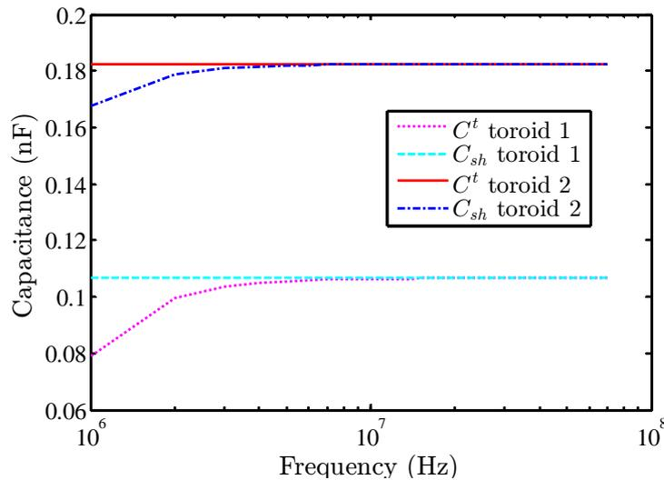
FIGURE 7.13: The parasitic capacitance  $C_{sh}$  and the equivalent capacitance  $C^t$  of the two cases.
