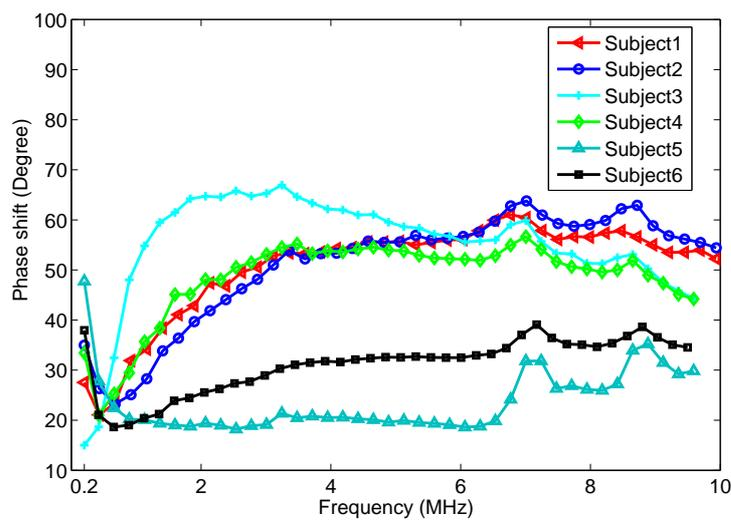
FIGURE 3.12: Measured phase shift (degree) as a function of frequency for six subjects.
