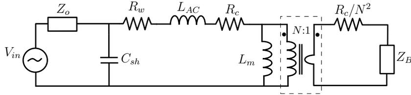
FIGURE 7.5: The equivalent circuit of the implanted toroidal inductor.  $V_{in}$  is the input voltage of the transmitter;  $Z_o$  is the output impedance of the transmitter;  $L_m$  is the magnetising inductance referred to the primary side; and  $Z_B$  is the impedance representing the effect of the human body and the surrounding.
