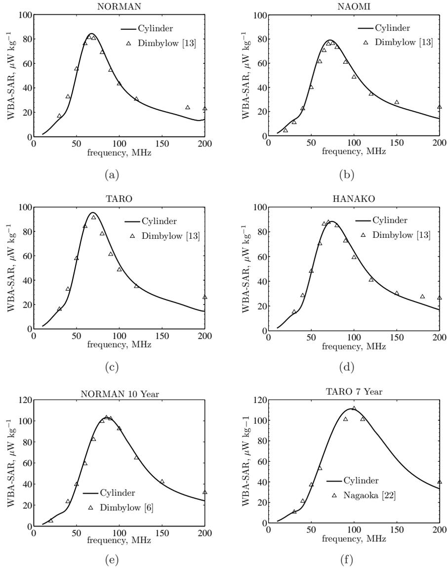
FIGURE B.2: WBA-SAR from the cylindrical model (solid line) and the FDTD computed on voxel models by other authors (triangle markers) for an incident field  $E^{inc} = \sqrt{2} \text{ Vm}^{-1}$  ( $1 \text{ Vm}^{-1}$  r.m.s.).
