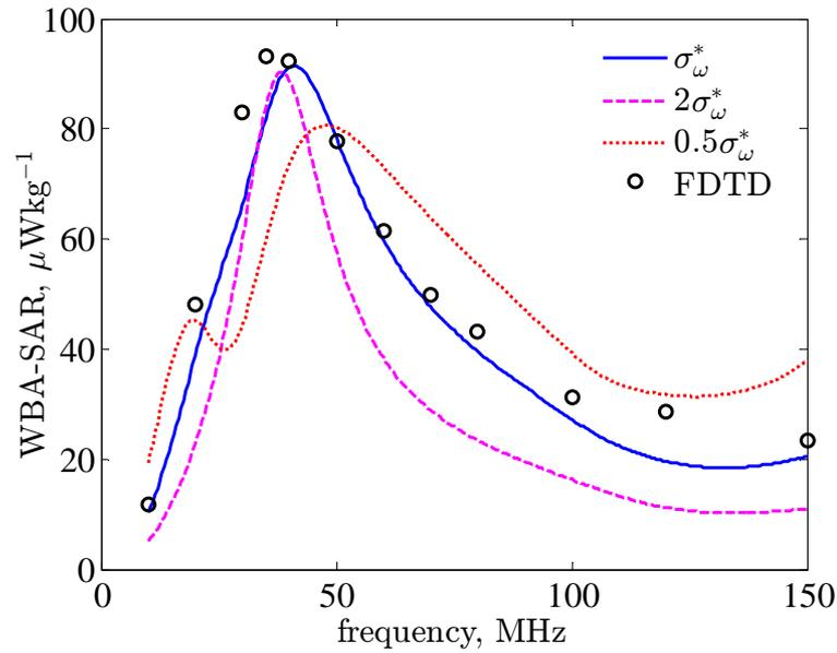
FIGURE 5.5: Comparison of the WBA-SAR calculated for different values of the complex conductivity.
