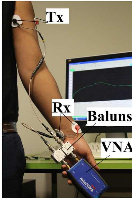
(a) Gain measurement setup
