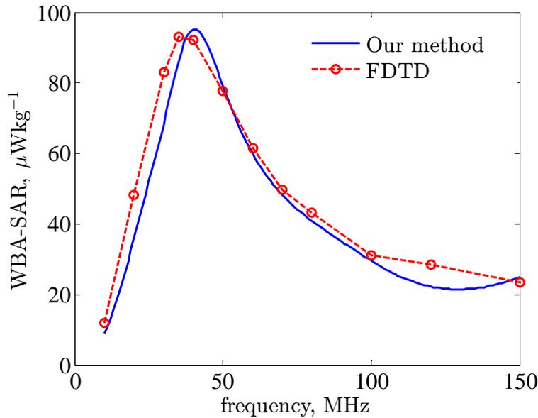
FIGURE 5.2: Comparison of the WBA-SAR calculated using the equivalent cylindrical antenna and using FDTD on the adultmale voxel model for  $E_0 = 1 \text{ Vm}^{-1}$  r.m.s..
