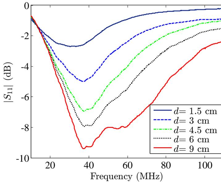
FIGURE 6.11: The measured reflection coefficient for different thicknesses of the rubber layers ( $\epsilon=3$ , area=  $22 \times 30$  cm<sup>2</sup>) placed underneath the human subject.
