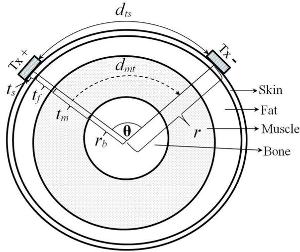
FIGURE 3.5: Cross-section of the upper arm abstraction along the transverse axis at the transmitter location.  $t_s$  is skin thickness,  $t_f$  fat thickness,  $t_m$  muscle thickness,  $r_b$  bone radius,  $r$  radius of the arm,  $d_{ts}$  inter-electrode distance,  $d_{mt}$  transverse path length of muscle, and  $\theta$  radian angle formed by the two electrodes of the transmitter .
