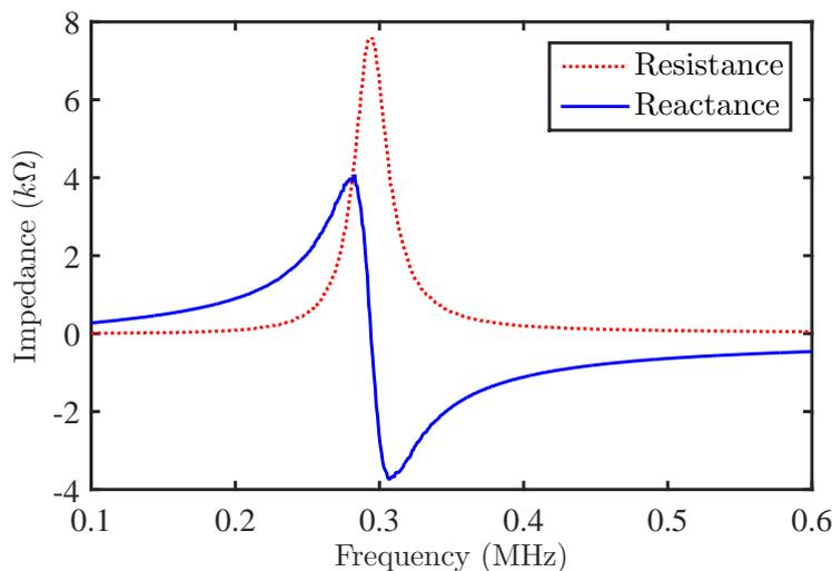
FIGURE 7.17: The measured impedance of the toroidal inductor.
