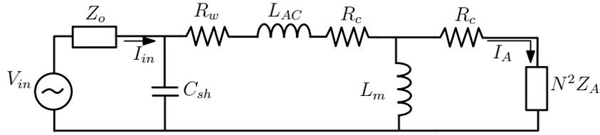
FIGURE 7.7: The simplified equivalent circuit of the implanted toroidal inductor in transmitting mode.
