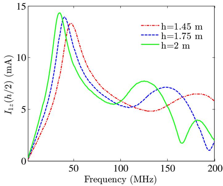
(a)  $I_{1z}(h/2)$  for different height of cylinder
