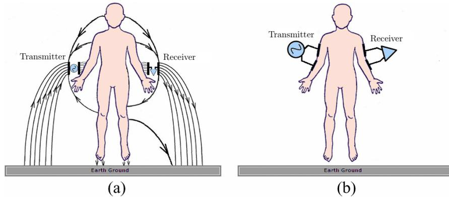
FIGURE 1.1: The two types of HBC. (a) is capacitive coupled and (b) is galvanic coupled
