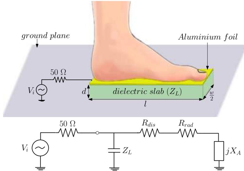
FIGURE 6.3: The diagram shows the typical setup of feeding the human body as a cylindrical monopole antenna and its corresponding equivalent circuit representation. A single foot is shown for clarity.
