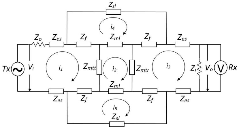
FIGURE 3.4: A simplified equivalent circuit representation of the upper arm for galvanic coupling type IBC, for the case of gelled electrodes, where  $Z_o$  is output impedance of the transmitter;  $Z_i$  is input impedance of receiver and the  $i_1$  to  $i_5$  are the mesh currents
