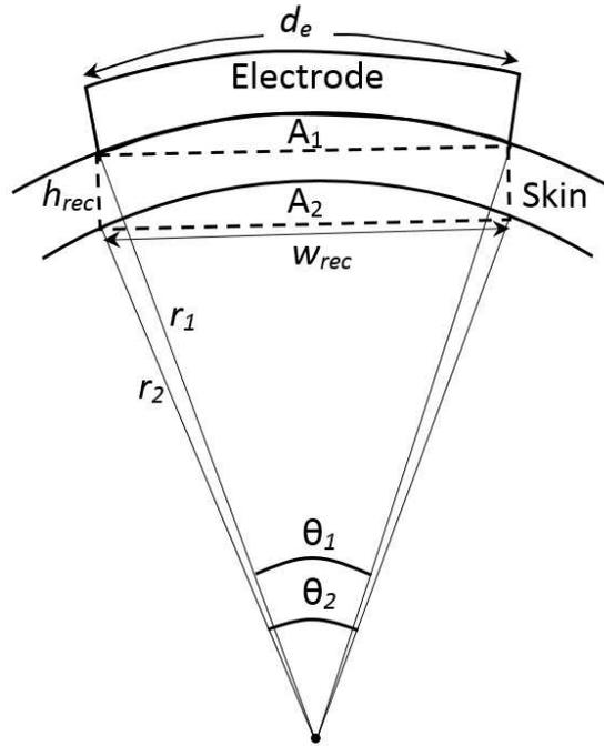
FIGURE 3.6: The cross-section of the arm where electrode is attached.  $r_1$  is radius of upper arc,  $r_2$  radius of lower arc,  $\theta_1$  central angle for the upper arc in radian,  $\theta_2$  central angle for the lower arc in radian,  $A_1$  is area of the upper circular segment,  $A_2$  is area of the lower circular segment,  $h_{rec}$  height of the rectangle,  $w_{rec}$  width of the rectangle and  $d_e$  electrode diameter.
