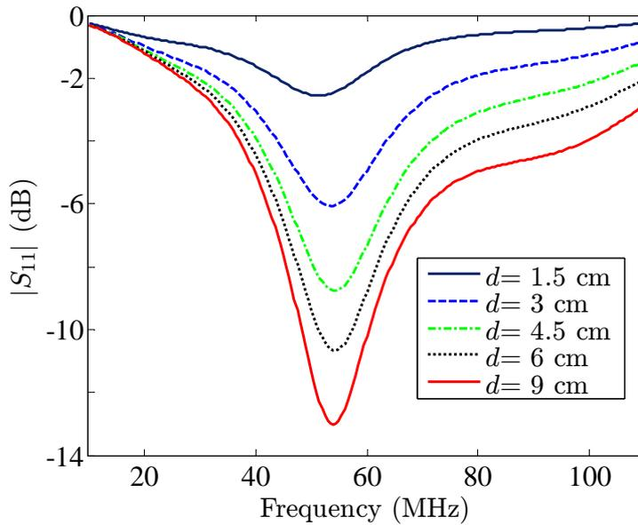
FIGURE 6.9: Comparison of the calculated reflection coefficients for different thicknesses  $d$  of the dielectric slab ( $\epsilon=3$ , area=  $22 \times 30$  cm<sup>2</sup>) placed underneath a cylindrical monopole antenna representing a human subject of height  $h=1.76$  m and weight  $m=73$  kg.
