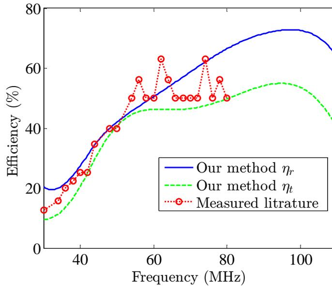
FIGURE 6.7: Comparison of  $\eta_r$  and  $\eta_t$  with the measured radiation efficiency found in [21].  $\eta_t$  was calculated based on the experimental setting in the literature;  $Z_0=50\ \Omega$ , parameter for  $Z_L$  are  $\epsilon=1$ ,  $A=\pi(0.15)^2\ \text{m}^2$ , and  $d=0.1\ \text{m}$ .
