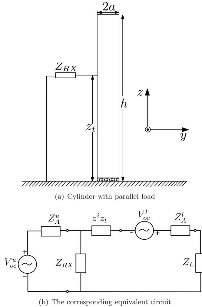
FIGURE 4.2: Human body cylinder model with externally embedded HBC receiver
