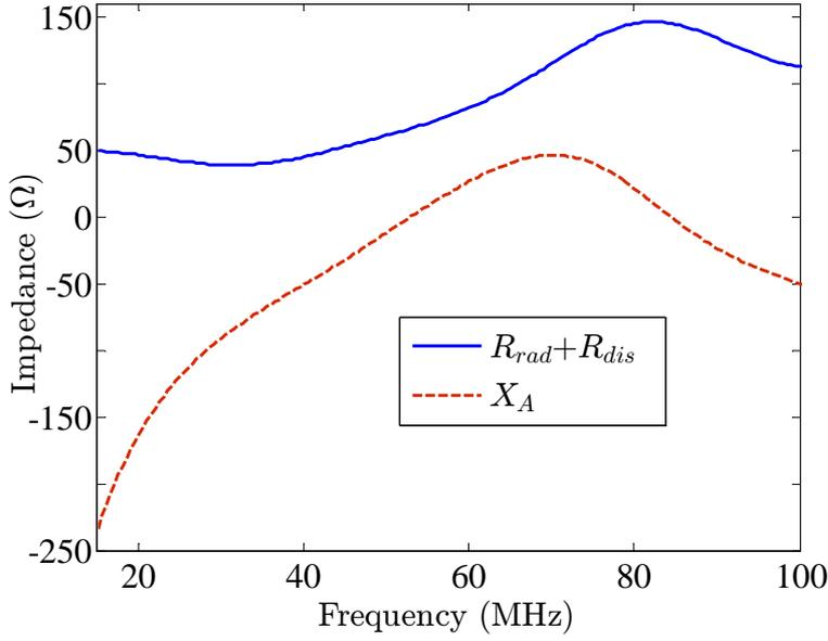
FIGURE 6.4: The antenna impedance  $Z_A$  calculated for a cylindrical monopole antenna representing a human subject of height  $h=1.76$  cm and weight  $m=73$  kg.
