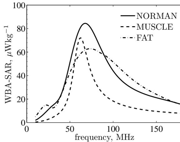
FIGURE B.4: Comparison of different dielectric properties for the cylindrical model
