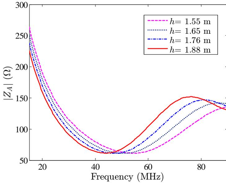
FIGURE 6.5: The magnitude of antenna impedance versus height of the cylindrical monopole antenna representing different human subjects that have the same body-mass-index of 23.56.
