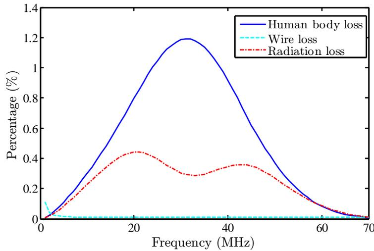
FIGURE 7.10: The power loss percentage in the human body, the wire and the radiated power.
