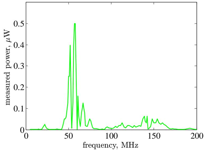
FIGURE 5.7: The measured power when a subject is illuminated by electromagnetic field touching an electrode attached to spectrum analyzer.
