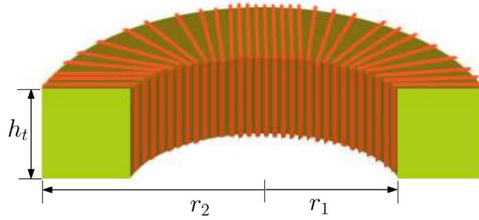
FIGURE 7.3: The half-section of the implanted toroidal inductor with ferrite core.
