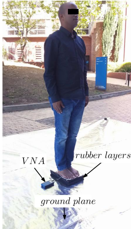
FIGURE 6.10: The experiment setup with a human subject of height  $h= 1.76$  m and weight  $m= 73$  kg.
