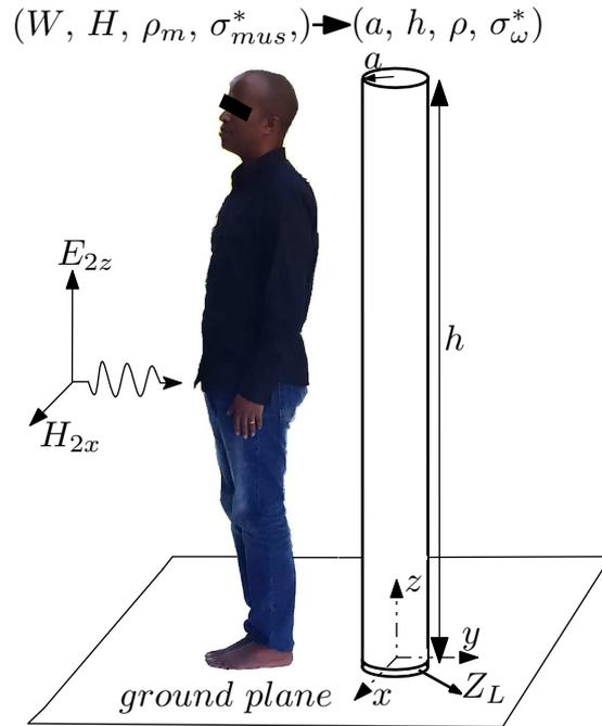
FIGURE 5.1: The equivalent cylindrical antenna representation of a grounded human body [53].
