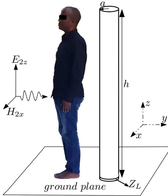
FIGURE 6.1: The equivalent cylindrical monopole antenna of a person standing on a highly conductive ground.  $Z_L$  is the load impedance due to the space (shoes) between the foot and the ground.
