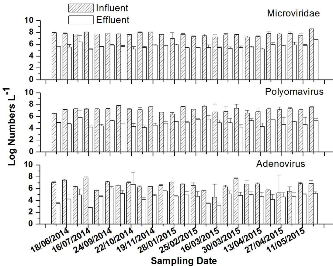
Figure 6-7. Comparative adenovirus, polyomavirus and *Microviridae* numbers in influent and effluent samples collected from Rosny WWTP.
