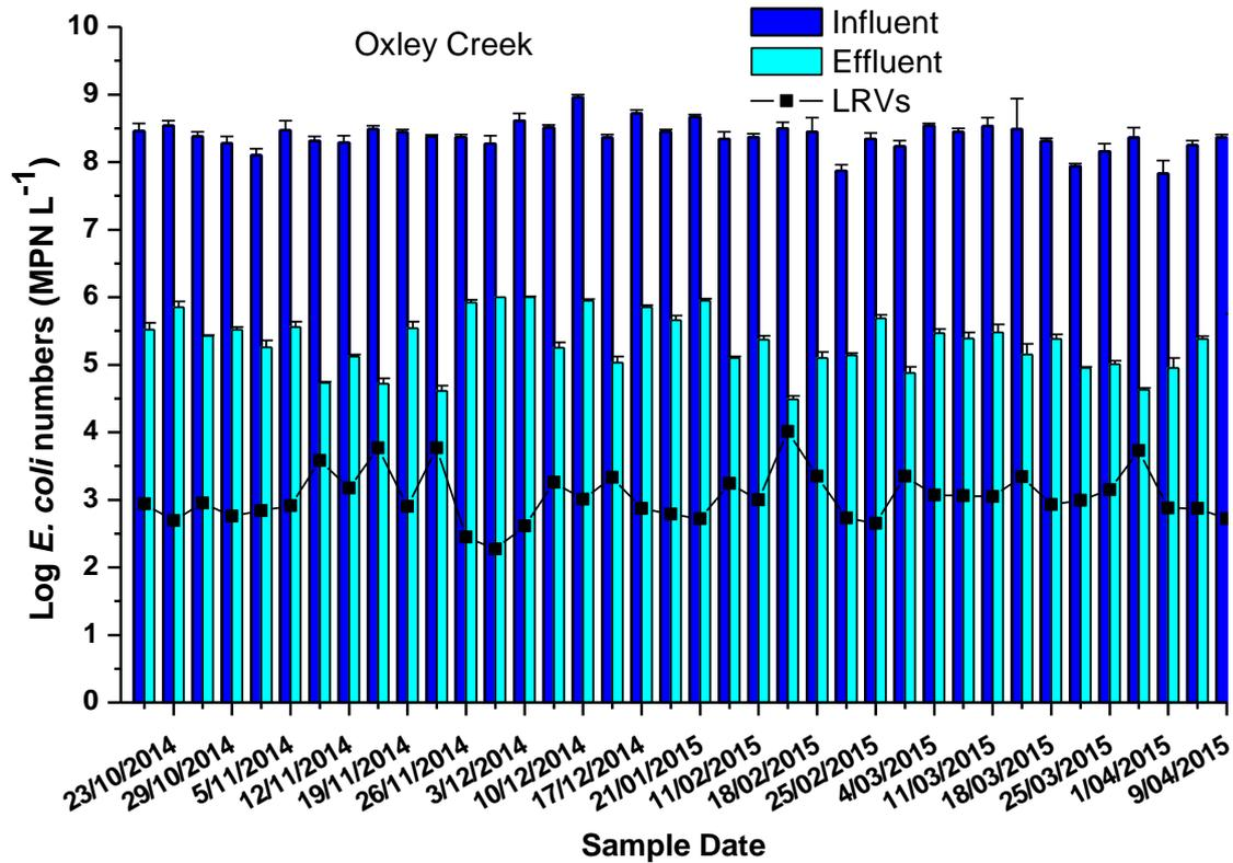
Figure 5-1. Comparative *Escherichia coli* numbers in the influent and effluent samples (n=40) at Oxley Creek wastewater treatment plant.
