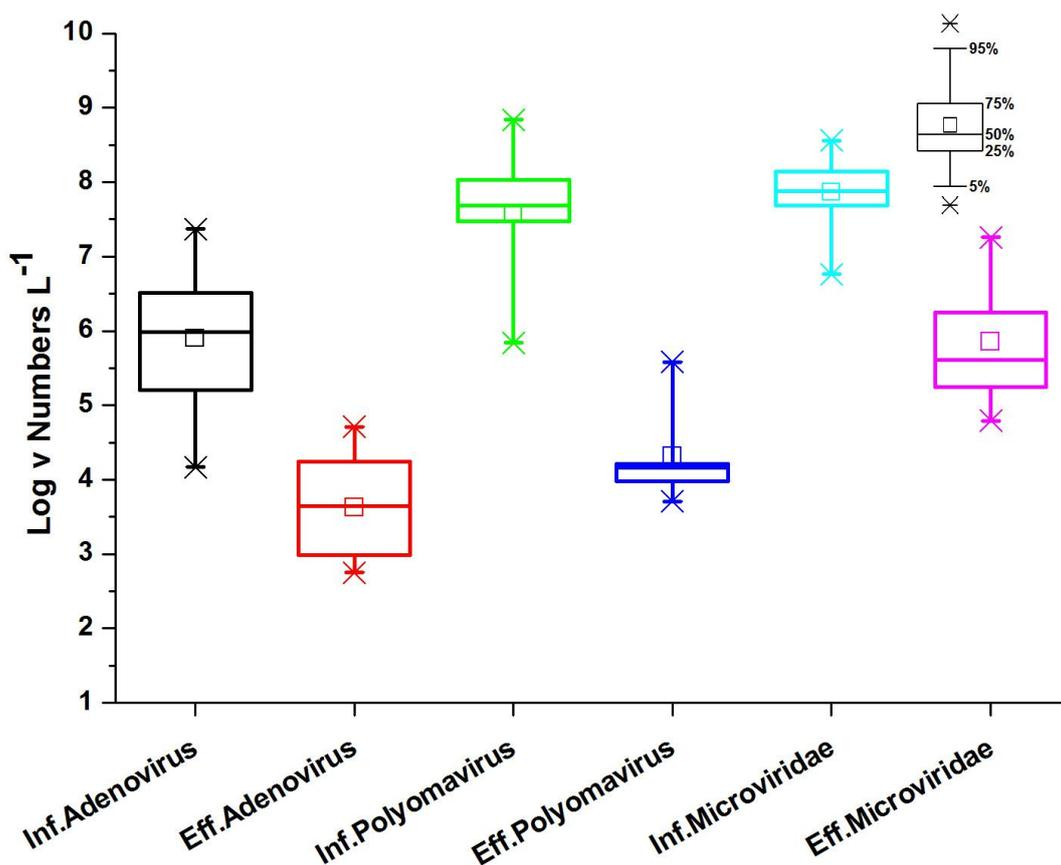
**Figure 6-6. Comparative adenovirus, polyomavirus and *Microviridae* numbers in influent (Inf.) and effluent (Eff.) samples collected from Boneo WWTP.**
