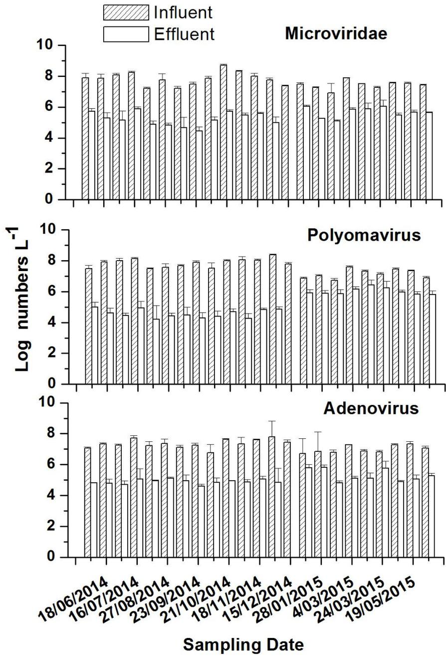
Figure 6-3. Comparative adenovirus, polyomavirus and *Microviridae* numbers in influent and effluent samples collected from the Beenyp WWTp.
