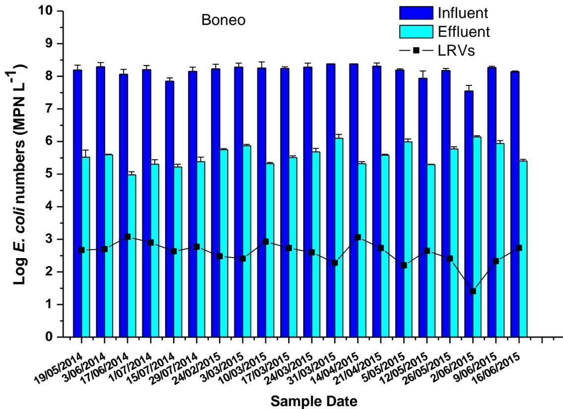
Figure 5-3. Comparative *E. coli* numbers in the influent and effluent samples at Boneo wastewater treatment plant.
