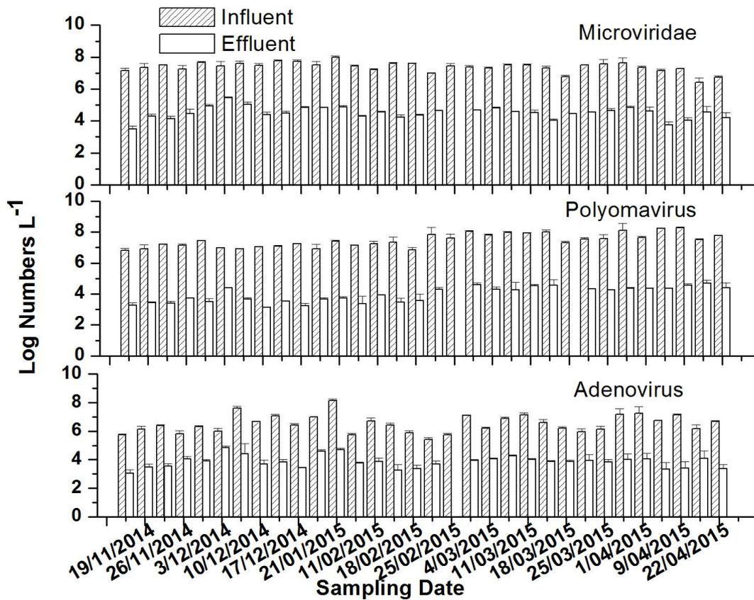
Figure 6-1. Comparative adenovirus, polyomavirus and *Microviridae* numbers in influent and effluent samples collected at the Oxley Creek WWTP.
