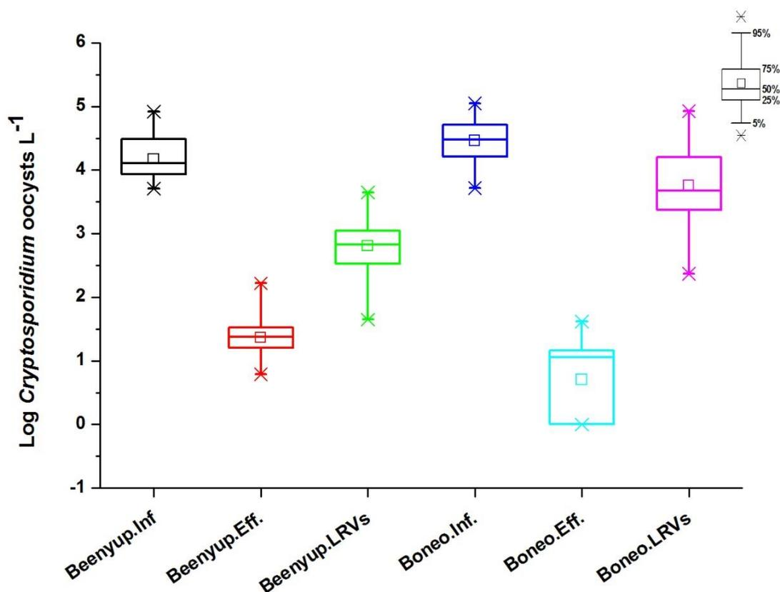
**Figure 7-3. Comparative numbers and log<sub>10</sub> removal of *Cryptosporidium* oocysts in influent and effluent samples at Beenyup and Boneo WWTPs.**
