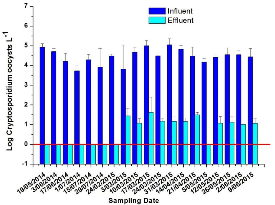
Figure 7-2. Comparative numbers and log<sub>10</sub> removal of *Cryptosporidium* oocysts in influent and effluent samples at Boneo WWTP.
