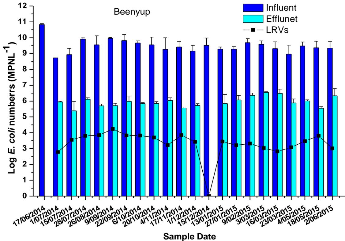
Figure 5-2. Comparative *E. coli* numbers in the influent and effluent samples at Beenyup wastewater treatment plant.
