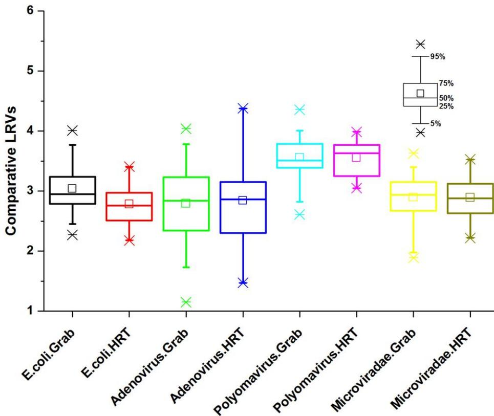
**Figure 9-1. Comparative Log Reduction Values (LRVs) observed from the simultaneous samples (n=40) and paired samples (n=20) on Hydraulic Retention Time (HRT) from Oxley Wastewater Treatment Plant.**
