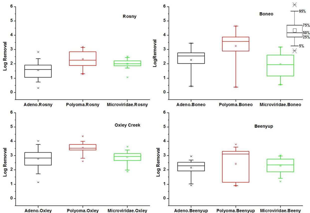
**Figure 8-1. Comparative Log Reduction Values (LRVs) for adenovirus, polyomavirus and *Microviridae* in Box and whisker plot at all four WWTPs.**
