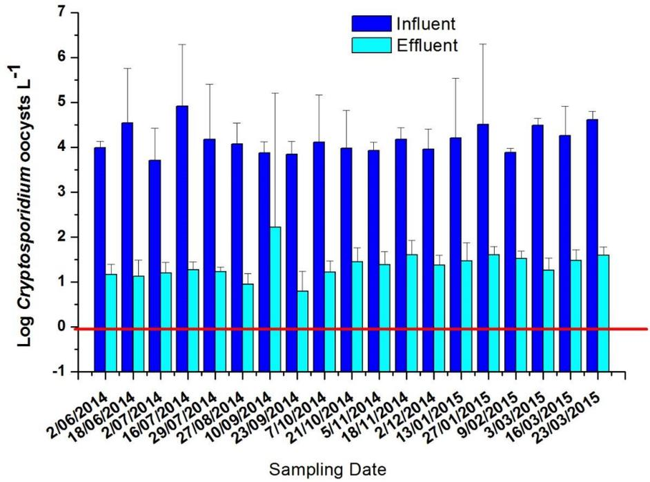
Figure 7-1. Comparative numbers and log<sub>10</sub> removal of *Cryptosporidium* oocysts in influent and effluent samples from Beenyup WWTP.
