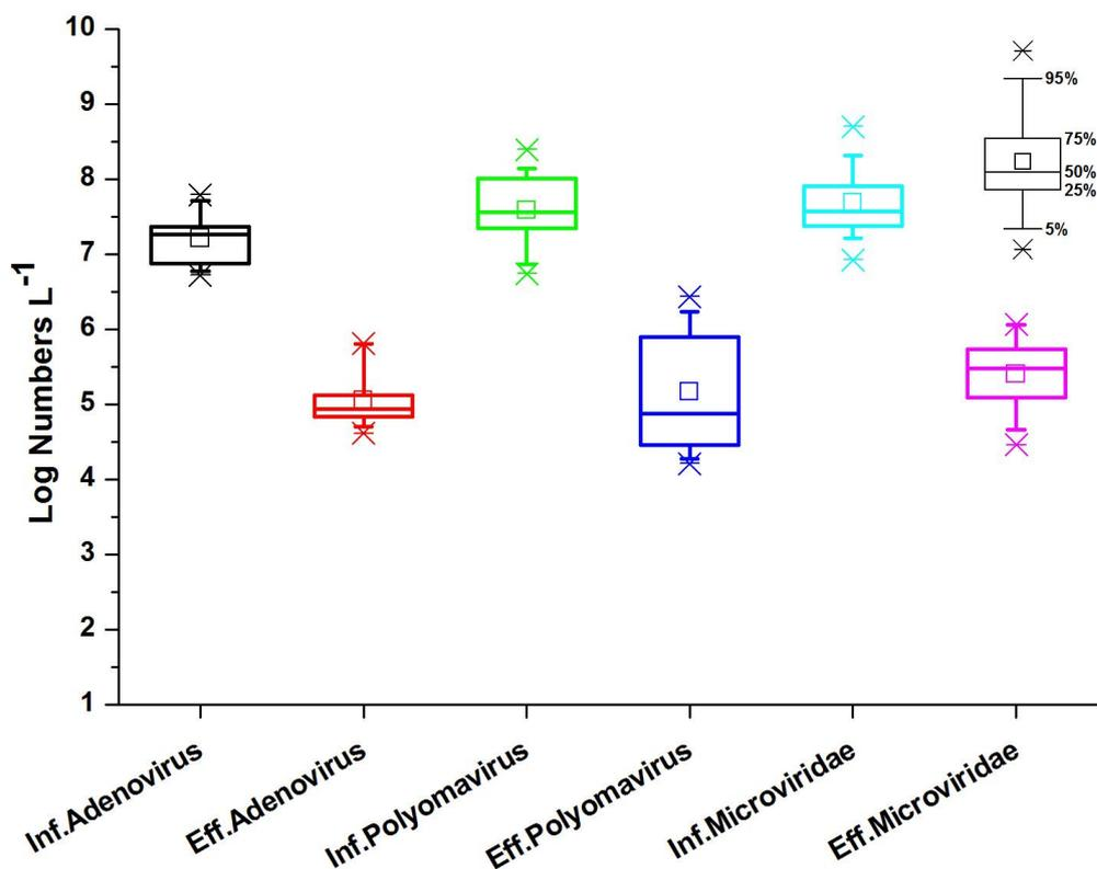
**Figure 6-4. Comparative adenovirus, polyomavirus and *Microviridae* numbers in influent (Inf.) and effluent (Eff.) samples collected from the Beenyup WWTP.**
