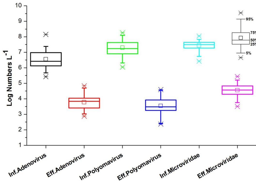
Figure 6-2. Comparative distribution of adenovirus, polyomavirus and *Microviridae* numbers in influent (Inf.) and effluent (Eff.) samples collected at the Oxley Creek WWTP.
