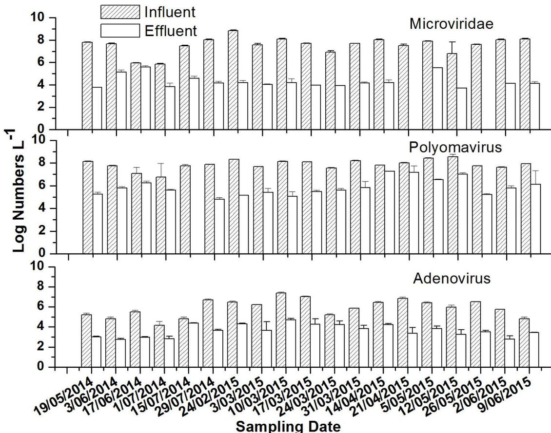
Figure 6-5. Comparative adenovirus, polyomavirus and *Microviridae* numbers in influent and effluent samples collected at the Boneo WWTP.
