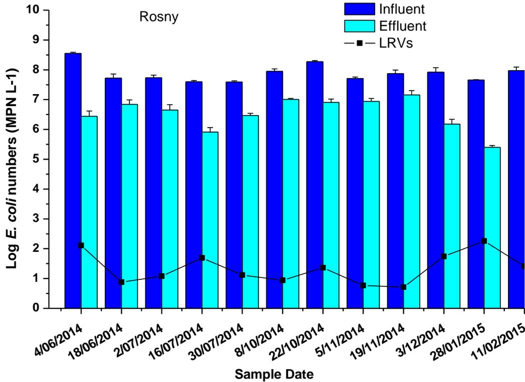
Figure 5-4. Comparative *E. coli* numbers in the influent and effluent samples at Rosny wastewater treatment plant.
