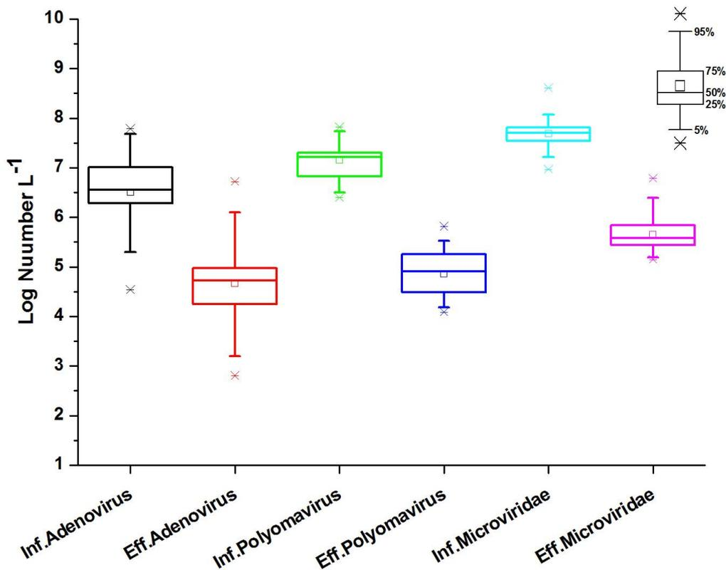
**Figure 6-8. Comparative adenovirus, polyomavirus and Microviridae numbers in influent (Inf.) and effluent (Eff.) samples collected from Rosny WWTP.**
