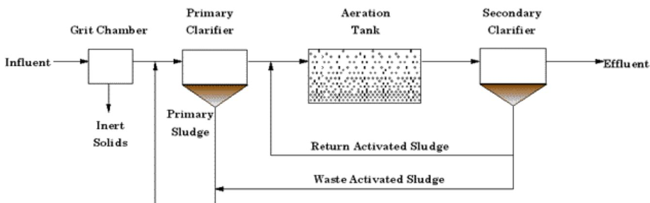
Figure 3-1. Schematic diagram of an activated sludge treatment plant.
