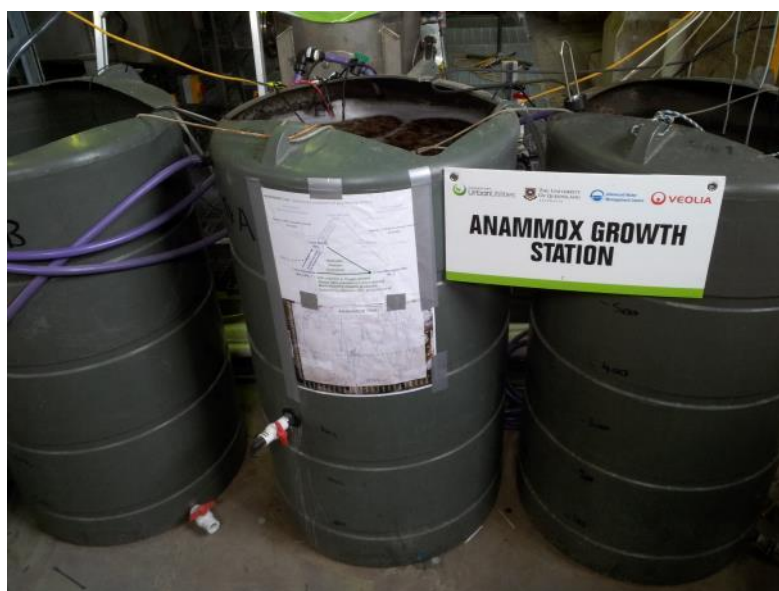
Figure 29. The anammox growth station in the Innovation Centre.
