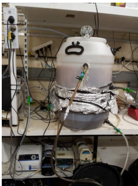
Figure 6. 50 L reactor for enrichment of anammox biomass on carriers.
