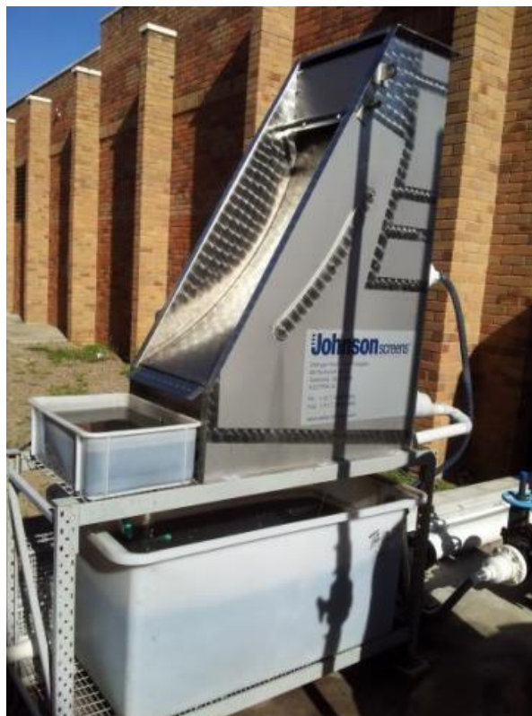
Figure 19. The static sieve bend unit outside the Innovation Centre providing screened sewage for the two treatment trains.
