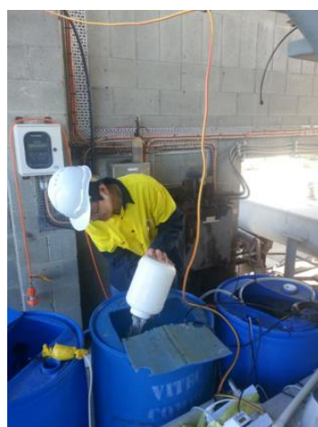
Figure 28. Inoculation of pilot-scale anammox enrichment tanks with biomass enriched in Phase 2 lab-scale study at Luggage Point STP.
