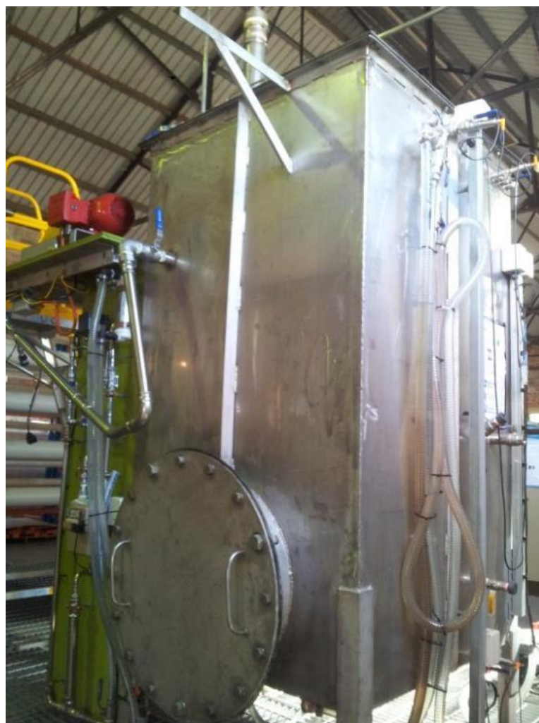
Figure 37. Reciprocatory AnMBR tank set up at the Innovation Centre.
