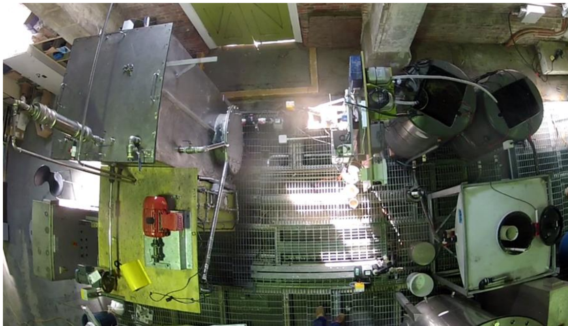
Figure 36. Mainstream AnMBR plus mainstream anammox pilot plant.
