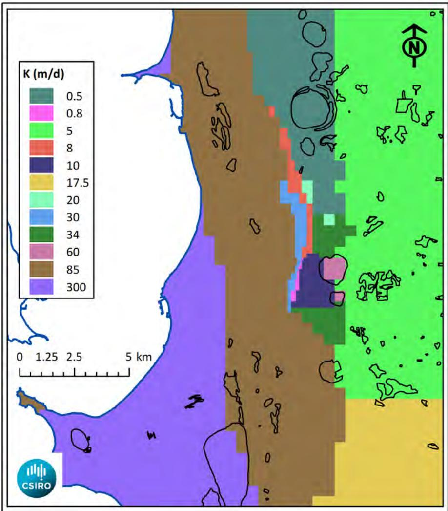
Figure 26 Zones of hydraulic conductivity for Layers 1 and 2
