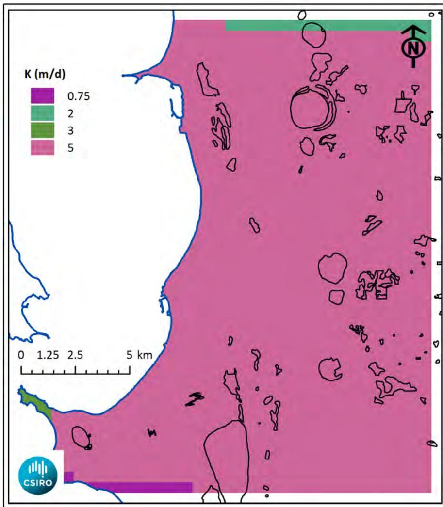
Figure 31 Zones of hydraulic conductivity for Layer 7
