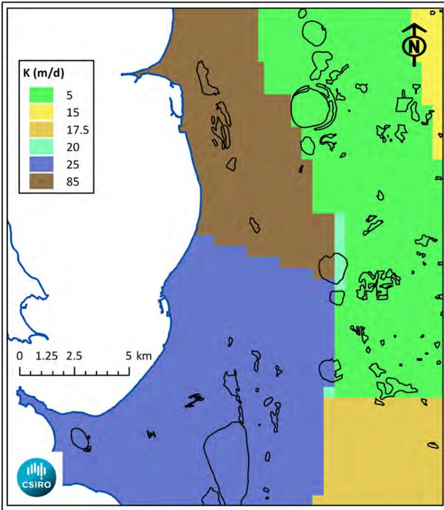
Figure 28 Zones of hydraulic conductivity for Layer 4
