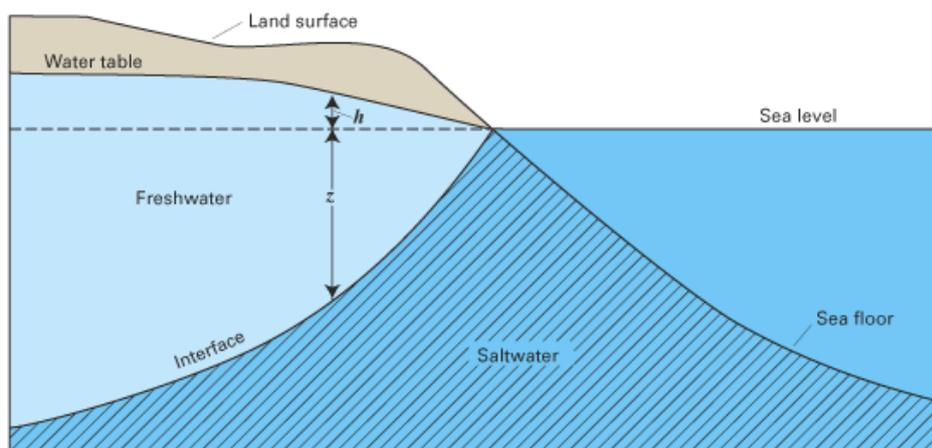
Figure 8.16 The freshwater-saltwater interface along a coastline. Reprinted from “Ground water in freshwater-saltwater environments of the Atlantic Coast,” by P. Barlow (2003), U.S. Geological Survey Circular 1262. Public domain image
