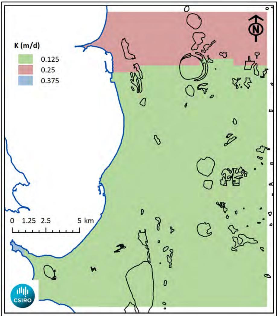
Figure 32 Zones of hydraulic conductivity for Layer 8
