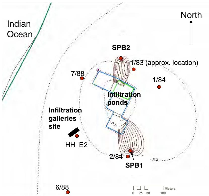
Figure 6.11 Map view of the infiltration galleries site at Halls Head relative to the ponds, monitoring bores and capture zones for recovery bores SPB1 and SPB2. Adapted from “Halls Head indirect treated wastewater reuse scheme,” by Toze et al. (2002), Client report to the Water Corporation. Copyright 2002. Adapted with permission.
