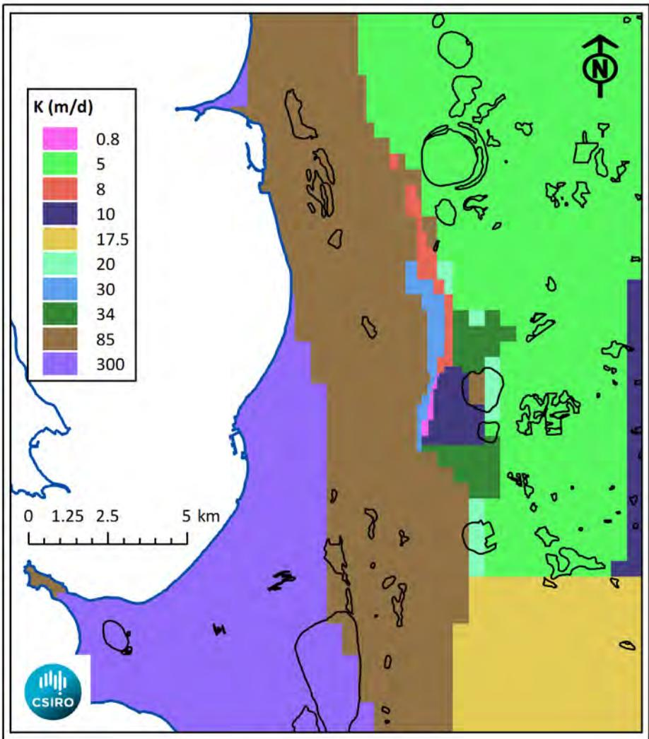
Figure 27 Zones of hydraulic conductivity for Layer 3
