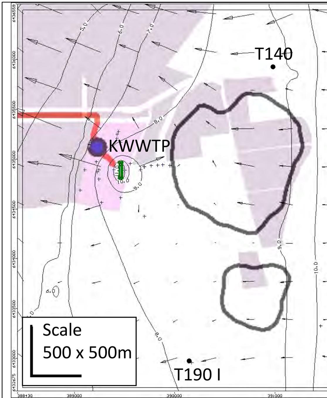
**Figure 8.12 Location of monitoring wells T140 and T190 I relative to the Kwinana WWTP and model predicted hydraulic heads for April 2004 to compare with data and model in Nield (2004)**
