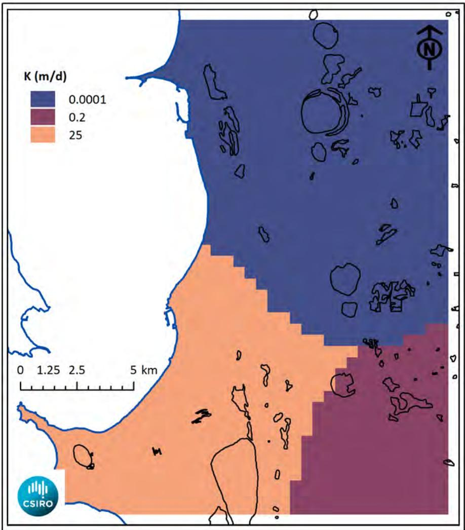
Figure 29 Zones of hydraulic conductivity for Layer 5
