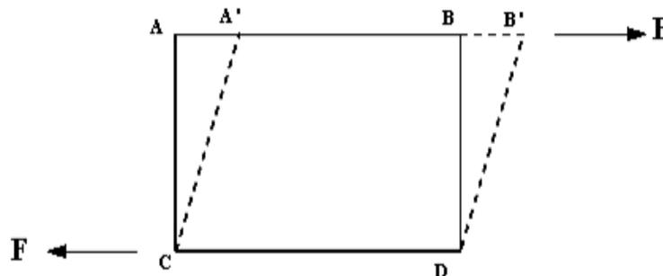
**Fig. 2A.6** Shearing force,  $F$  acting tangentially on a rectangular (solid lined) element  $ABDC$  and produces the (dashed lined) rhombus element  $A'B'DC$ .
