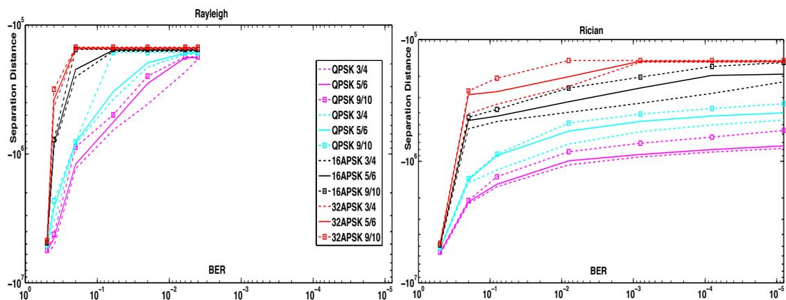
Figure 6.6: Separation distance vs. BER graph for Rayleigh and Rician
