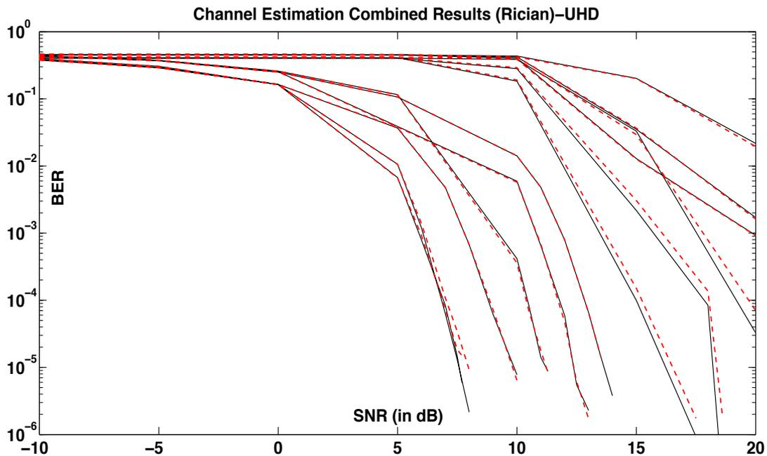
Figure 5.37: Channel Estimation results: UHD (black) vs. HD (red)
