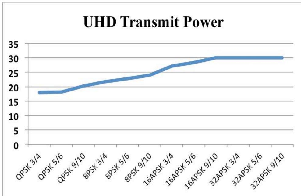
Figure 6.9: UHD Transmit Power in dBm
