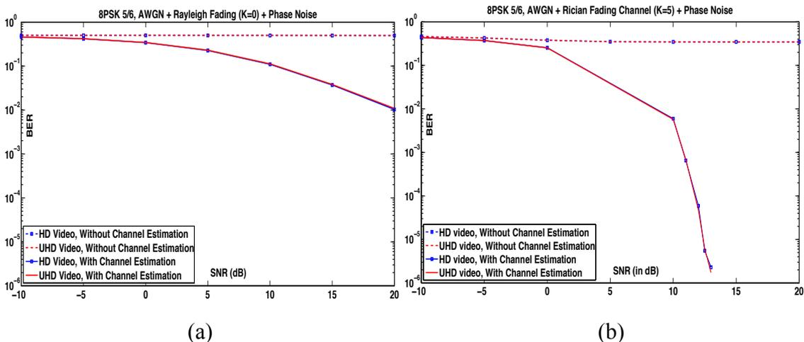
Figure 5.28: BER vs. SNR for 8PSK-5/6 (a) Rayleigh Fading (b) Rician Fading
