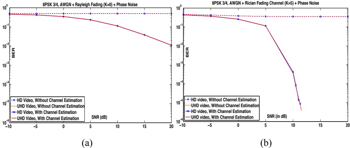
Figure 5.27: BER vs. SNR for 8PSK-3/4 (a) Rayleigh Fading (b) Rician Fading
