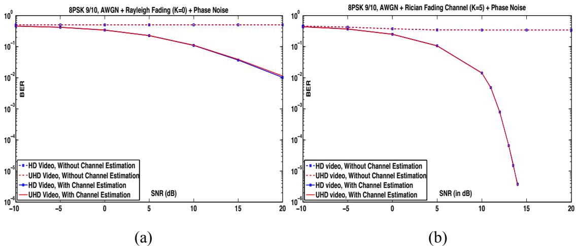
Figure 5.29: BER vs. SNR for 8PSK-9/10 (a) Rayleigh Fading (b) Rician Fading
