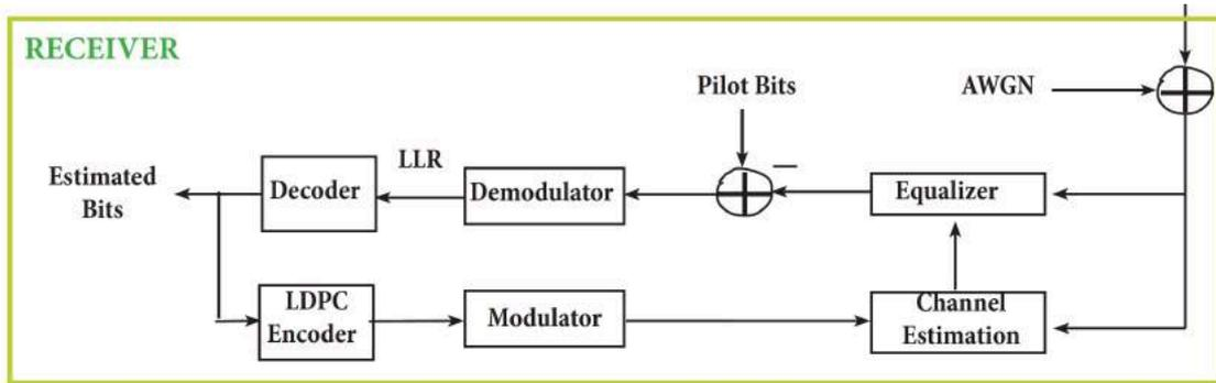
Figure 4.1 Channel Estimation Block Schematic
