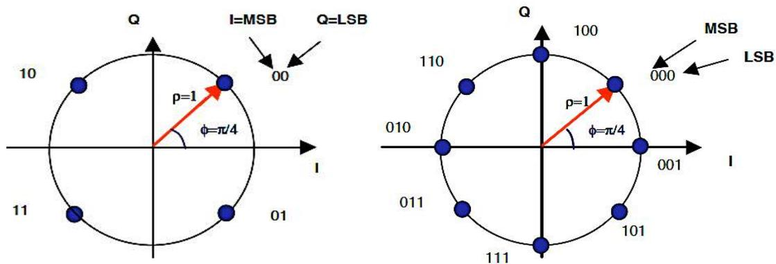
Figure 3.3: Constellation Diagram of QPSK (left) and 8PSK (right) [25]
