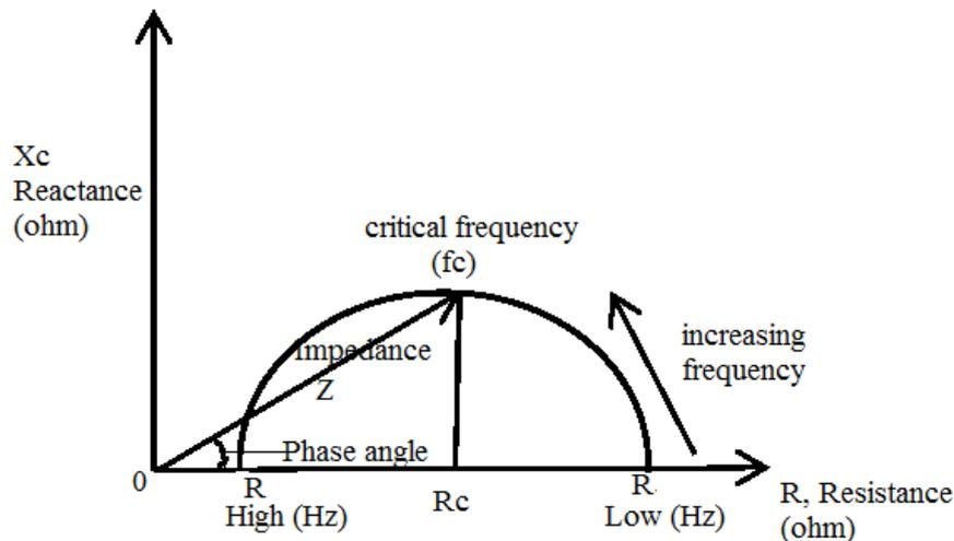
FIGURE 2.4: Reactance versus resistance as a function of frequency adapted from Jaffrin *et al* [65]
