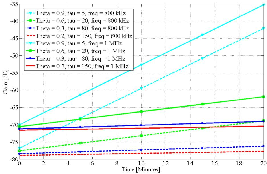
FIGURE 4.8: Model predictions of attenuation for simulated hydration at 800 kHz and 1 MHz when  $\tau$  is inversely proportional to  $\theta$ . This indicates low BMI equals lower time-dependent metabolic rate [105], higher rate of hydration [24] and more body of water [106]
