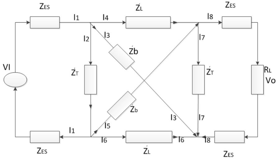
FIGURE A.1: The equivalent circuit showing directions of the current flow
