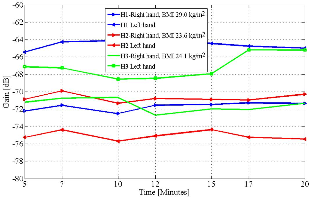
FIGURE 6.7: Graph of galvanic coupled signal attenuation at 900 kHz, after fluid restriction and fluid intake, on both arms of healthy subjects
