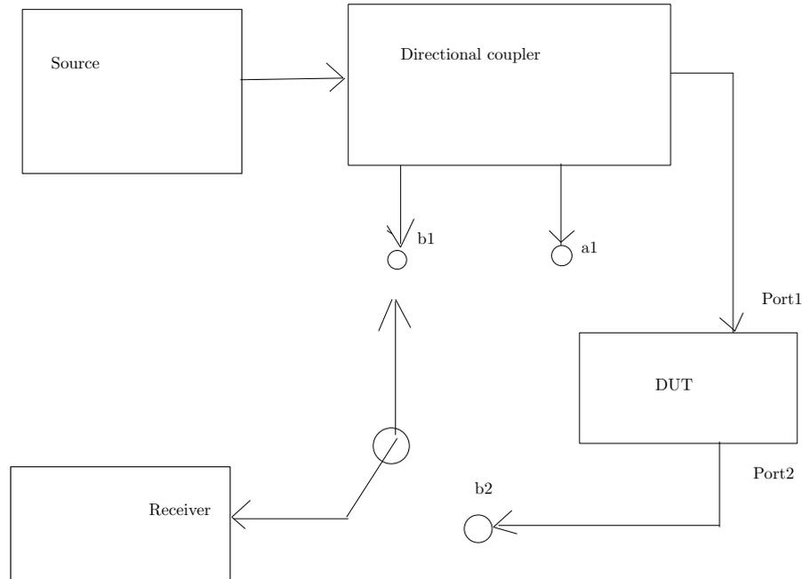
FIGURE 3.2: Schematic diagram for measuring the scattering parameters of the using a two port network model
