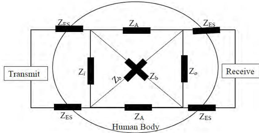
FIGURE 2.12: Simplified four terminal galvanically coupled IBC circuit showing approximations of the impedance components by Song *et al* [69]
