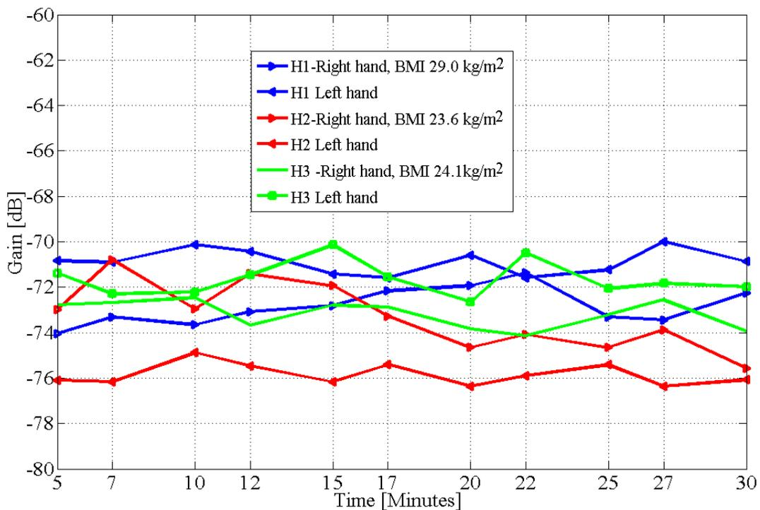
FIGURE 6.6: Graph of galvanic coupled signal attenuation at 900 kHz, on both arms of healthy subjects without fluid restriction
