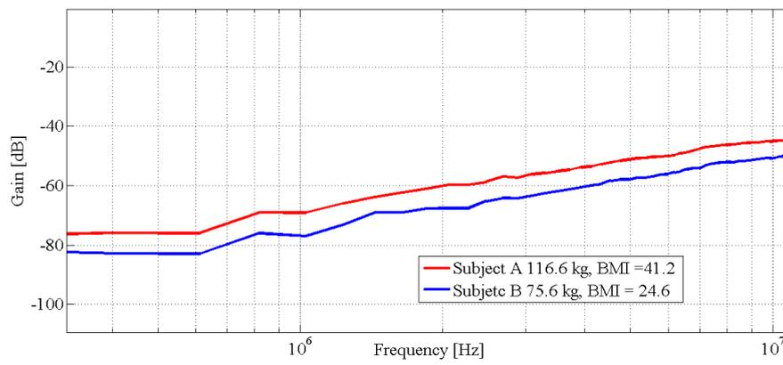
FIGURE 3.9: Gain versus frequency for high and low BMI at 20 cm distance between transmit and receive electrodes
