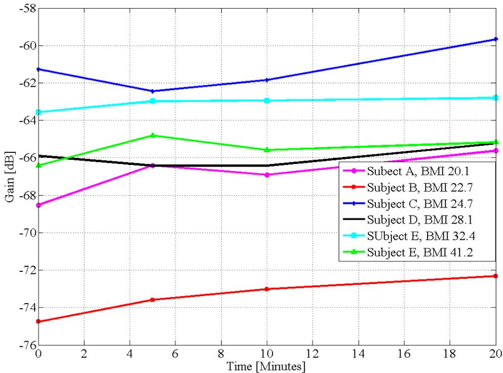
FIGURE 4.12: Changes in signal gain at 1 MHz as hydration occurs on 6 subjects after fluid intake
