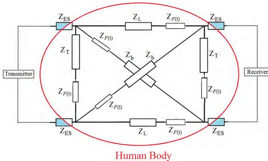
FIGURE 4.1: Improved circuit with variable impedance component from dynamic changes in human body fluid level
