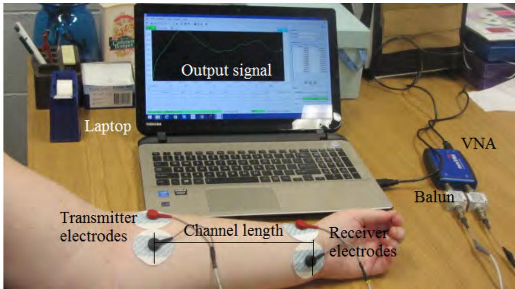
FIGURE 6.1: Measurement of galvanic coupled signal attenuation on the affected left arm of a lymphoedema subject
