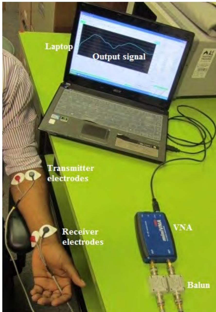
FIGURE 3.13: Galvanic-coupling circuit on the lower left arm, the four terminal silver-silver chloride Noraxon electrodes are attached to the body and connected to the VNA via a balun. The output signal shows on the laptop screen fitted with the VNA software
