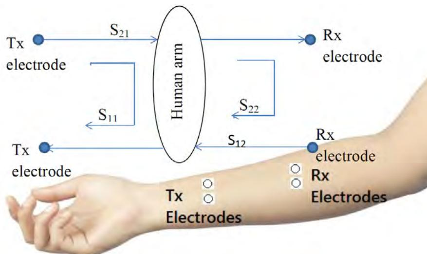
FIGURE 3.3: Human body arm showing the measurement of scattering parameters in a galvanic coupled signal transmitted from Tx and received at Rx
