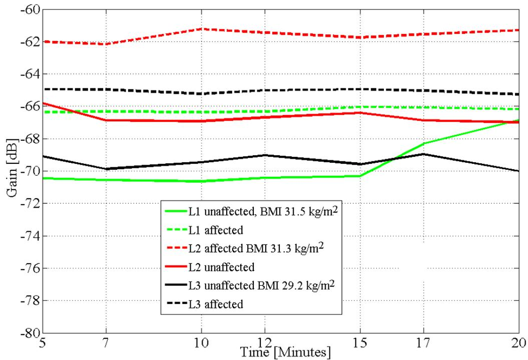
FIGURE 6.5: Graph of galvanic coupled signal attenuation at 900 kHz, after fluid restriction and intake of water, on both arms of lymphoedema affected subjects
