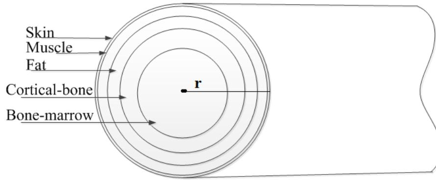
FIGURE 4.2: A cross section of the arm with radius  $r$ , showing the different tissue layers used in this experiment
