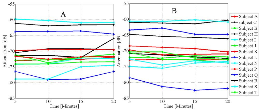
FIGURE 5.4: Graph of the rate of hydration A, and dehydration B, after 600 mL of fluid intake on subjects A,C,E,H,I,J,K,L,N,P,Q,R,S and T observed at 900 kHz.  $W_2 < W_0$ . The protocol produced mild dehydration on subjects
