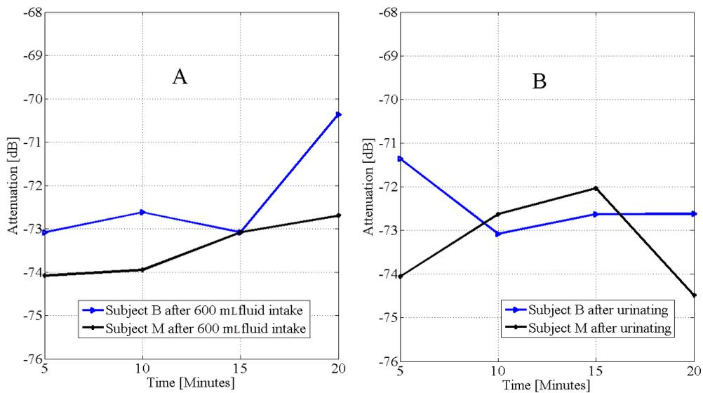
FIGURE 5.3: Graph of the rate of hydration A, and dehydration B, after 600 mL of fluid intake on subjects B and M observed at 900 kHz,  $W_2 < W_0$ . The protocol produced severe dehydration on subjects B and M. After urinating, subject B dehydrated and stopped after 10 minutes while subject M started dehydration after 15 minutes. Both showed longer period of re-absorption
