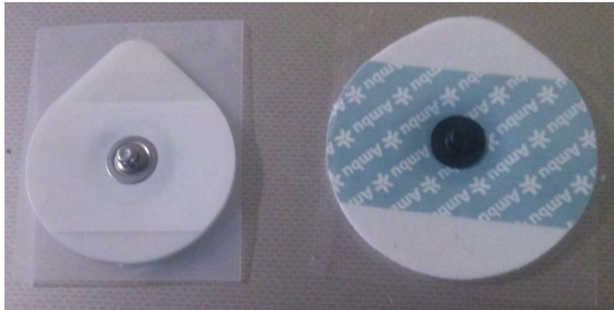
FIGURE 3.6: Round pre-gelled medical electrodes. Left is Noraxon self-adhesive, single use, EMG electrode, product code: 270 and Right is Ambu WhiteSensor single use self-adhesive ECG electrode, product code: 4500M
