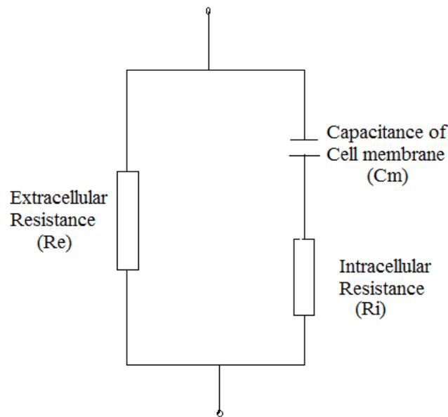
FIGURE 2.3: Equivalent circuit of tissues with parallel resistances
