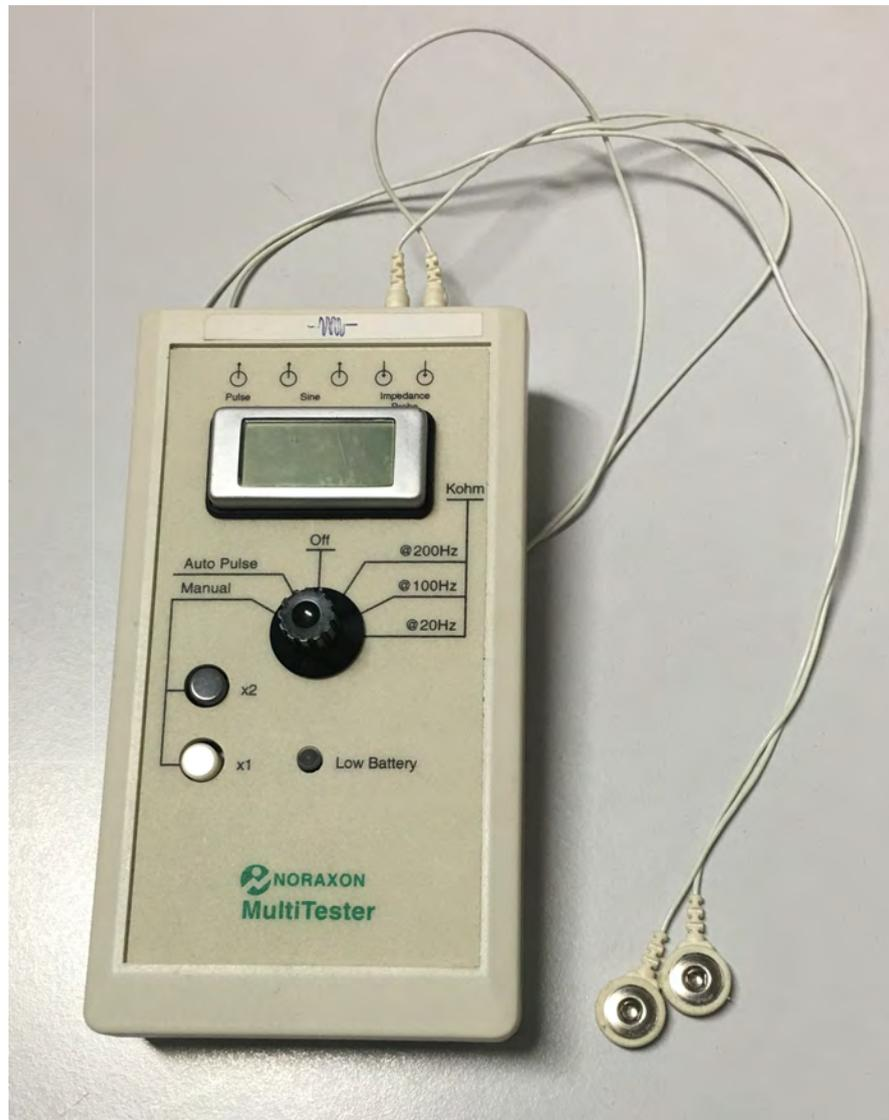
FIGURE 3.12: Noraxon Multitester for testing skin-electrode impedance
