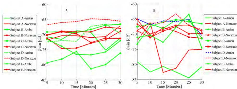
FIGURE 3.10: Transmission coefficient "A" without body movement and "B" with body movement
