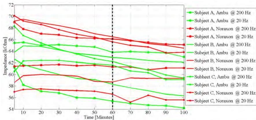
FIGURE 3.7: Comparison of skin-electrode impedance of Noraxon EMG electrode and Ambu WhiteSensor 4500M, ECG electrode on 3 subjects at 200 Hz and 20 Hz.
