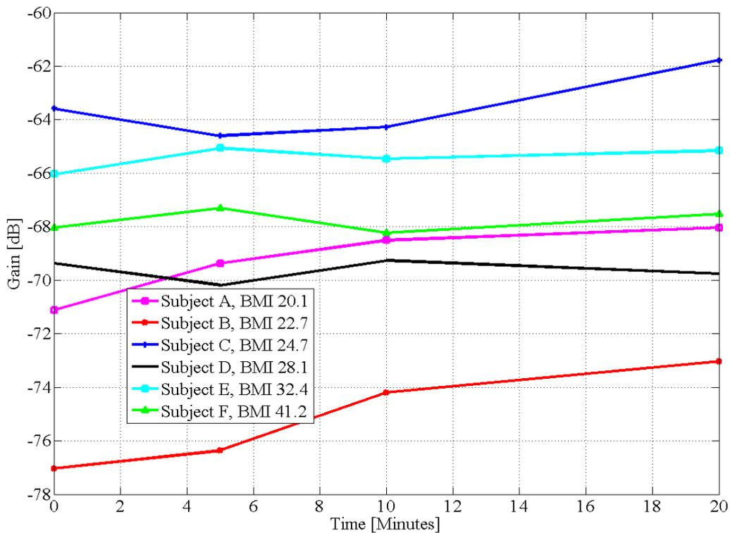
FIGURE 4.11: Changes in signal gain at 800 kHz as hydration occurs on 6 subjects after fluid intake
