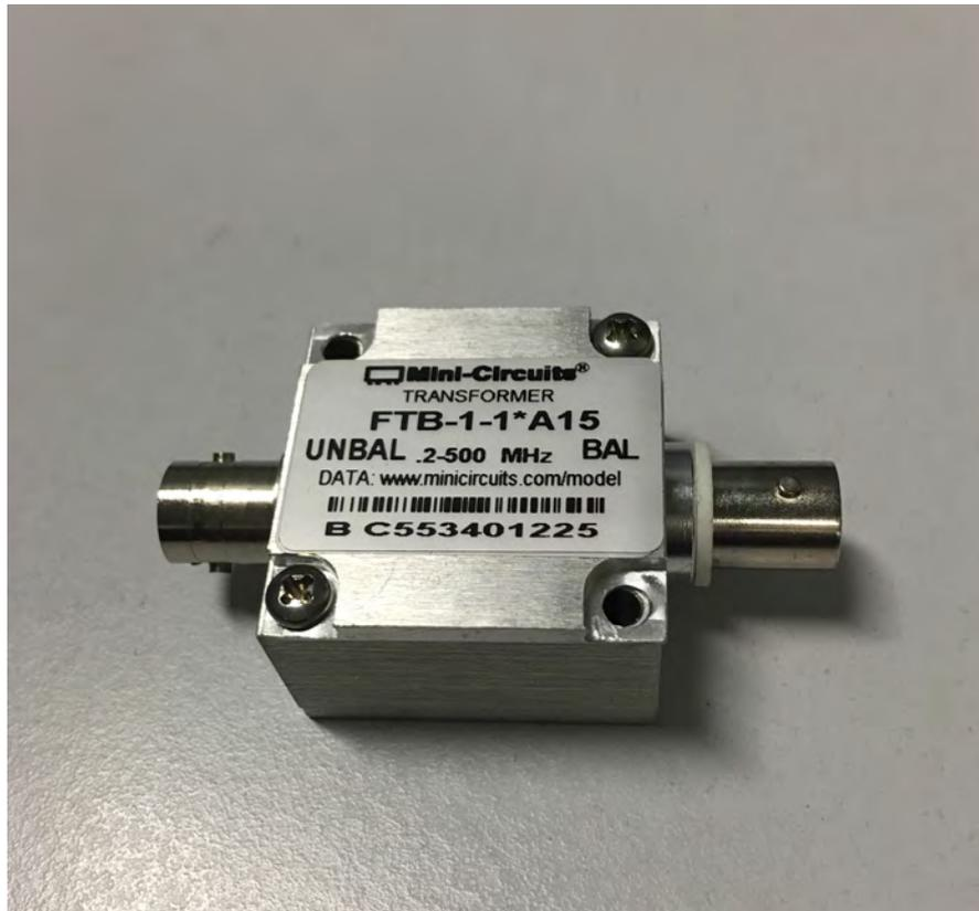
FIGURE 3.4: Balun model number FTB-1-1+ impedance ratio 1, and frequency range 0.2-500 MHz
