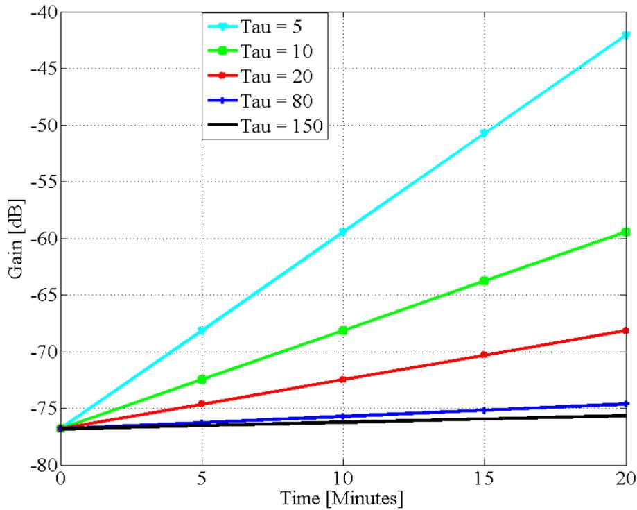
FIGURE 4.7: Graph of attenuation versus time at 800 kHz, showing the effect of changes in  $\tau$ , at  $\theta = 0.9$ .
