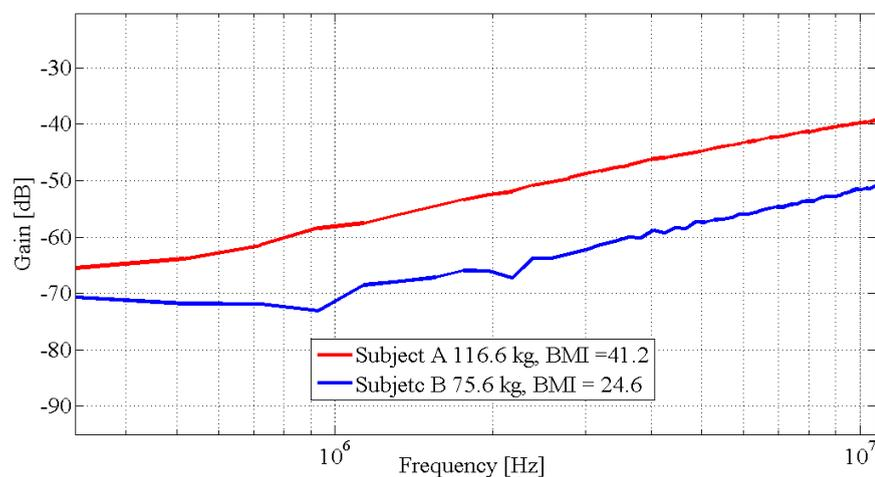
FIGURE 3.8: Gain versus frequency for high and low BMI at 10 cm distance between transmit and receive electrodes
