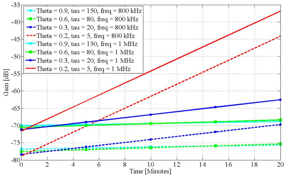
FIGURE 4.9: Model predictions of attenuation for simulated hydration at 800 kHz and 1 MHz where  $\tau$  is proportional to  $\theta$ . The result shows high BMI has high hydration rate and low time-dependent metabolic rate. This is not supported by empirical results and is not explained physiologically
