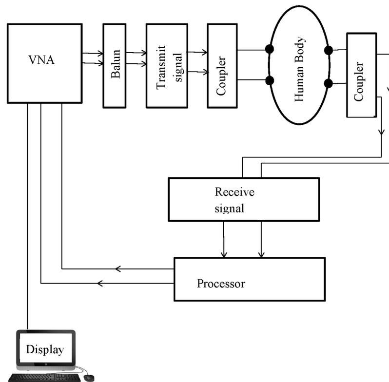
FIGURE 3.1: Block diagram of the devices used for measurement
