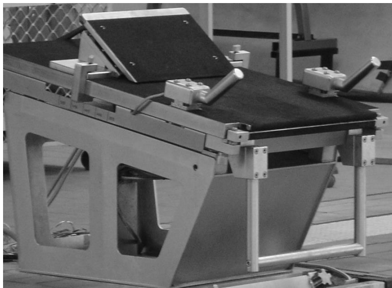
Figure 6 Wetplate Analysis System - Instrumented Starting Block
