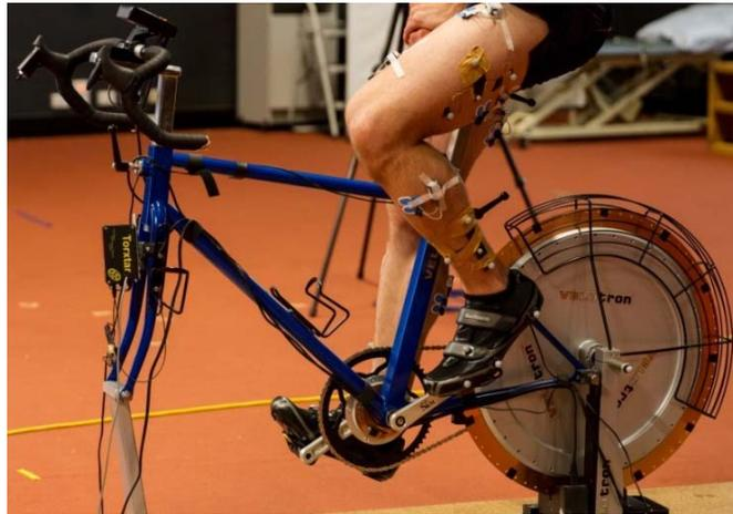
**Figure 4.4.** Experimental set up for data collection, including the equipment used for mechanical, kinematic and EMG data acquisition.
