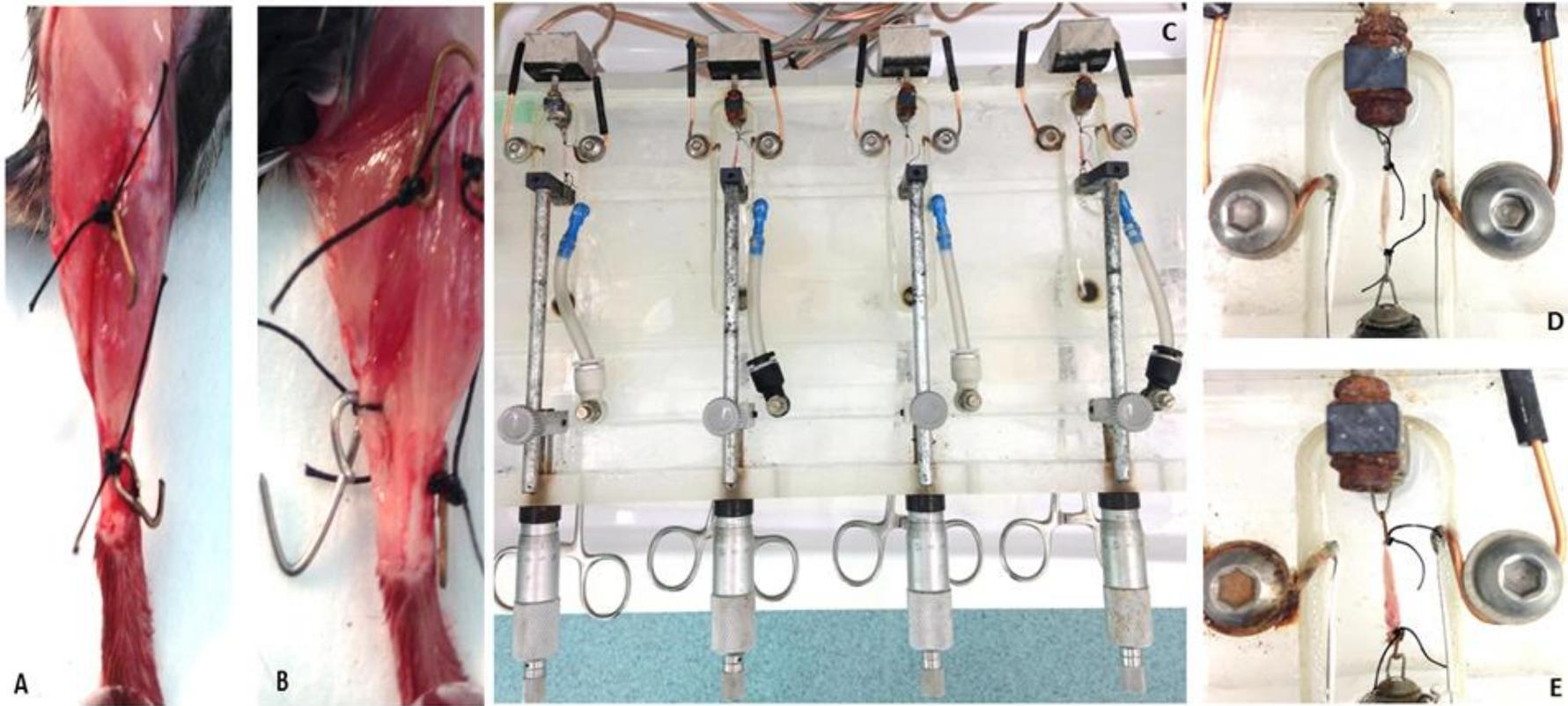
**Figure 3.2. Muscle dissection and contractile bath setup.** Panels A and B demonstrate the tied proximal and distal tendons of EDL and SOL respectively. Panel C shows the contractile baths housing the EDL (bath 1 and 3) and SOL (bath 2 and 4) during equilibration time with Panels D and E showing close-ups of EDL and SOL, respectively.
