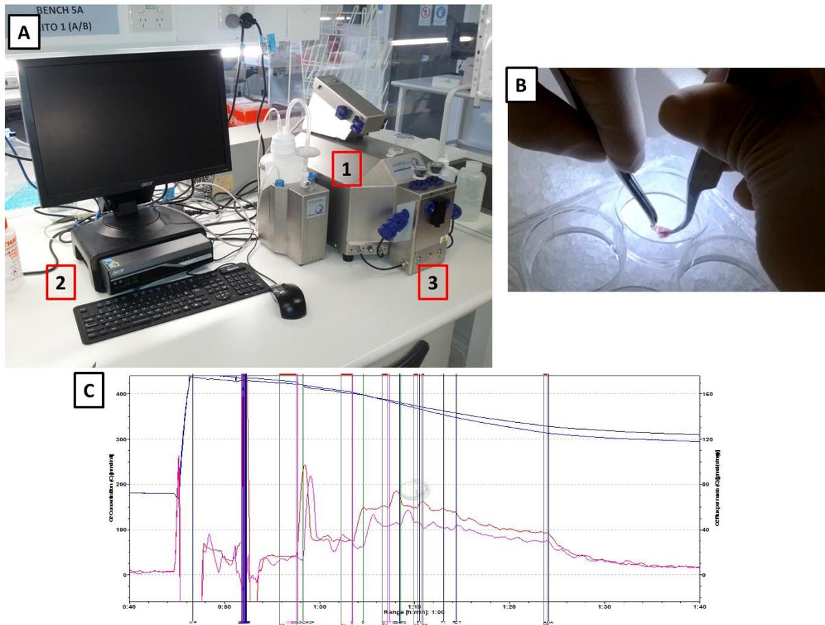
**Figure 2-3. Mitochondrial respiration apparatus, muscle fibre separation and respiration data.** A, Oxygraph-2k (1), computer system with DataLab software v5.1.0.2 (2), and O2k-Fluo LED2-Module (3). B, mechanical separation of muscle fibres, in preparation for permeabilisation procedure. C, Representative data obtained from DataLab software.
