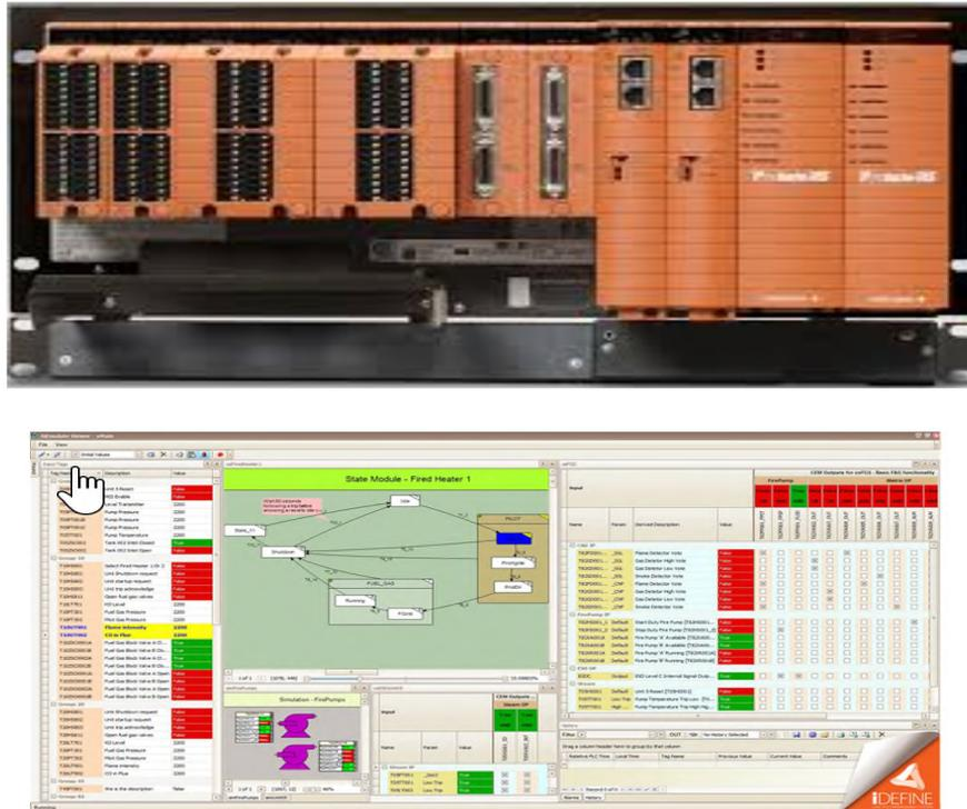
**Fig. 5.13.** Logic Solver Yokogawa ProSafe-RS and Workbench
