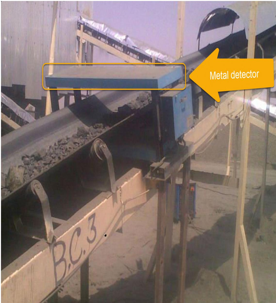
**Fig. 3.7.** SIF#2 (M100) – Metal Detector [118]
