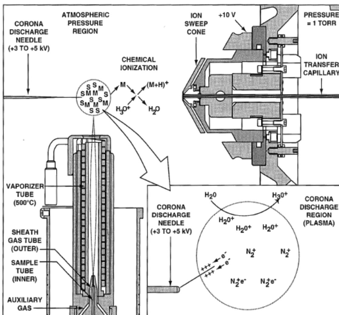
Figure 1-7: Atmospheric pressure chemical ionisation process in the positive ion polarity mode (Thermo Electron Corporation 2003)
