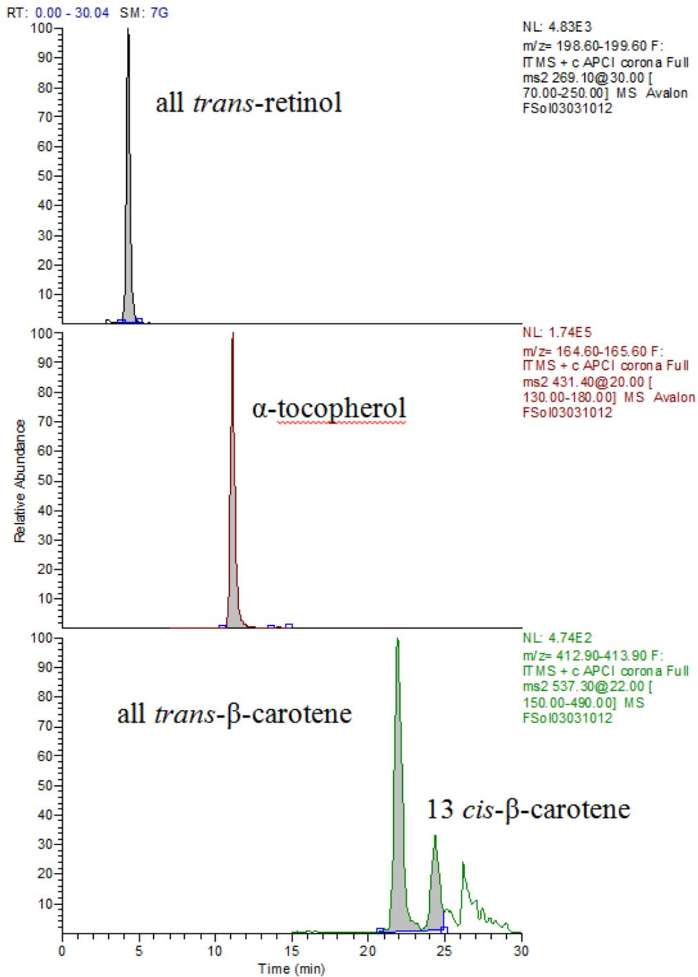
Figure 4-1: HPLC-MS<sup>2</sup> chromatogram of a cow milk sample containing all *trans*-retinol (50  $\mu\text{g}/100\text{ ml}$ ),  $\alpha$ -tocopherol (200  $\mu\text{g}/100\text{ ml}$ ) and  $\beta$ -carotene (12  $\mu\text{g}/100\text{ ml}$ )
