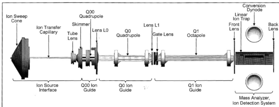
Figure 1-8: Internal components of the linear ion trap mass spectrometer (Thermo Electron Corporation 2003)
