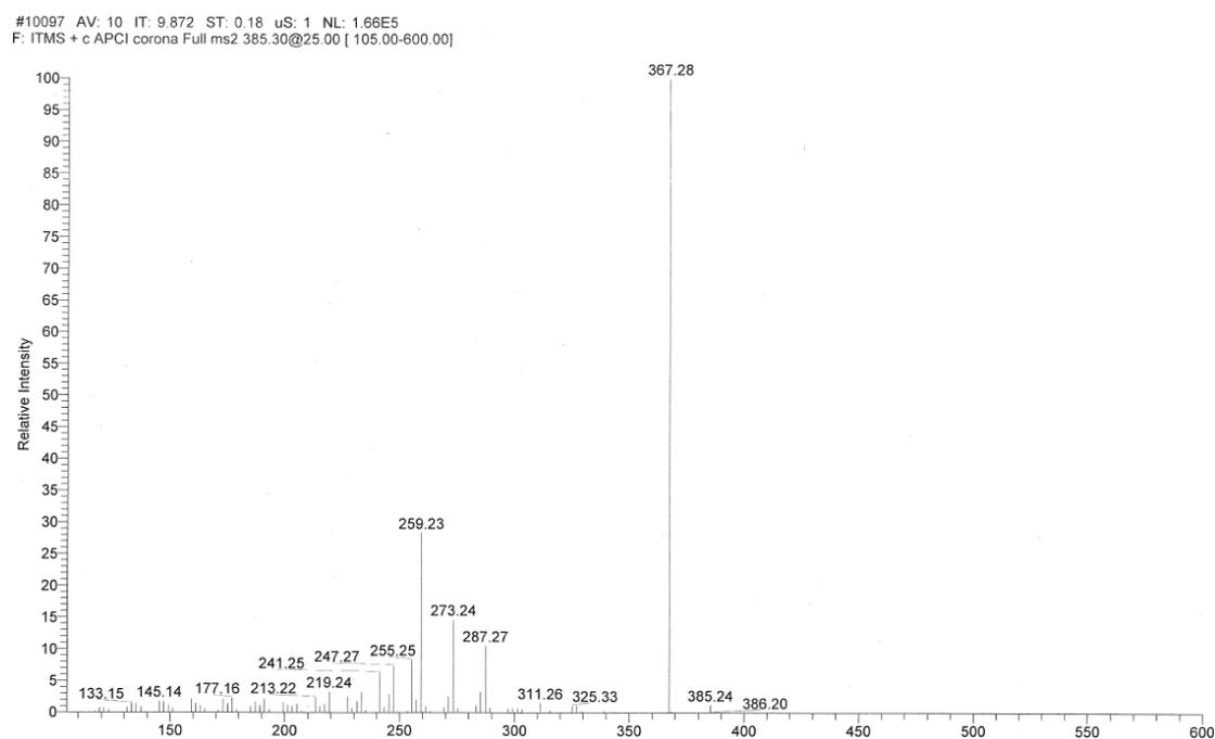
Figure 3-2: HPLC-MS<sup>n</sup> product ion spectra for the fragmentation of vitamin D<sub>3</sub>
