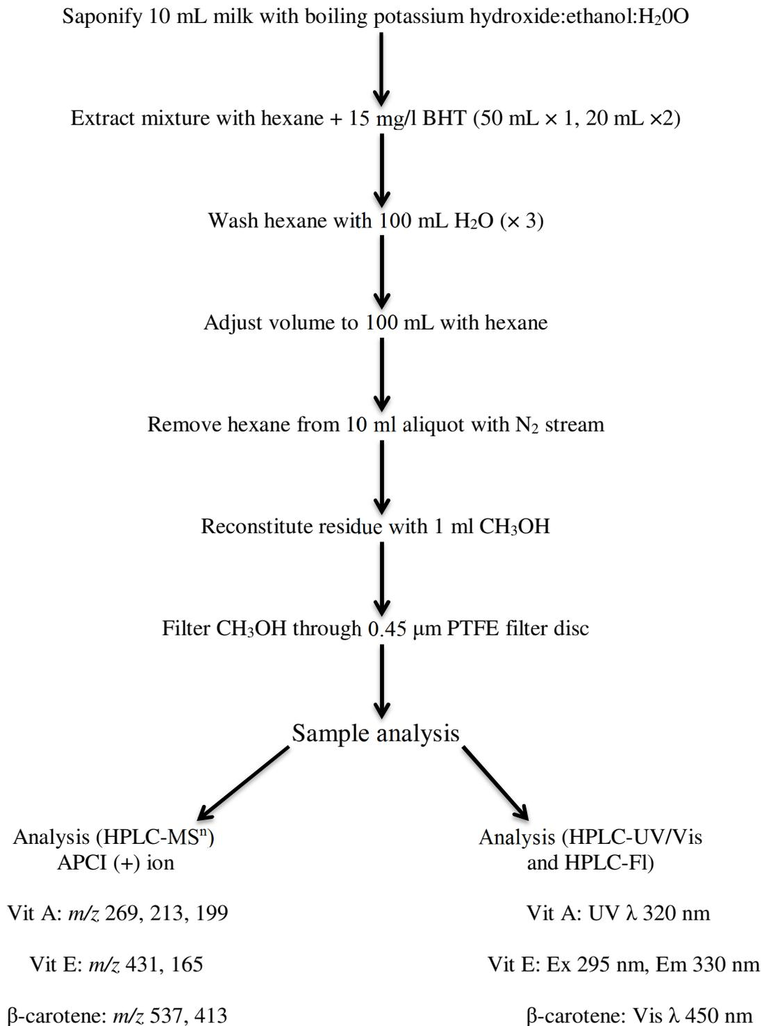
Figure 2-2: Flow diagram of the methodology for the analysis vitamins A, E and β-carotene in cow milk by both HPLC-MS<sup>n</sup> and HPLC-UV/Vis and HPLC-FI
