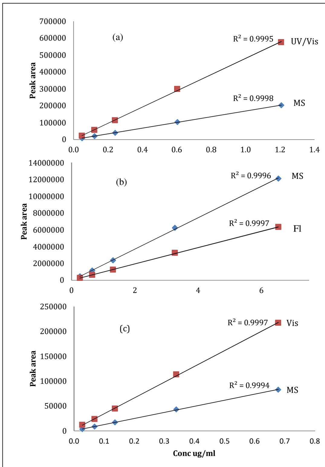
Figure 4-3. HPLC-MS<sup>2</sup>, HPLC-UV/Vis and HPLC-Fl calibration plots for (a) all *trans*-retinol, (b)  $\alpha$ -tocopherol and (c)  $\beta$ -carotene
