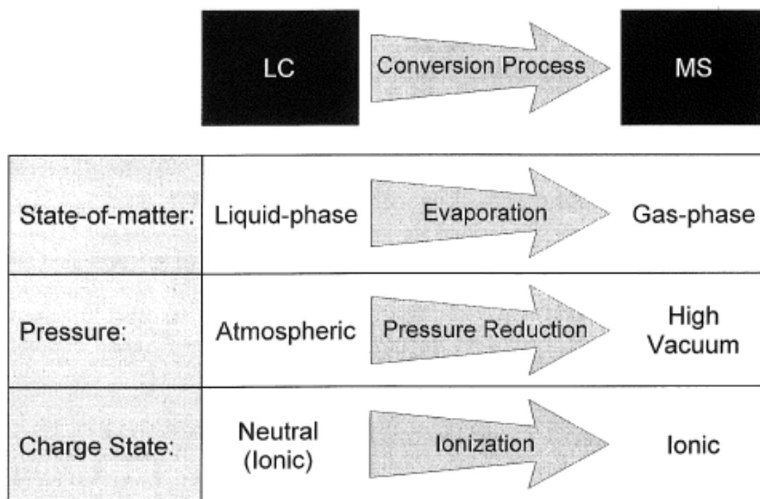
Figure 1-5: Conversion processes required for interfacing liquid chromatography with mass spectrometry (Willoughby 2002)
