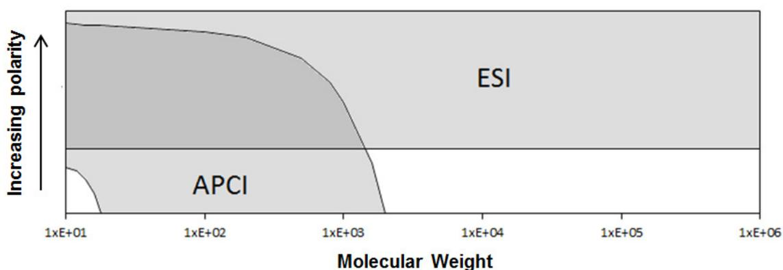
Figure 1-6: The molecular weight and polarity domains of electrospray ionisation and atmospheric pressure chemical ionisation. Adapted from Willoughby 2002.
