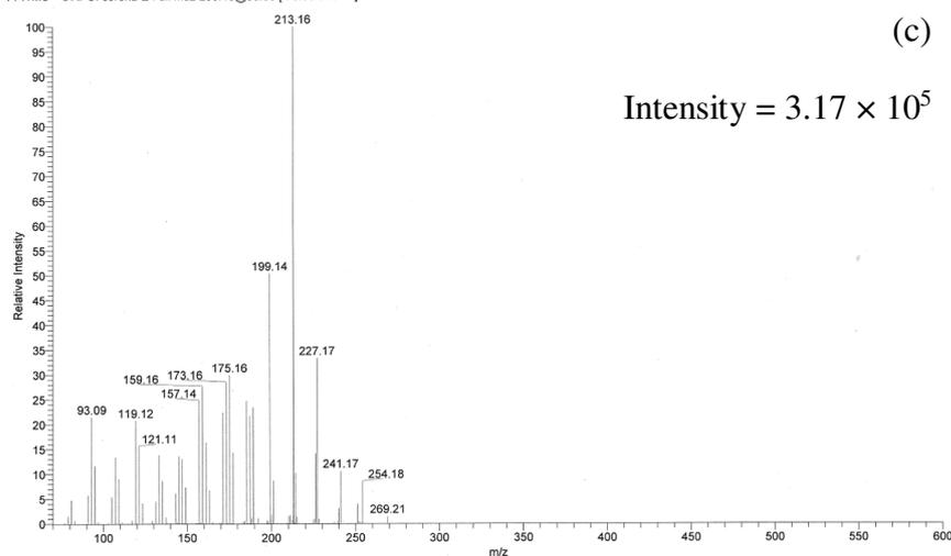
Figure 4-2: Mass spectra of all *trans*-retinol infused into the ion trap MS operating in APCI positive mode, (a) MS<sup>1</sup>, (b) MS<sup>2</sup> with isolation width of 1.0, (c) MS<sup>2</sup> with isolation width of 1.4
