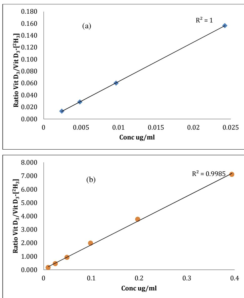
Figure 3-4: HPLC-MS<sup>n</sup> calibration plots for vitamin D<sub>3</sub> for (a) non-fortified samples and (b) fortified samples
