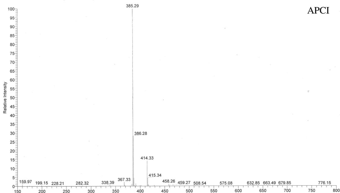
Figure 3-1: Optimised HPLC-MS<sup>n</sup> ESI and APCI spectra of 10 µg/ml vitamin D<sub>3</sub> infused at 10 µl/min into 0.2 ml/min mobile phase
