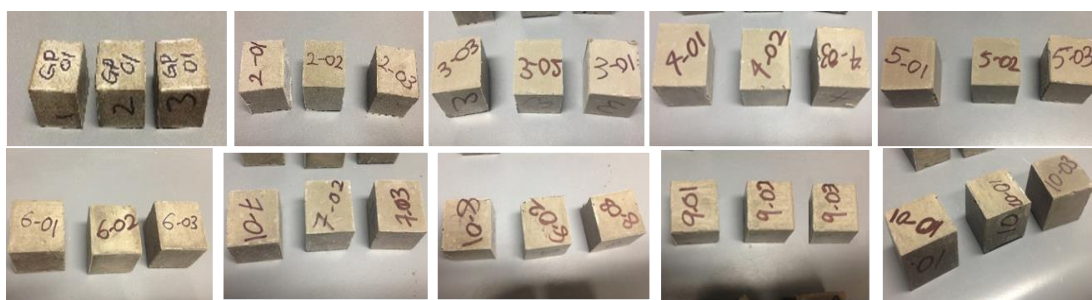
Figure 4.13 – Sealed Gladstone FA GP 25mm specimens–Before temperature exposure
