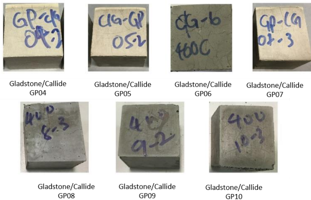
Figure 4.26 – Gladstone/Callide FA GP 50mm specimens after 400°C exposure
