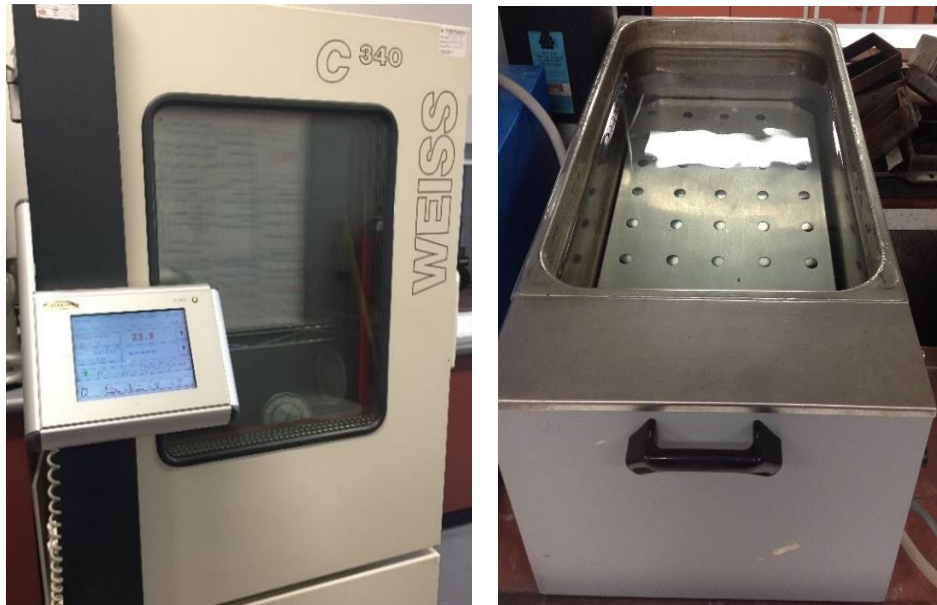
Figure 3.8a (left)–WEISS WVC Series Temperature and Climatic Test Chamber.
