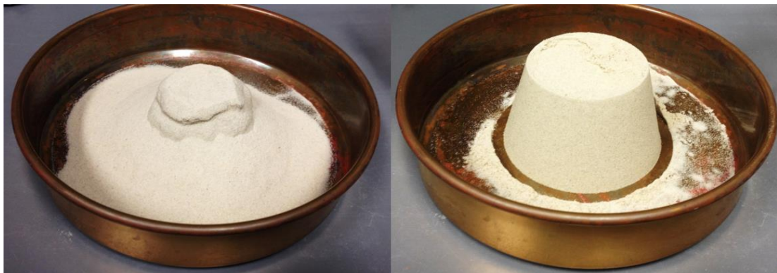
Figure 3.5 – Determination of absorption water required to achieve SSD condition of silica sand
