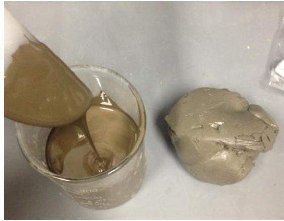
Figure 4.5 – Comparison of workability conditions Gladstone FA GP01 (left)/ Gladstone/Callide FA GP01 (right)
