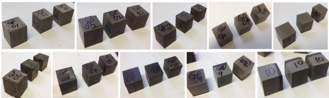
Figure 4.9 – Non-sealed Gladstone FA GP 25mm specimens–Before temperature exposure
