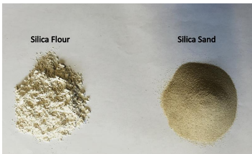
Figure 3.3 – Top view of aggregates used in the study
