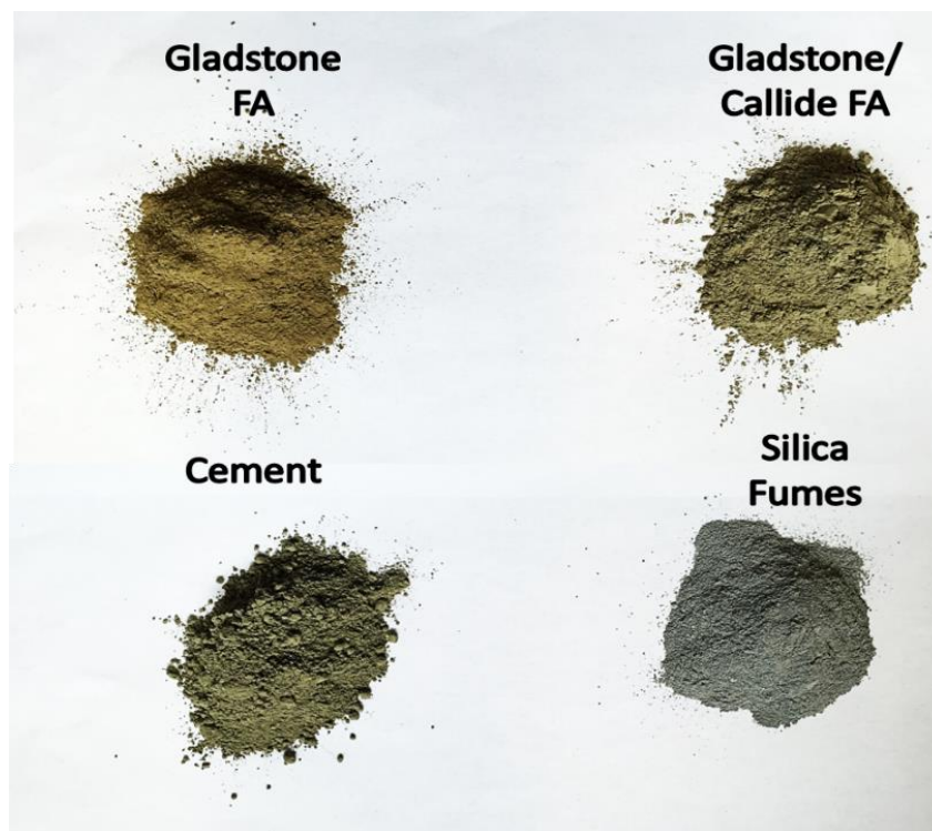
Figure 3.2 – Top view of cementitious materials used in the study
