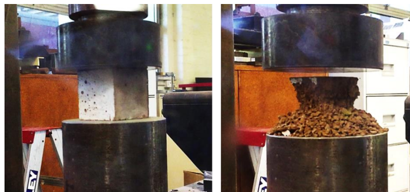
Figure 4.20– Specimen after high heat exposure before and after compression
