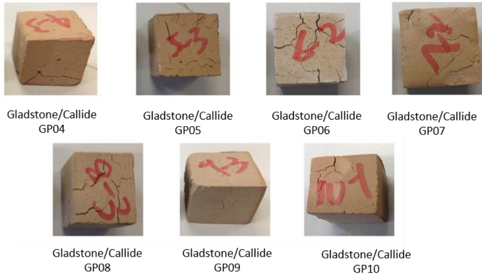
Figure 4.25 – Gladstone/Callide FA GP 25mm specimens after 800°C exposure
