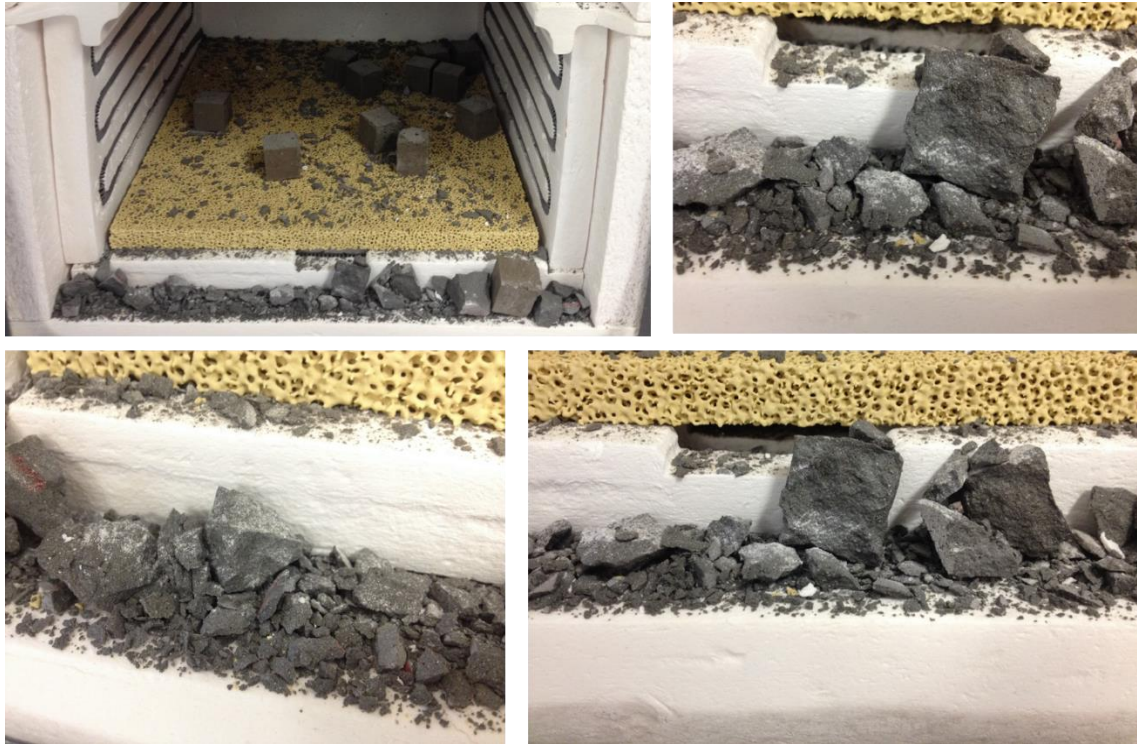
Figure 4.33 – RPC specimens after elevated temperature exposure
