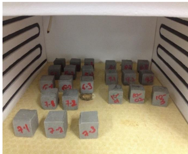
Figure 3.11 – Specimens placed inside the muffle furnace before exposure.
