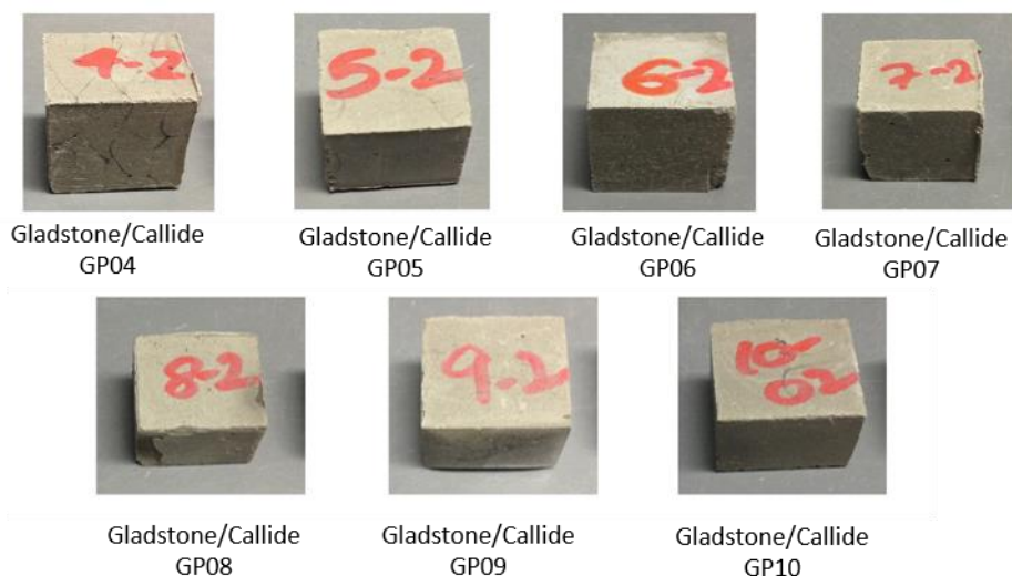
Figure 4.24 – Gladstone/Callide FA GP 25mm specimens after 400°C exposure
