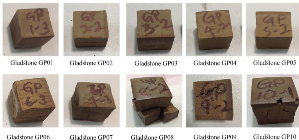
Figure 4.10 – Non-sealed Gladstone FA GP 25mm specimens–After 800°C exposure
