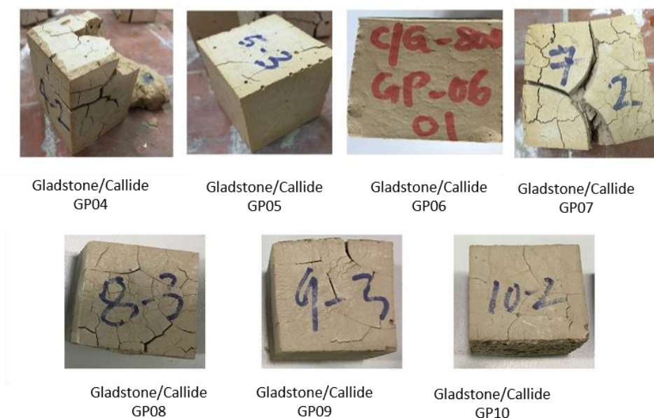
Figure 4.27 – Gladstone/Callide FA GP 50mm specimens after 800°C exposure
