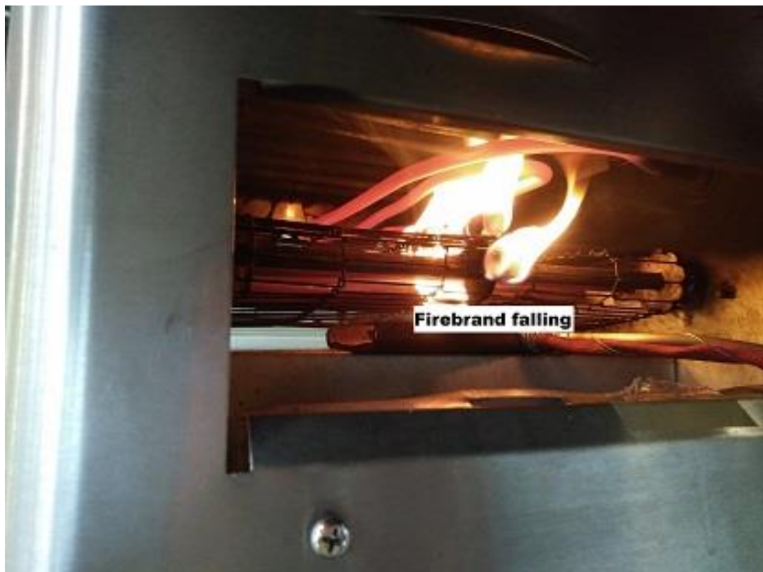
(b) Firebrand heater which ignites the firebrand before being fed to the VUSSG
