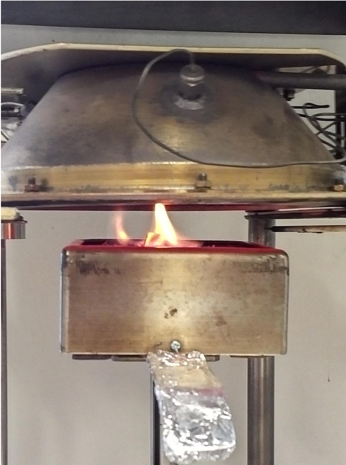
(a) ignition by firebrand in CC segment
