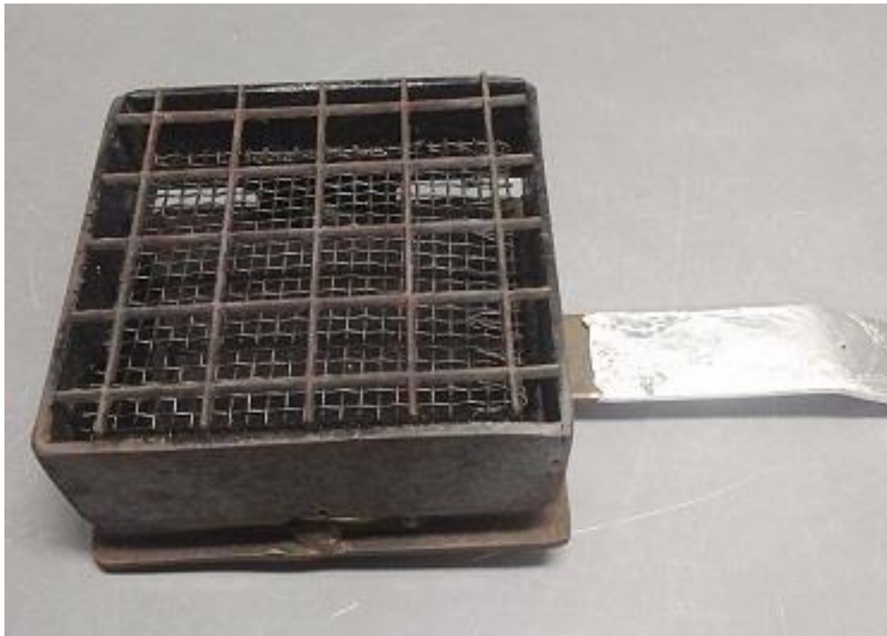
Fig. 5.3: Modified cone calorimeter sample holder with mesh base to allow air flow through the sample in OC, and when a retainer frame is placed blocks the flowing air through the mesh base leading to CC
