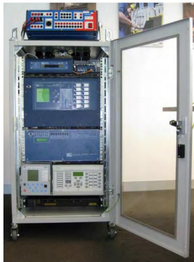
Figure 2: Portable IEC61850 Testing Unit developed by VU
