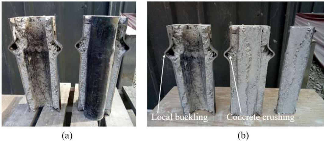
Fig. 6. Section view of Specimen SC1.
