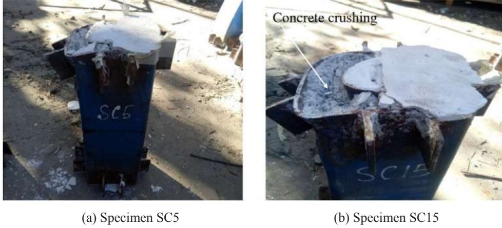
Fig. 11. Failure modes of Specimens SC5 and SC15.
