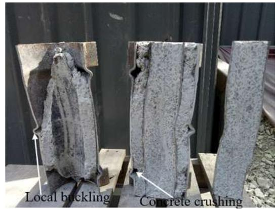
Fig. 5. Section view of Specimen CC10.
