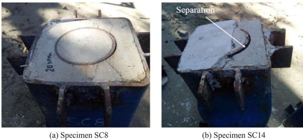
Fig. 10. Separation of sandwiched concrete and inner steel tube in Specimens SC8 and SC14.
