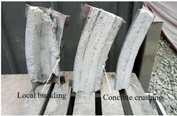
Fig. 10. Section view of Specimen CC13.
