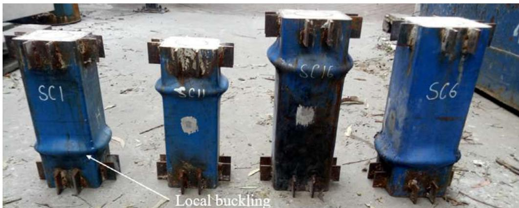
Fig. 5. Failure modes of square CFDST short columns under axial compression.
