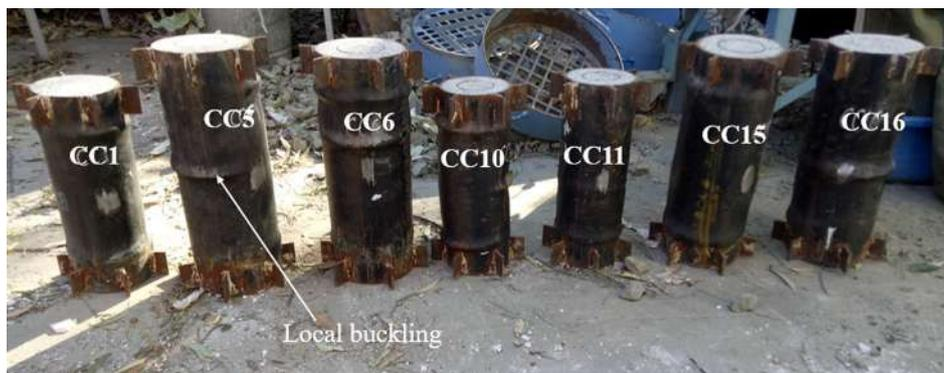
Fig. 4. Failure modes of axially loaded circular CFDST short columns.
