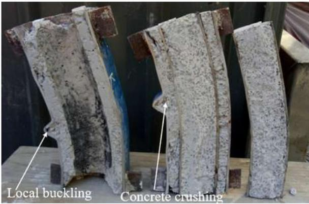
Fig. 12. Section view of Specimen SC14.
