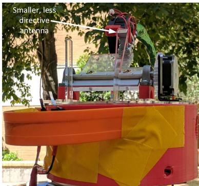
**FIGURE 3.** Modified receiver with 9.6 dBi antenna.
