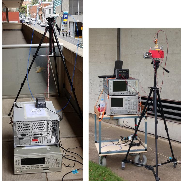
FIGURE 4.5: CW transmissions. (a) LHS Two signal generators, for Horizontal and Vertical polarisation (HP8360 and Agilent N5230A). Example frequencies: 39.499 GHz and 39.501 GHz (b) RHS Receiver with 2 LNAs (Miteq JS426004000-30-10P) feeding spectrum analyser (R& S FSIQ40).
