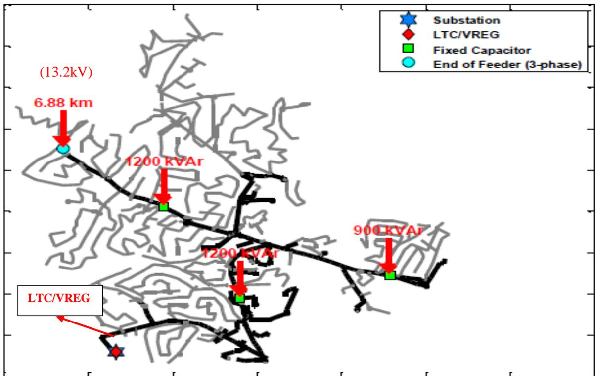
Fig. 3.1. EPRI CKT24 Network Diagram [81].
