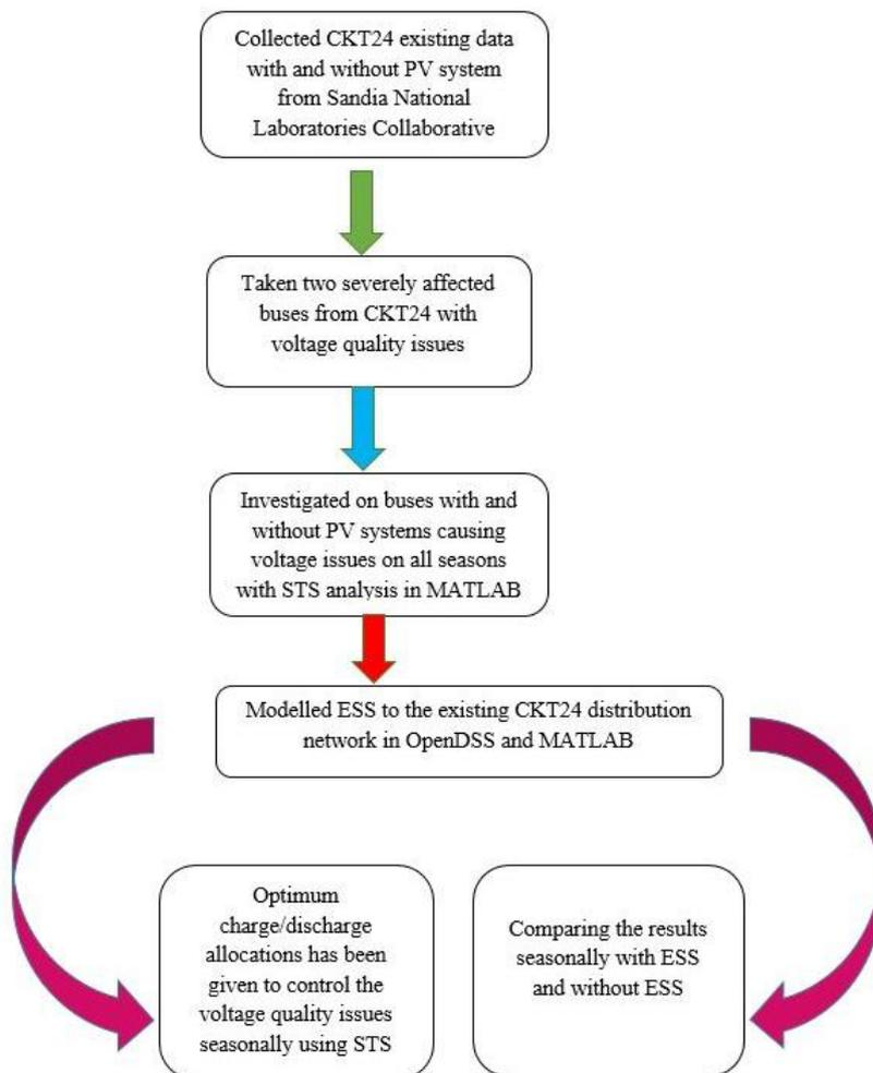
Fig. 1.1. A proposed methodology for the existing CKT24 distribution network.
