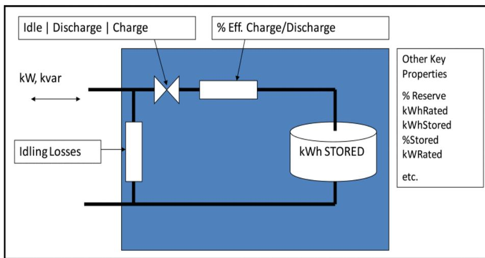
Fig. 4. 3. EPRI OpenDSS storage model basic concept [100].
