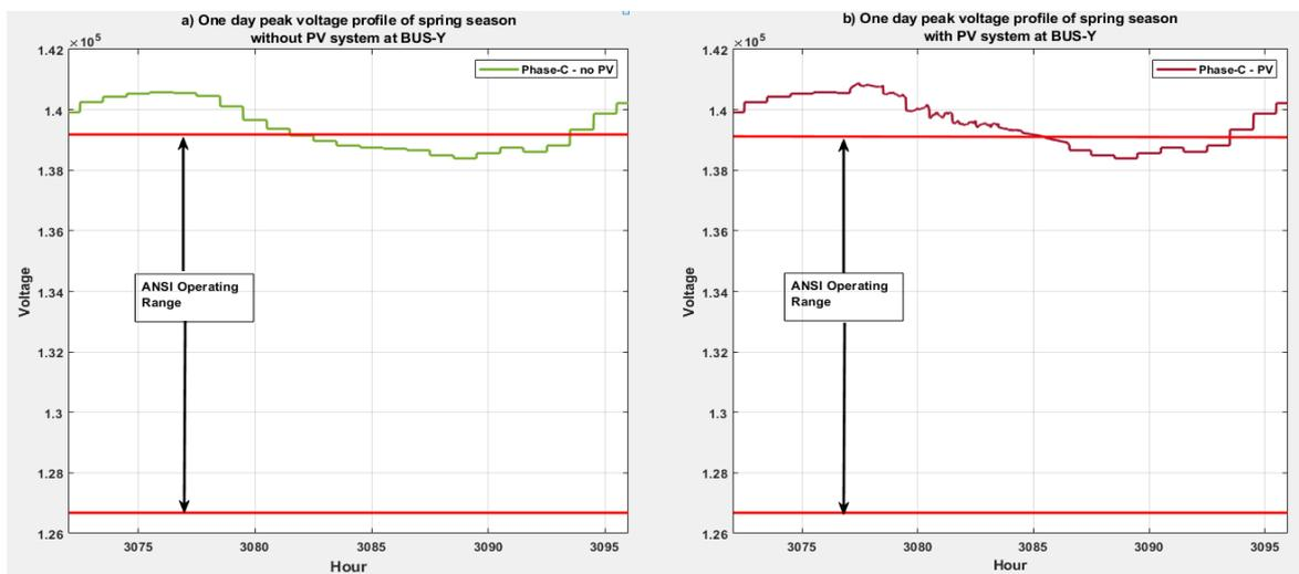
Fig. 3.13. Daily voltage profile in spring season with and without PV system at BUS-Y.
