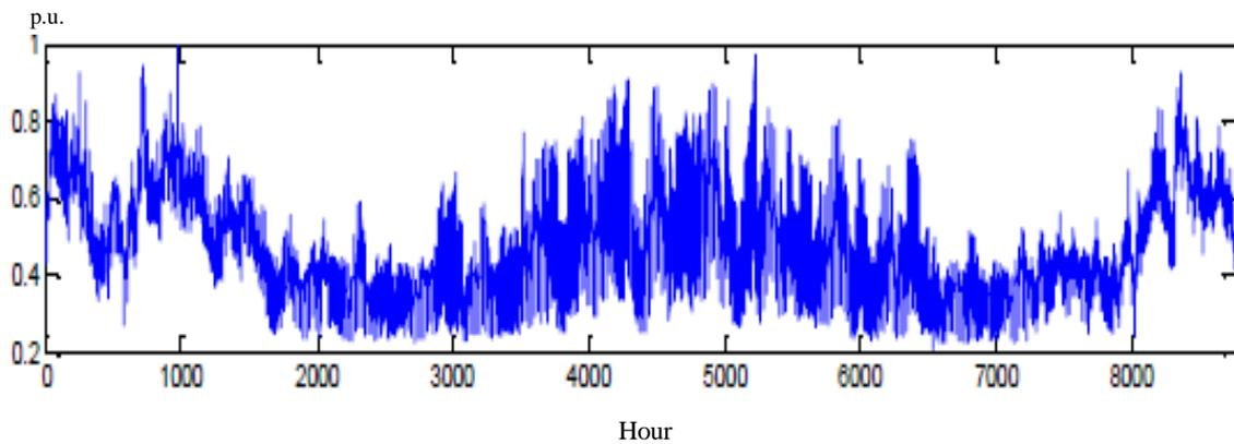
Fig. 3.3. Average Three Phase EPRI CKT24 load shape for one year [81].
