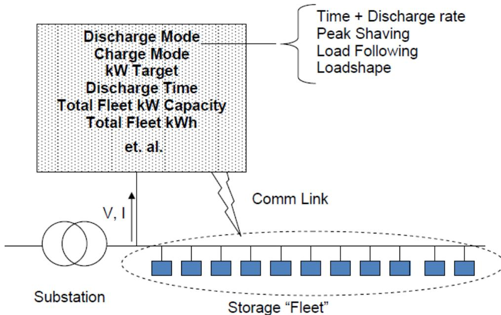
Fig. 4. 4. OpenDSS storage controller concept [100].
