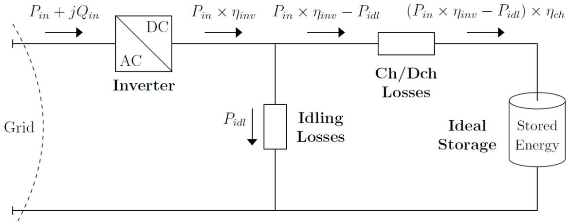
Fig. 4. 5. The Operation of a storage element in a charge state [101].
