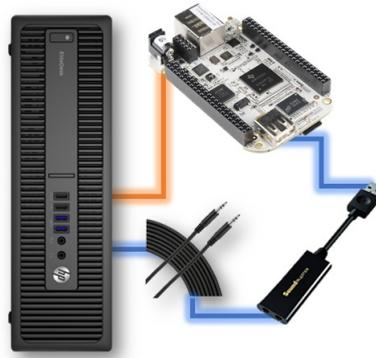
Figure 3.1. Experimental set-up. Blue lines indicate analog and digital signal paths, while the orange line represent a power/communication path.
