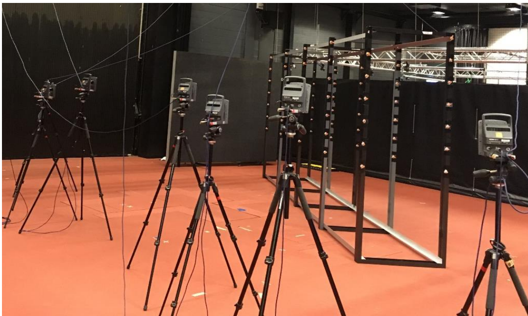
Figure 4.9 Marker location validation using seven-camera motion analysis system.
