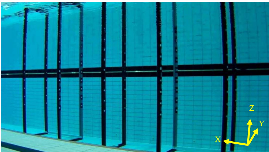
Figure 4.6 Underwater camera view of the calibration frame position in the pool (from FloorCam5 camera, Camera Frame 2).
