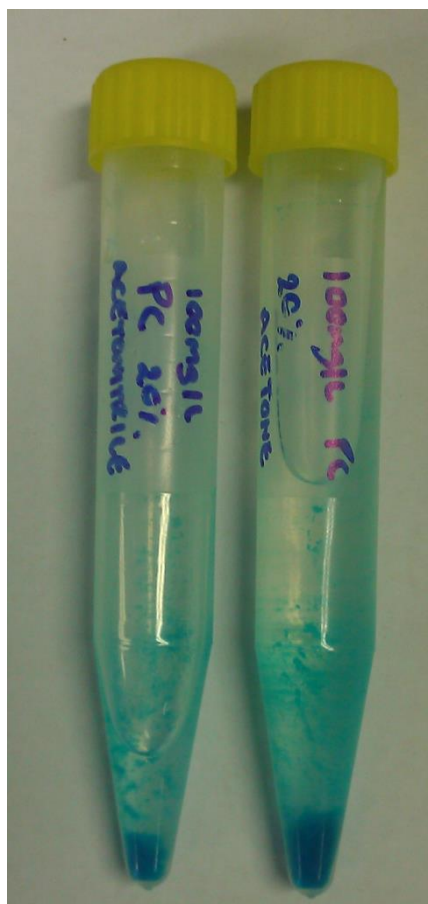
Figure 6.15: Precipitation of pure phycocyanin in 20% acetonitrile (left tube) and 20% acetone (right tube).
