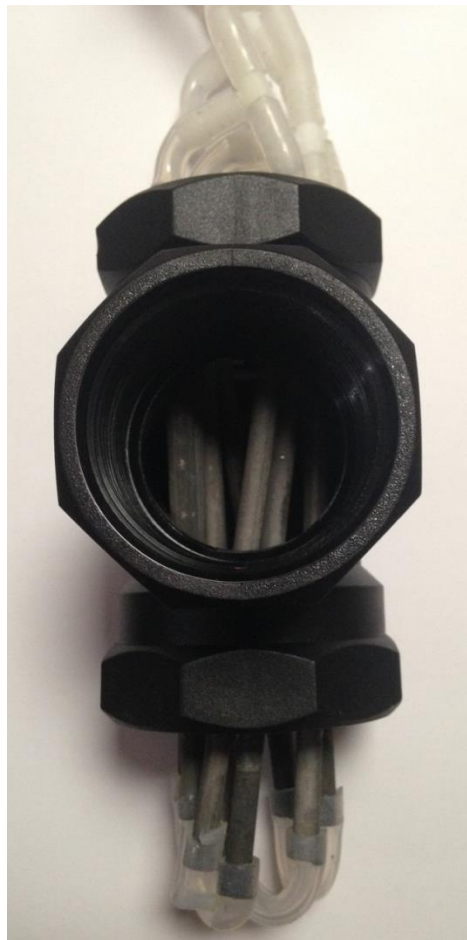
Figure 8.4: Tubular membranes used for cyanobacteria filtration.
