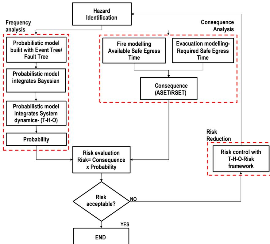
Figure 3: Specific enhancements to the general approach to probabilistic fire risk assessment provided in BSI PD 7974-7
