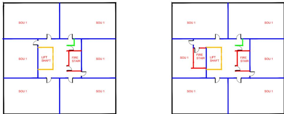
Figure 3. Case #2—Performance (left) and DTS (right) solutions.
