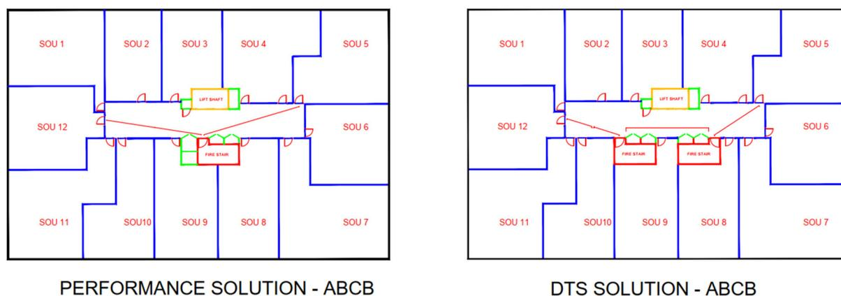
**Figure 2.** Two solutions for Case #1 Australian Building Codes Board (ABCB) model residential building.
