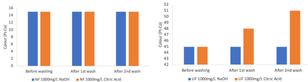
**Figure 6.6.** Colour removal of NF (left) and UF (right) being cleaned with 1000 mg/L NaOH and citric acid (Feed colour = 1343 Pt-Co)
