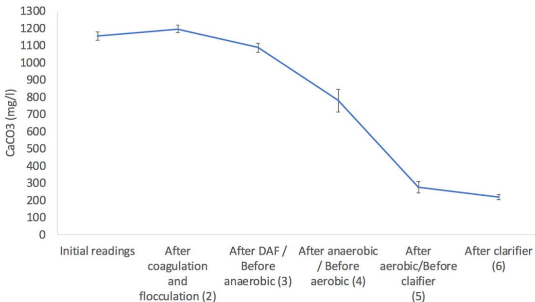
**Figure 4.7.** Hardness values at each point of the wastewater treatment process
