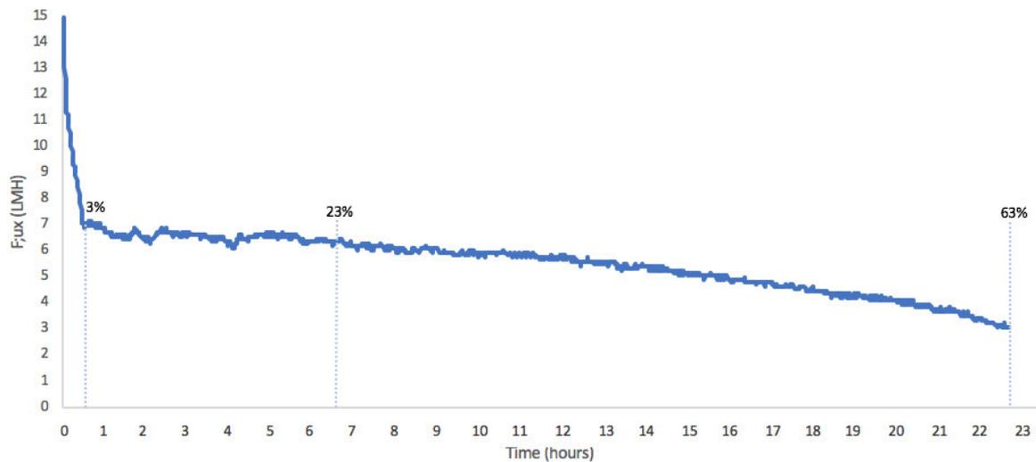
**Figure 6.3.** NF fouling trend when flux experienced an 80% reduction.
