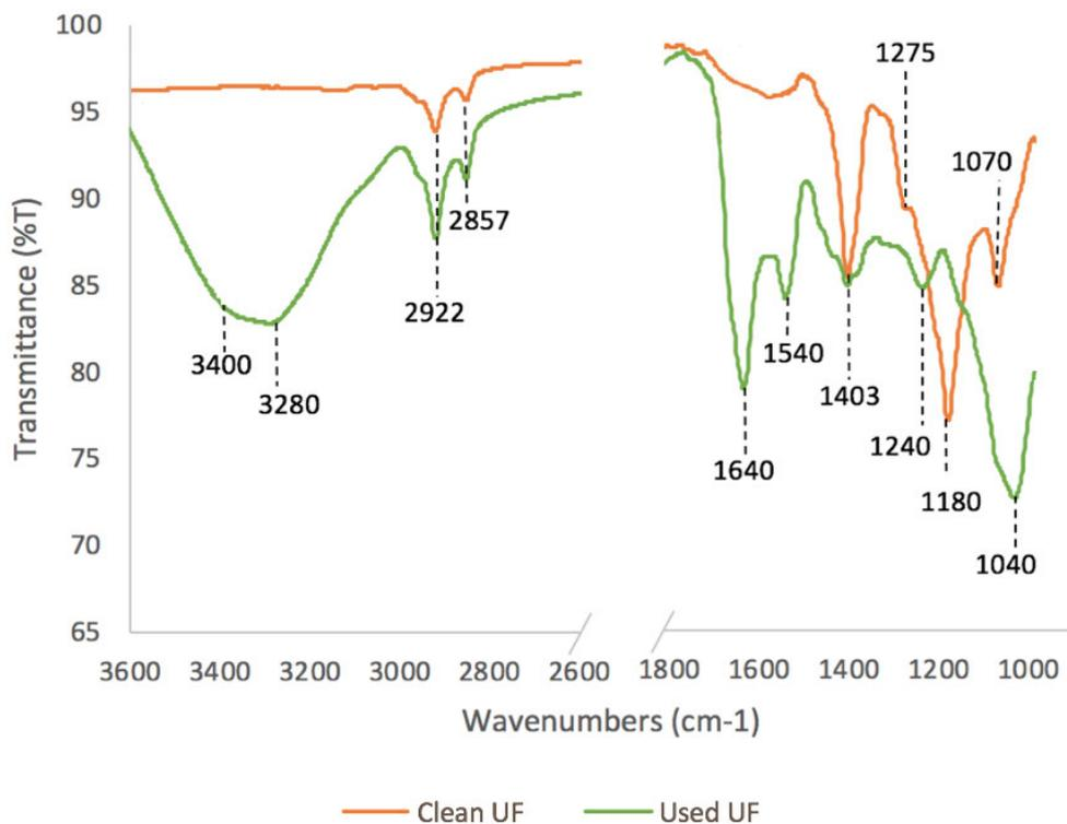
**Figure 6.13.** FTIR spectra of clean and used UF membrane.
