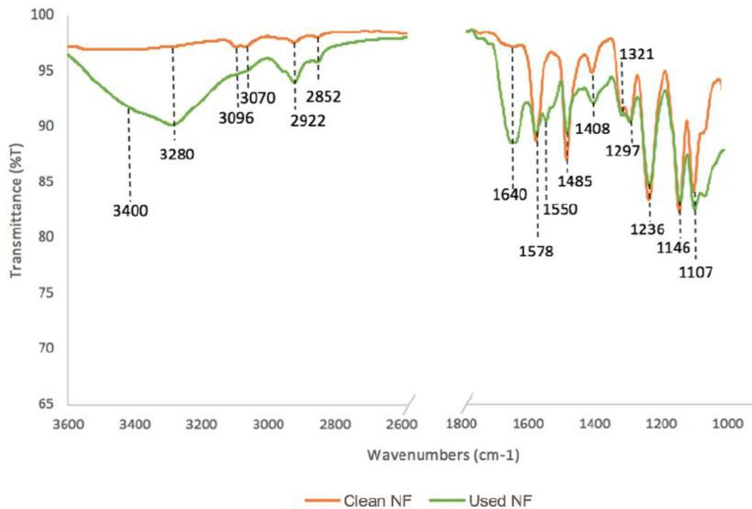
**Figure 6.14.** FTIR spectra of virgin and fouled NF membrane.
