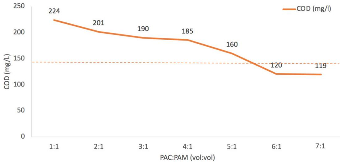
**Figure 5.3.** Enhanced coagulation and flocculation with different PAC:PAM (vol:vol) ratios for COD removal.
