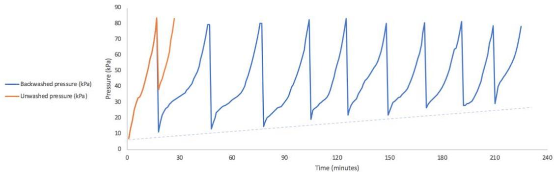
**Figure 6.8.** The effect of backwashing on UF membrane.
