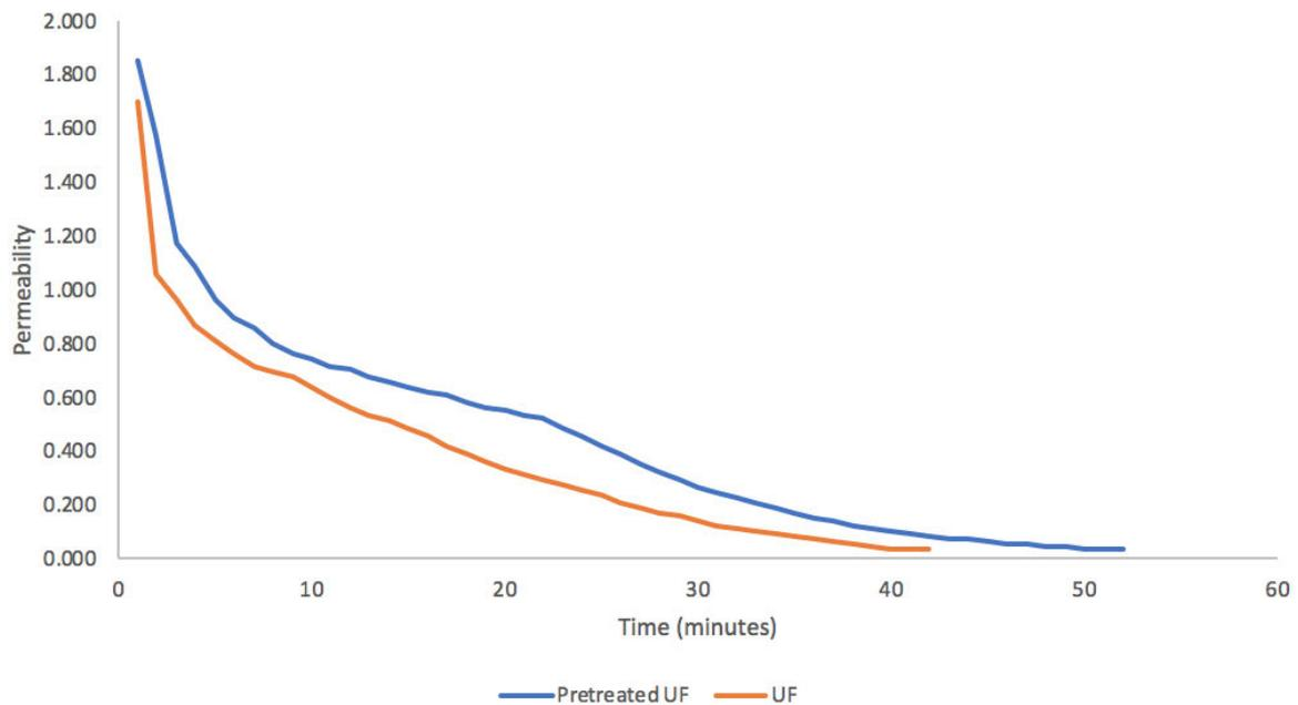
**Figure 6.11.** Permeability of UF membrane without pretreatment and UF membrane pretreated with coagulant.
