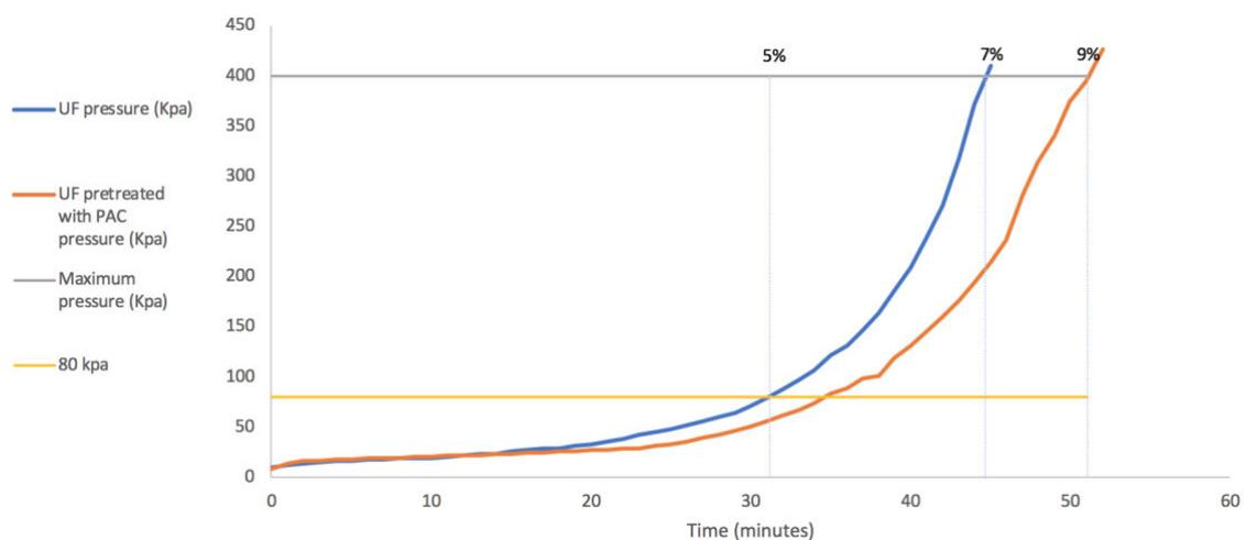
**Figure 6.9.** Fouling trend of UF compared to pre-treated UF
