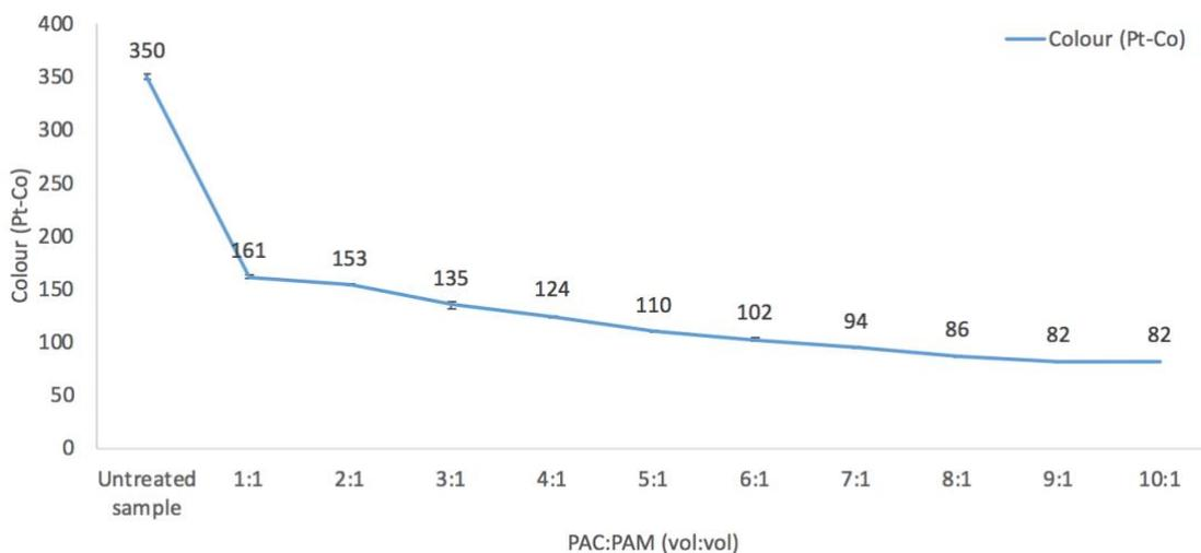
**Figure 5.2.** Colour removal efficiency of different PAC:PAM (vol:vol) ratios given a fixed amount of PAM and an increasing amount of PAC.
