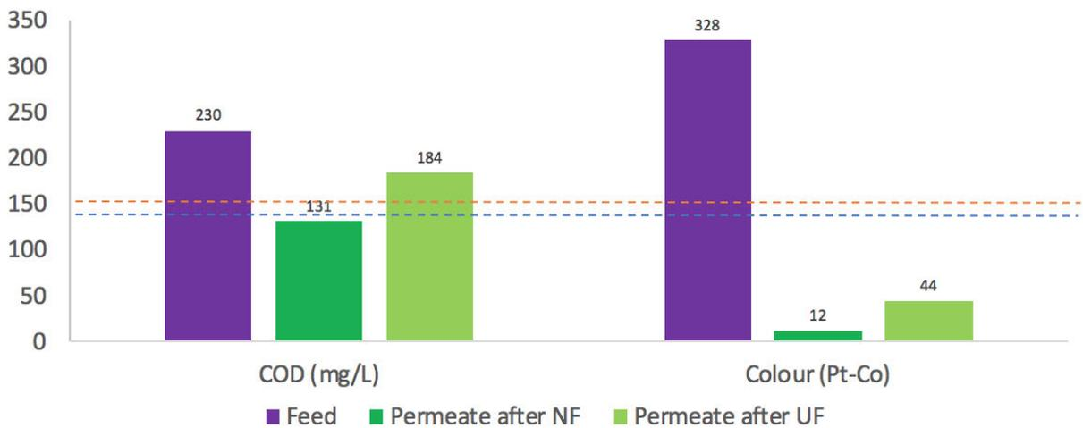
**Figure 6.2.** Colour and COD removal efficiency using simulated biologically treated wastewater.
