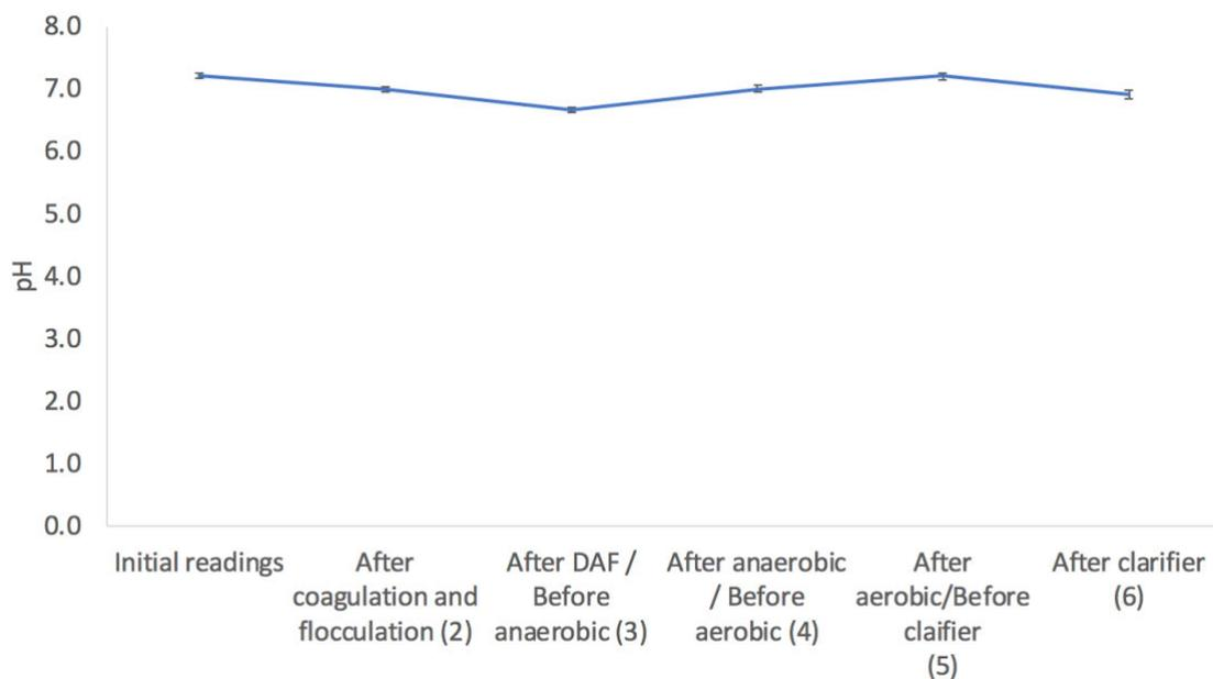
**Figure 4.8.** pH values at each point of the wastewater treatment process.
