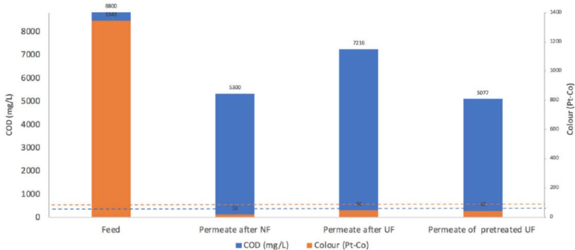
**Figure 6.10.** Colour and COD rejection rates of NF and UF compared to pre-treated UF for untreated effluent.
