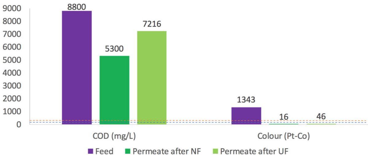
**Figure 6.1.** Colour and COD removal efficiency using untreated recycled paper mill wastewater
