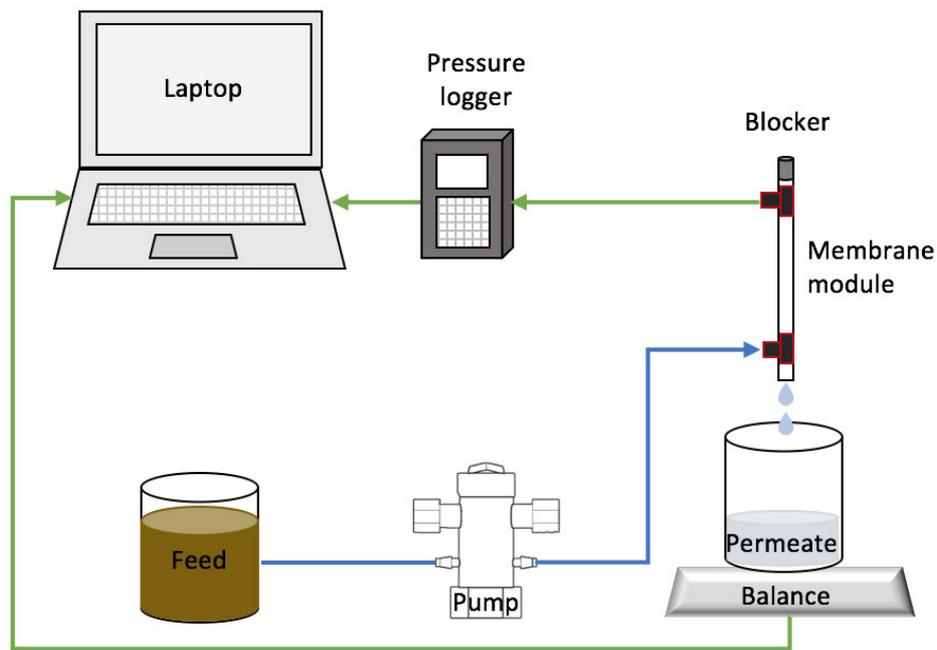
**Figure 3.1.** UF membrane rigs in outside-inside and dead-end mode.
