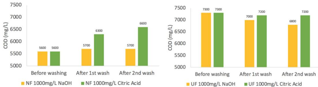
**Figure 6.7.** COD rejection of NF (left) and UF (right) after cleaned with 1,000 mg/L NaOH and citric acid (Feed COD = 8,800 mg/L).
