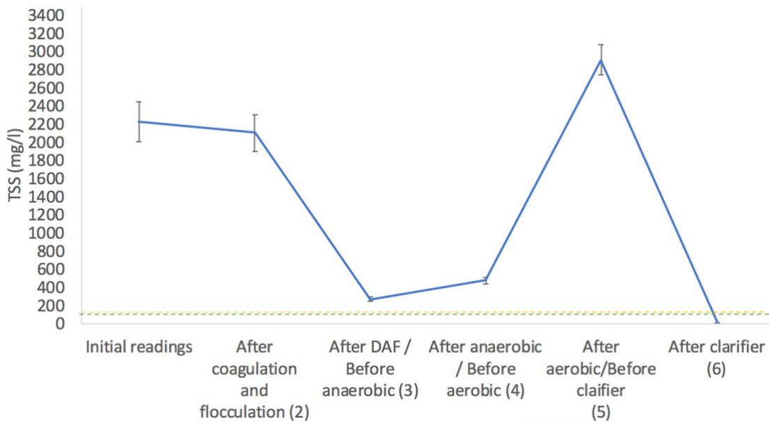
**Figure 4.6.** Total suspended solids values at each point of the wastewater treatment process.
