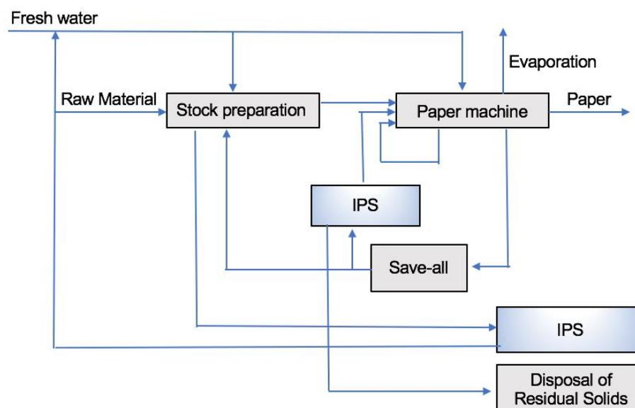
**Figure 2.1.** An example of a completely closed process water loop with integrated purification systems (IPSs). (Adapted from Hamm and Schabel, 2007).
