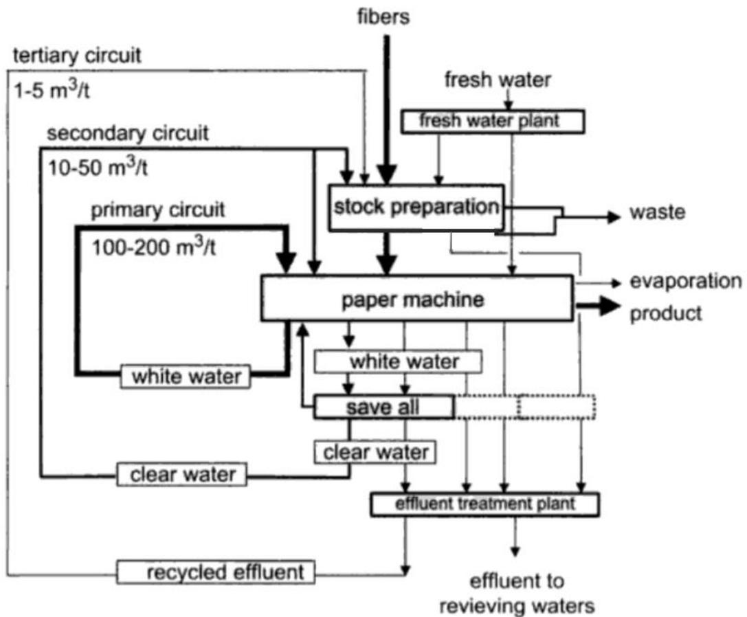
**Figure 1.1.** Simplified water system of a pulp and paper mill and its water recycling opportunities (Blanco et al., 2015).
