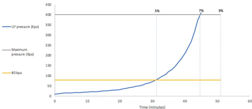
**Figure 6.4.** UF fouling trend when pressure reached the critical threshold.
