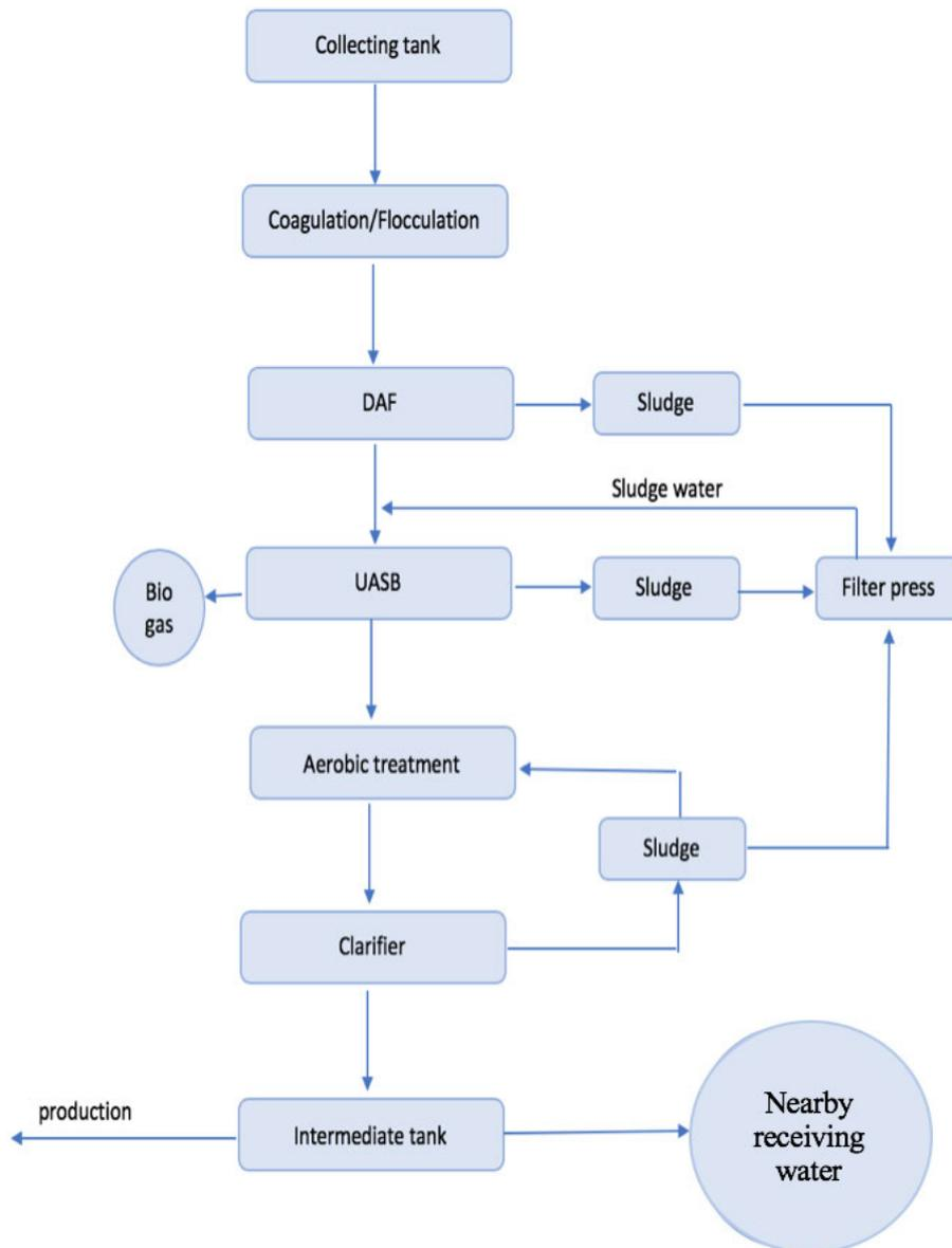
**Figure 4.2.** An Binh's wastewater treatment system
