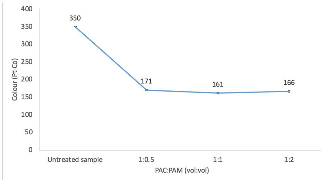
**Figure 5.1.** Colour removal efficiency of different PAC:PAM (vol:vol) ratios given a fixed amount of PAC and an increasing amount of PAM.
