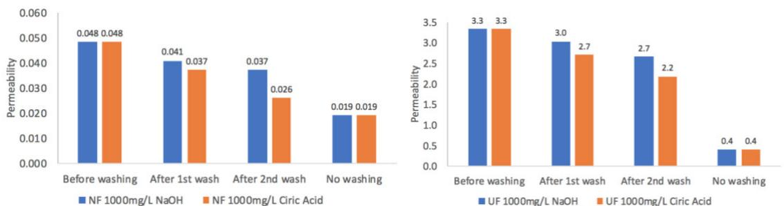
**Figure 6.5.** Permeability of NF (left) and UF (right) being cleaned with 1000 mg/L of NaOH and 1000 mg/L of citric acid separately.
