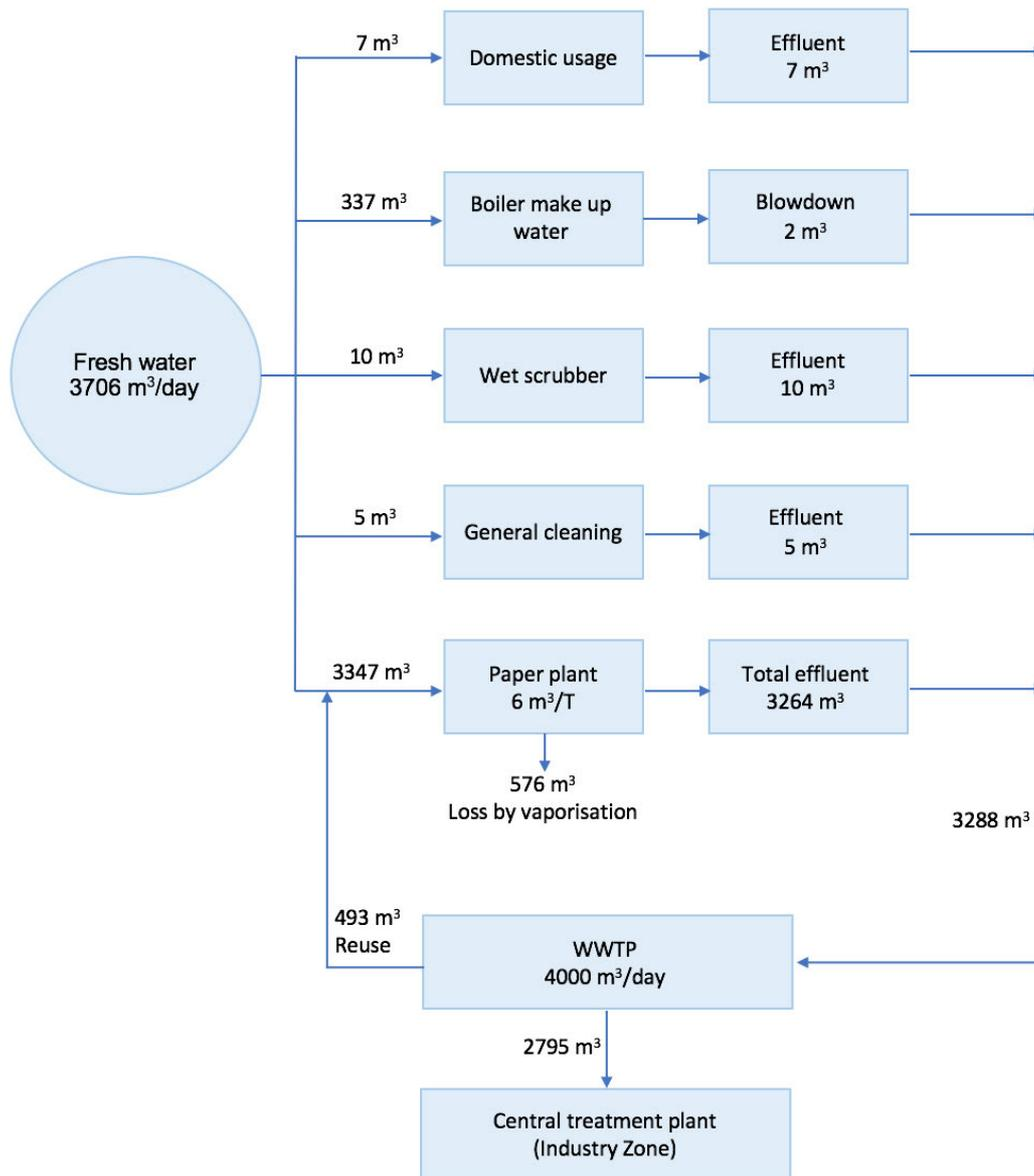
**Figure 4.10.** A proposed water balance for Khoi Nguyen using 6 m<sup>3</sup> fresh water/T product, giving it a production capacity of roughly 180000 tonnes/year.
