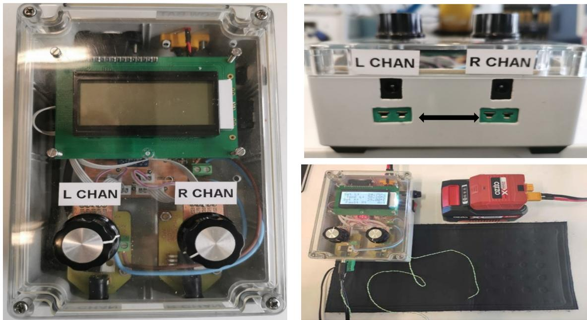
Figure 2.2. The power regulator platform comprised of two separate outputs for simultaneous use on two targets. The regulator platform controls the power output provided by 12V volt battery pack.
