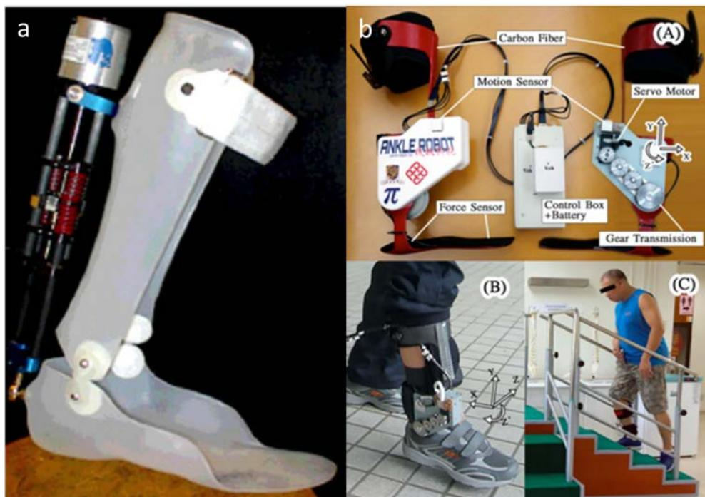
Figure 2.5 Electromechanics active AFOs. Adapted from a) (Blaya & Herr, 2004) and b) (Yeung et al., 2017).
