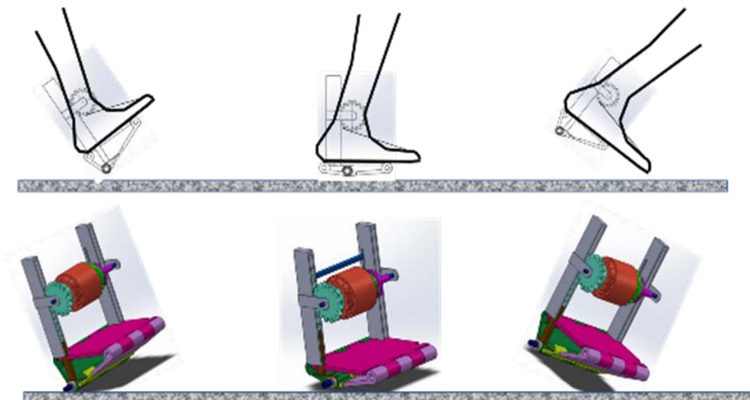
Figure 5.3 One concept developed for a harvest-store-release-reset sequence in each step.
