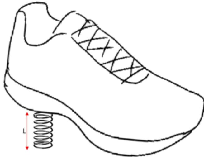
Figure 5.2 Simple mechanism to harvest heel strike energy using a compressive spring.
