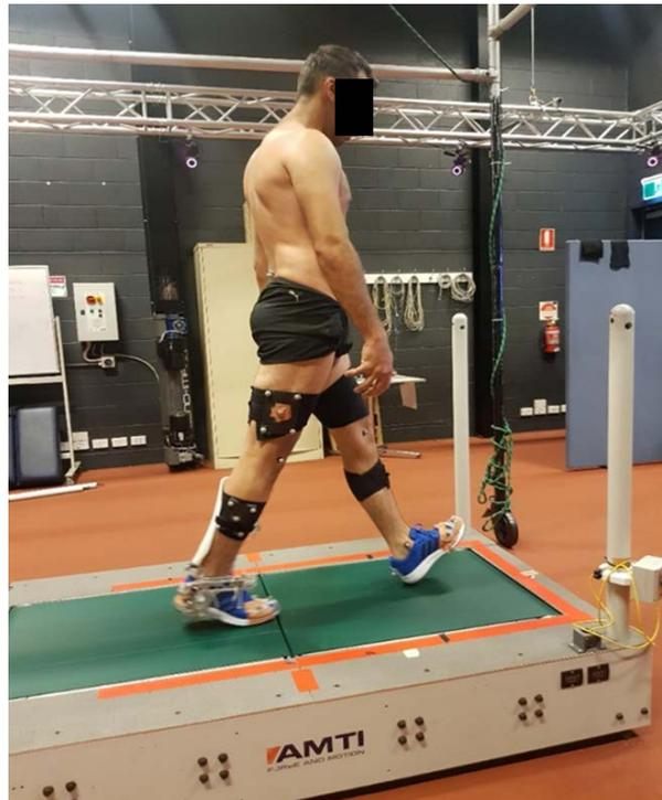
Figure 6.1 Experimental Setup. The Vicon default lower body marker set with four additional marker clusters attached to the thigh and shank of both legs. Upper body markers were discarded.
