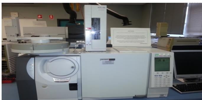
Figure 3.3.4 Shimadzu GC-MS equipment (from our work)
