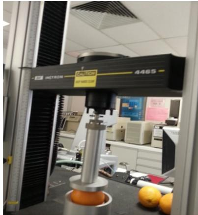
Figure 3.7.2 Instron Universal Testing Equipment used
