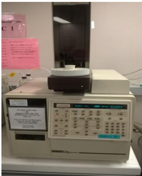
Figure 3.3.5 GC equipment used in the study of freeze treated orange skin oil and control sample (from our work).
