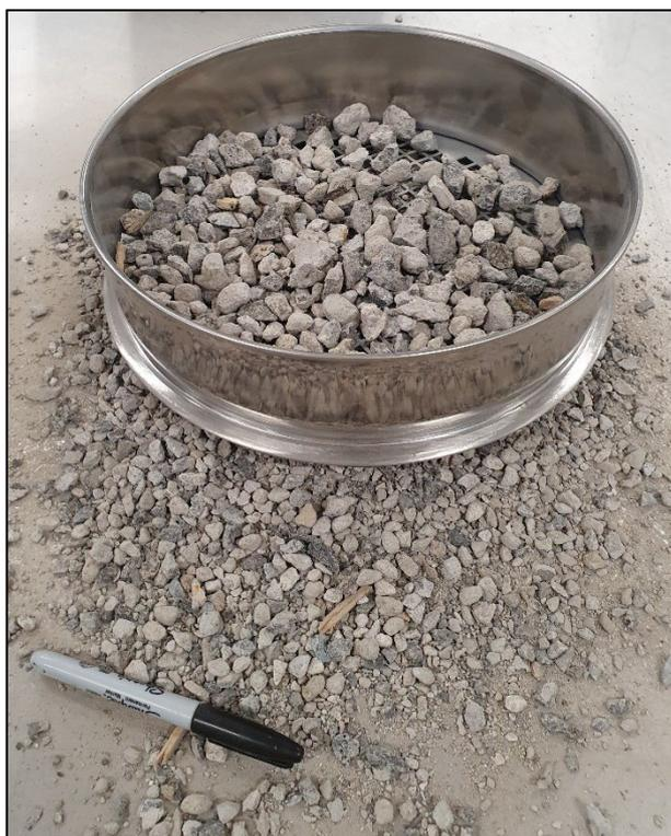
Figure 7 RCA sieved through the 9.5 mm sieve.
