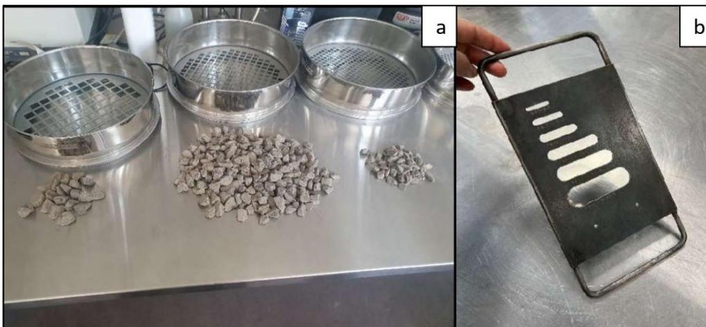
Figure 10 Images showing a) aggregate separated based on particle size using sieves, and b) Flakiness Index gauge.
