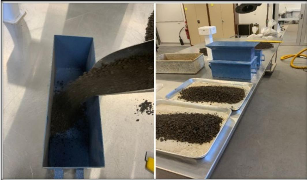
Figure 8 Aggregate quartering process using sample splitter.
