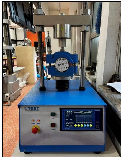
Figure 14 Image showing Marshall Stability testing equipment.
