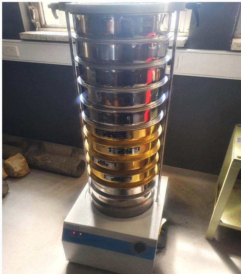
Figure 9 The set of sieves used for the determination of the PSD.
