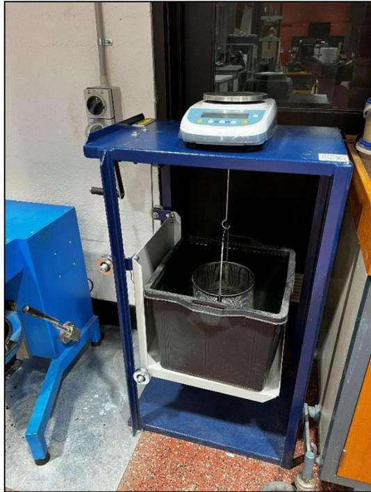
Figure 13 Weigh-in-water balance used for bulk density testing.
