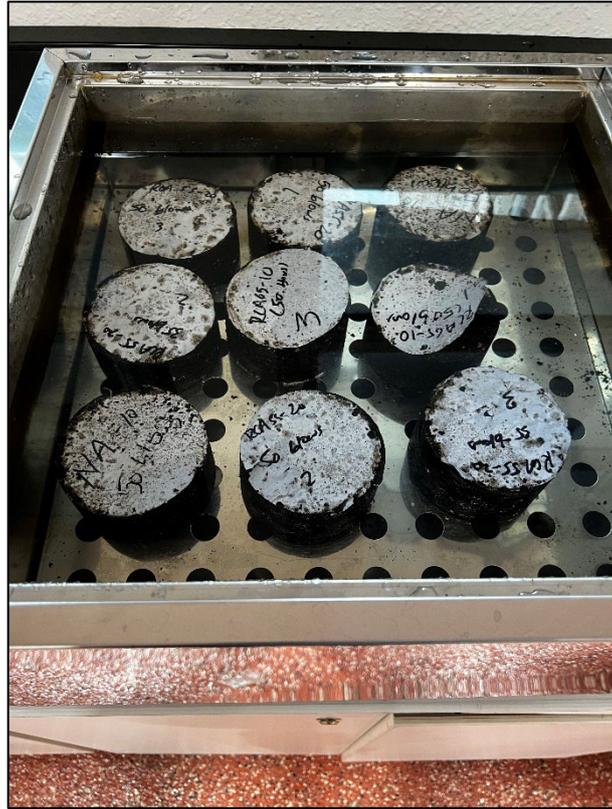
Figure 16 Water bath with test specimens inside.
