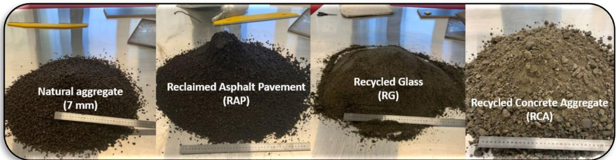
Figure 6 Images of the used aggregates in their wet state.
