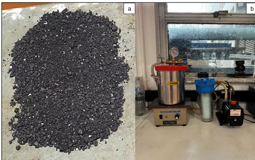
Figure 11 Images showing a) a loose asphalt mixture sample b) maximum theoretical density testing equipment setup.
