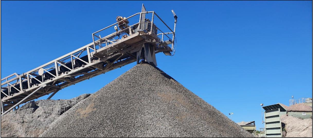
Figure 5 Pile of Class 2 RCA, Delta Group.
