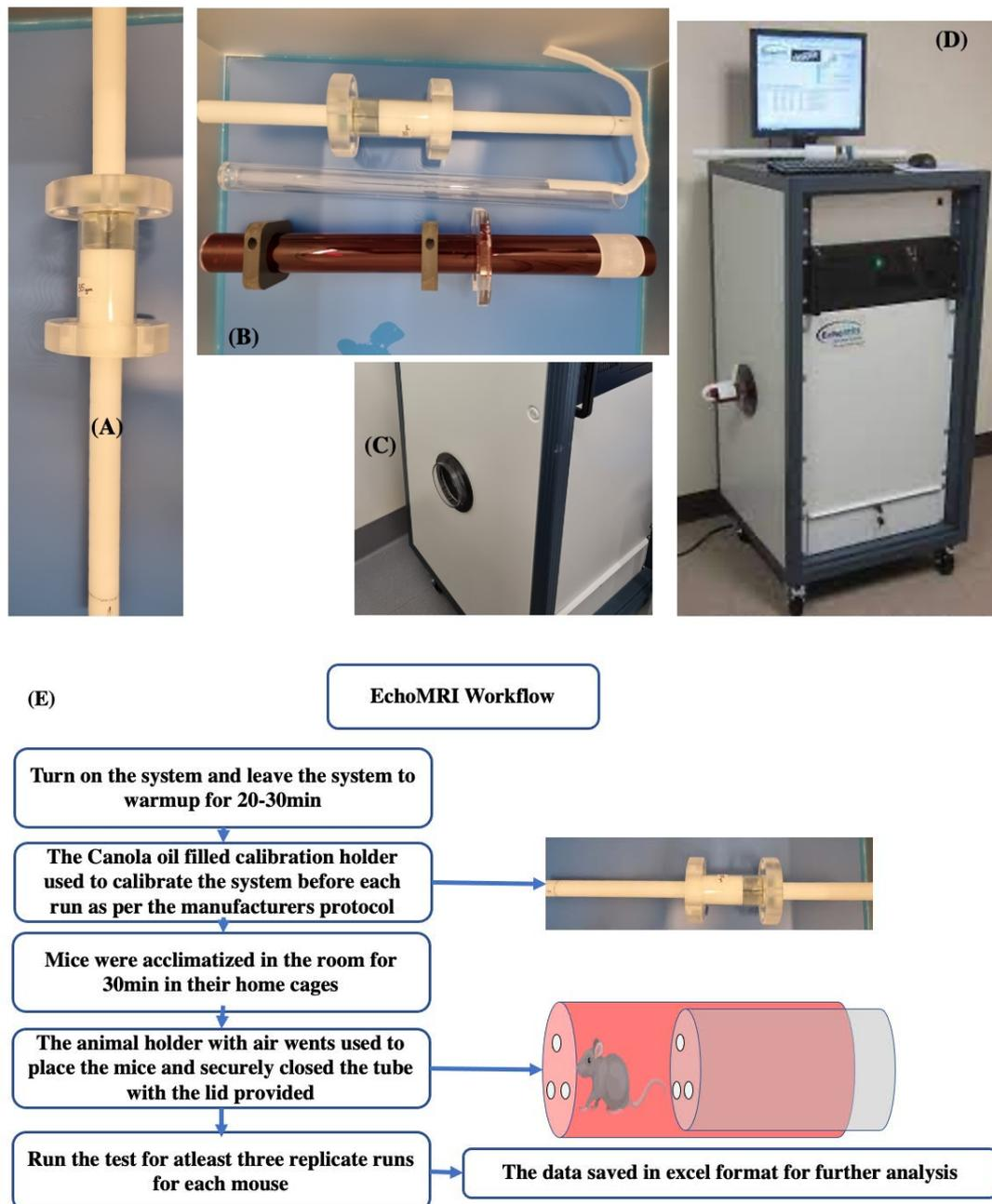
**Figure 5.1:** EchoMRI-900 and workflow of the body composition measurement: (A) Canola oil holder for EchoMRI calibration with fat content of 35.68g, (B) The red holder is used to place the animal to measure the body composition, (C) The slot to place the animal holder into the instrument, (D) After placing the animal holder into the system, and (E) workflow of EchoMRI to measure the mice body composition.
