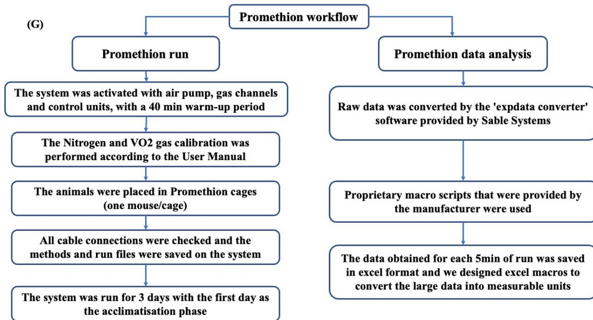
**Figure 5.2:** Components of Promethion cage and workflow of Promethion metabolic cage monitoring: (A) Promethion cage base with gas channel, (B) and (C) cage lid with mass module inserts, (D) Different hoppers that can go with each mass module in the cage, (E) Hoppers hanging to the respective mass module, (F) Gas tubes connected to the gas channel in the cage and (G) Overall brief workflow of Promethion system handling
