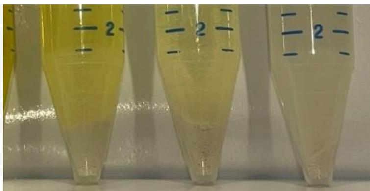
**Figure 3.13: Example of precipitate formed at bottom of an MEC anode sample**
