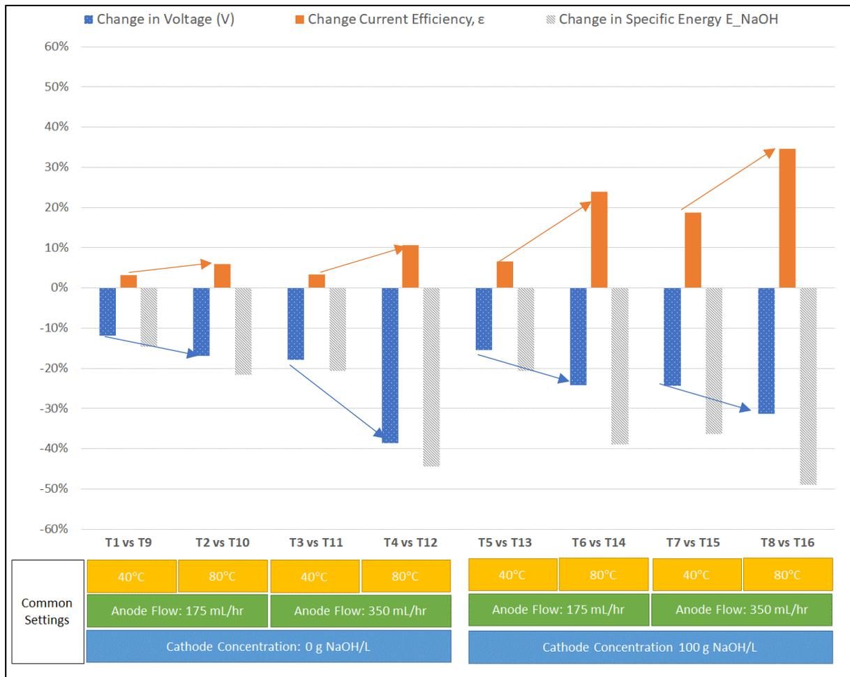
**Figure 5.8: Effect of Increasing Anode Feed Concentration (100 to 200 g/L) on MEC Performance at 1.39 kA/m<sup>2</sup> (5 A), arrows indicate effect of increasing temperature.**
