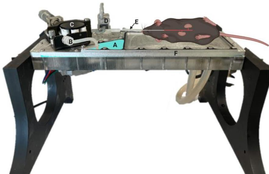
**Figure A1.** Renal perfusion setup with a graphical representation of the mouse. The main key features in the setup include **A.** KREBS/Drug well, **B.** tubes perfusing KREBS A to kidney, **C.** peristaltic pump, **D.** pressure sensor, **E.** microtube inserted into thoracic aorta and towards the renal artery, and **F.** heated plate maintained at 37°C.
