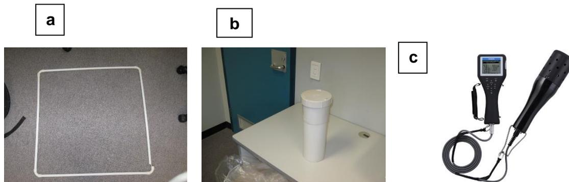
**Figure 2.6:** (a) 50 cm X 50 cm Quadrat used to randomly find sample – Source: own image; (b) 10 cm internal diameter by 26 cm length of PVC pipe used to collect seagrass and sediment sample – Source: own image; (c) Horiba U-50 – Source: [https://www.horiba.com/en\\_en/products/detail/action/show/Product/u-50-434/](https://www.horiba.com/en_en/products/detail/action/show/Product/u-50-434/)
