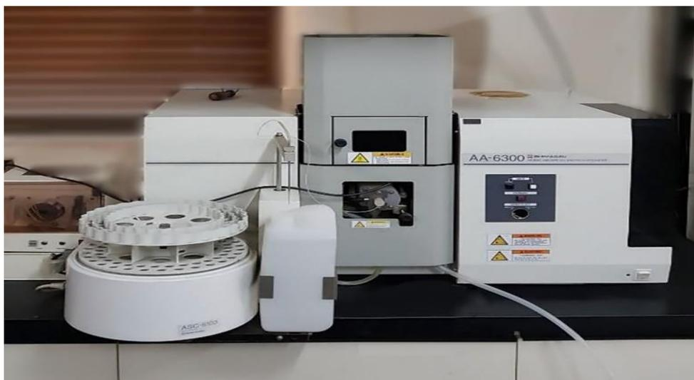
**Figure 2.9:** Shimadzu Atomic Absorption Spectrophotometer AA-6300 used to validate the ICP-AES samples. Source - <https://caeonline.com/buy/spectrophotometers/shimadzu-aa-6300/9241714>
