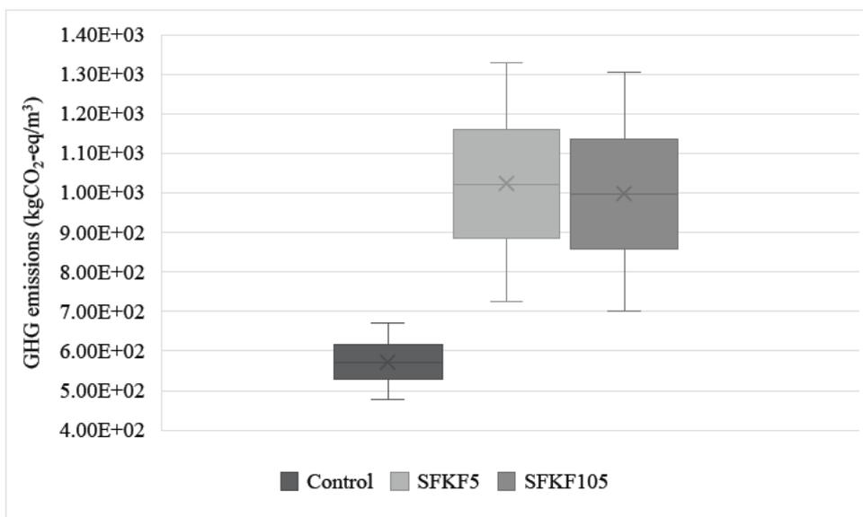
**Figure 9** Total GHG emissions for 1m<sup>3</sup> concrete
