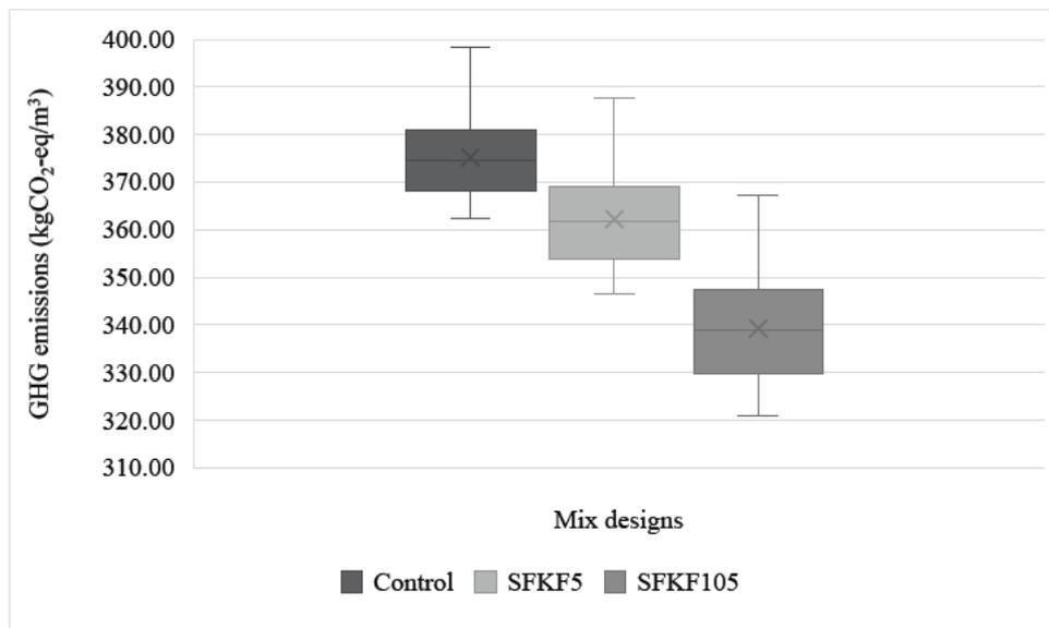
**Figure 6** Transportation and material GHG emissions of 1m<sup>3</sup> concrete materials
