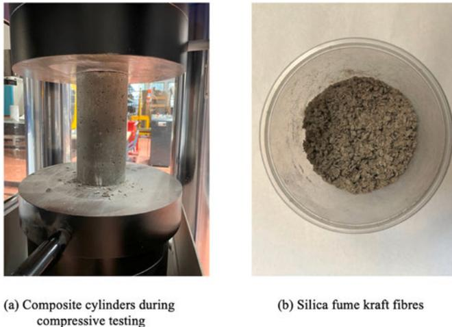
**Fig. 5.** Sample of the novel composite and KFs.
