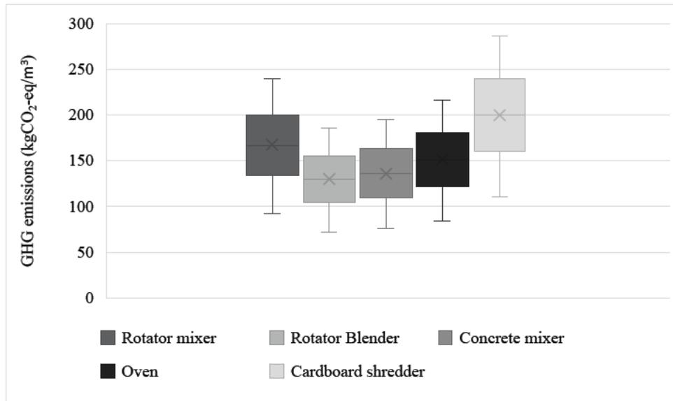
**Figure 11** Equipment variation of GHG emissions produced for 60- 300-minute usage
