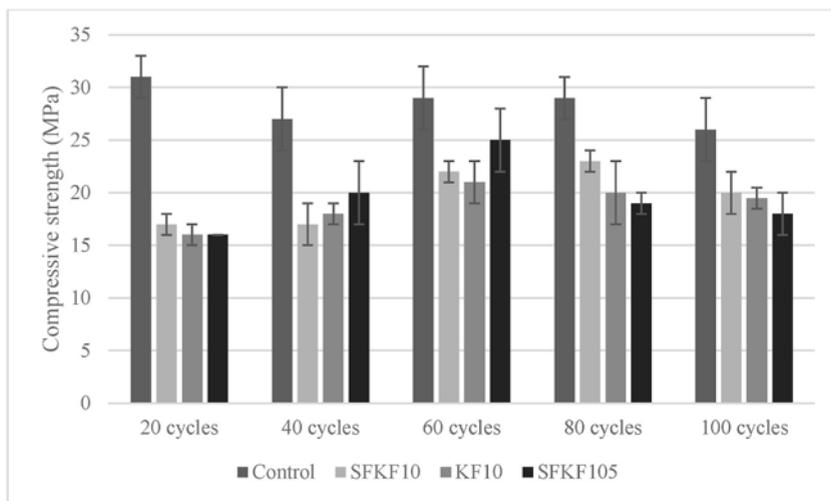
Fig. 9. Compressive strength vs wet/dry cycles.
