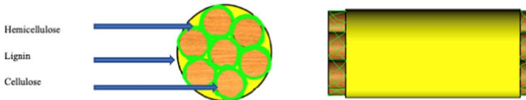
Fig. 6. Components of NFs. Redrawn from [48].
