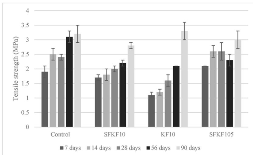
Fig. 7. Tensile strength at various ages.
