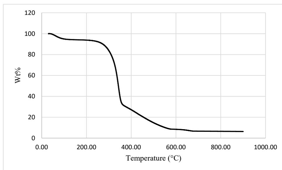
**Figure 3.** Thermogram obtained for CB sample at a heating rate of 10 °C min<sup>-1</sup> in nitrogen.
