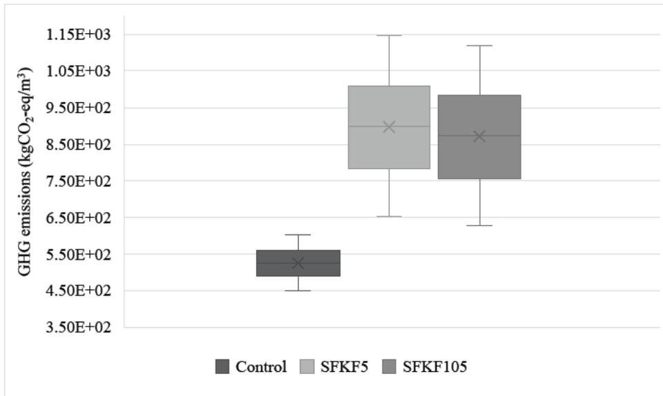
**Figure 8** Material and manufacturing GHG emissions for 1m<sup>3</sup> concrete
