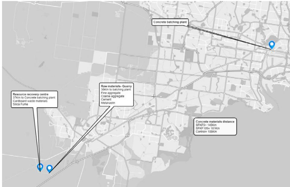
**Figure 7** Travel distances for materials to concrete batching plant
