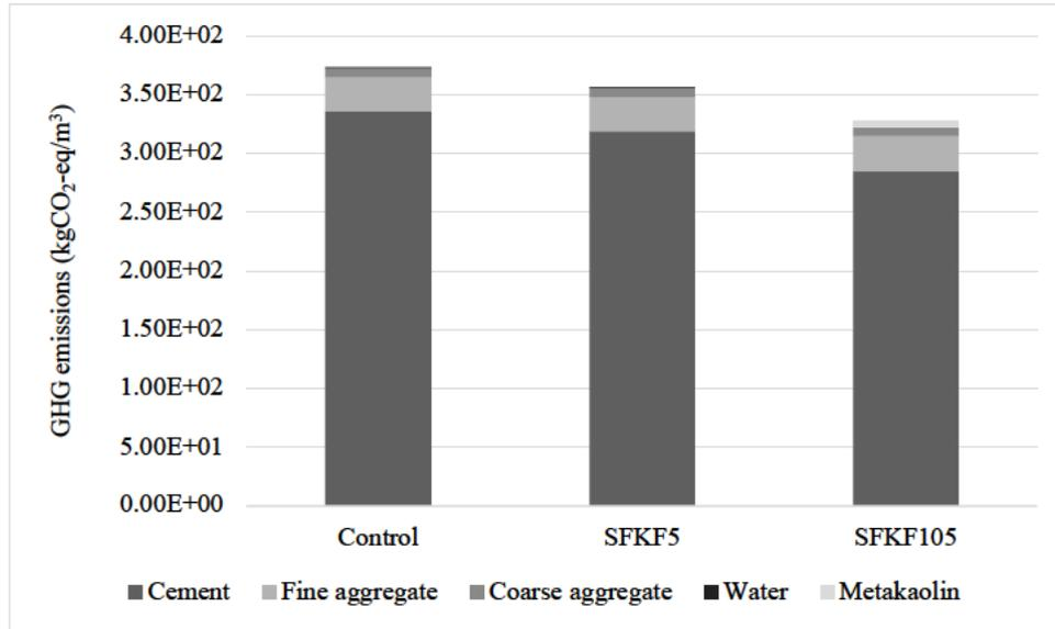
**Figure 5** GHG emissions of concrete composites (1m<sup>3</sup>)
