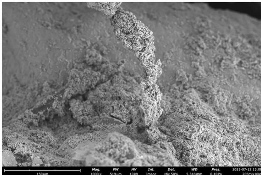
Fig. 5. Total petrification of KF walls.
