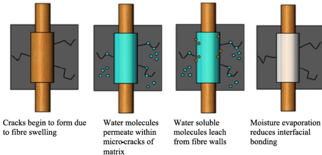
Fig. 5. Consequence of NFs containing moisture within composite matrix. Redrawn from [40].
