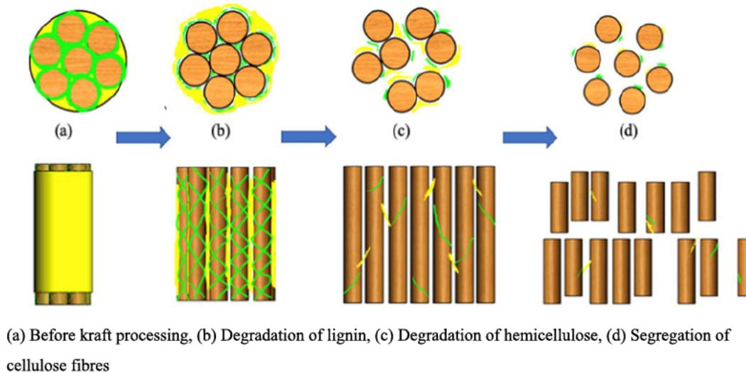
Fig. 7. Kraft transformation process of NFs. Redrawn from [48].
