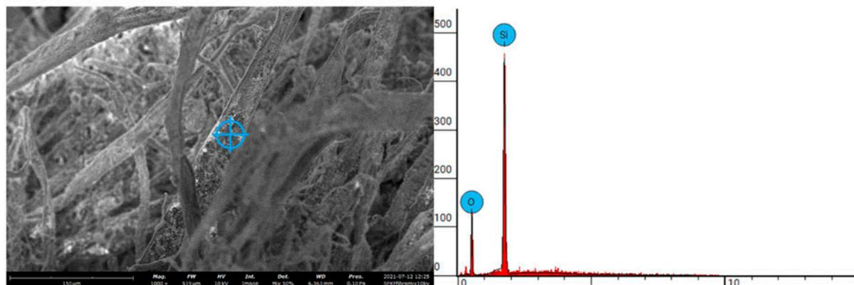
**Figure 5.** SEM/EDS report of SF on fibre.
