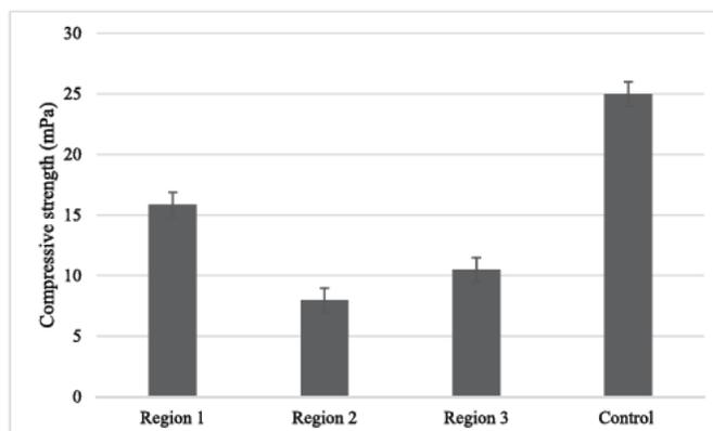
Fig. 4. Compressive strength results for optimised mix design regions.
