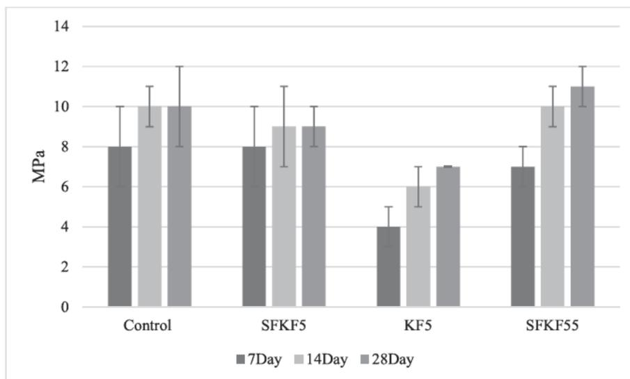
Fig. 8. Variation of tensile strength.
