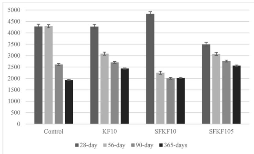
Fig. 3. Charge passed through specimens.
