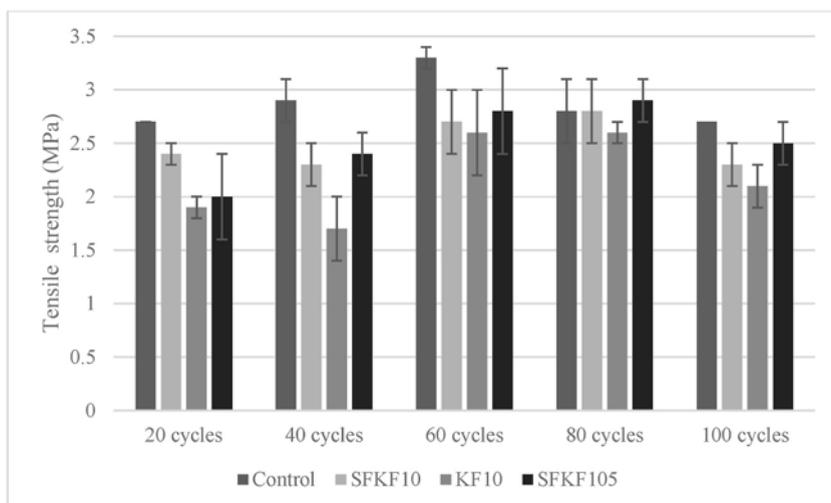
Fig. 10. Tensile strength vs wet/dry cycles.
