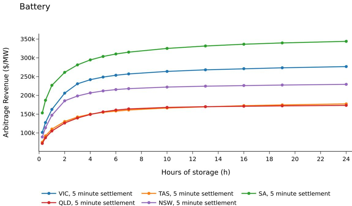
**Figure 36. Difference between battery storage and PH Arbitrage Revenue**
