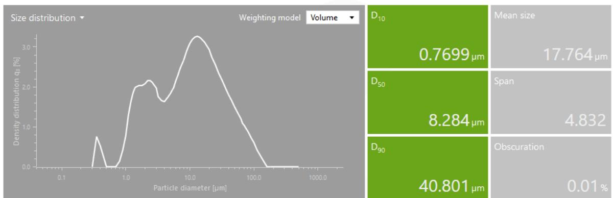
**Figure 3.9:** Particle size measurement for developed iron oxide nanoparticle with 4 grams zeolite added.
