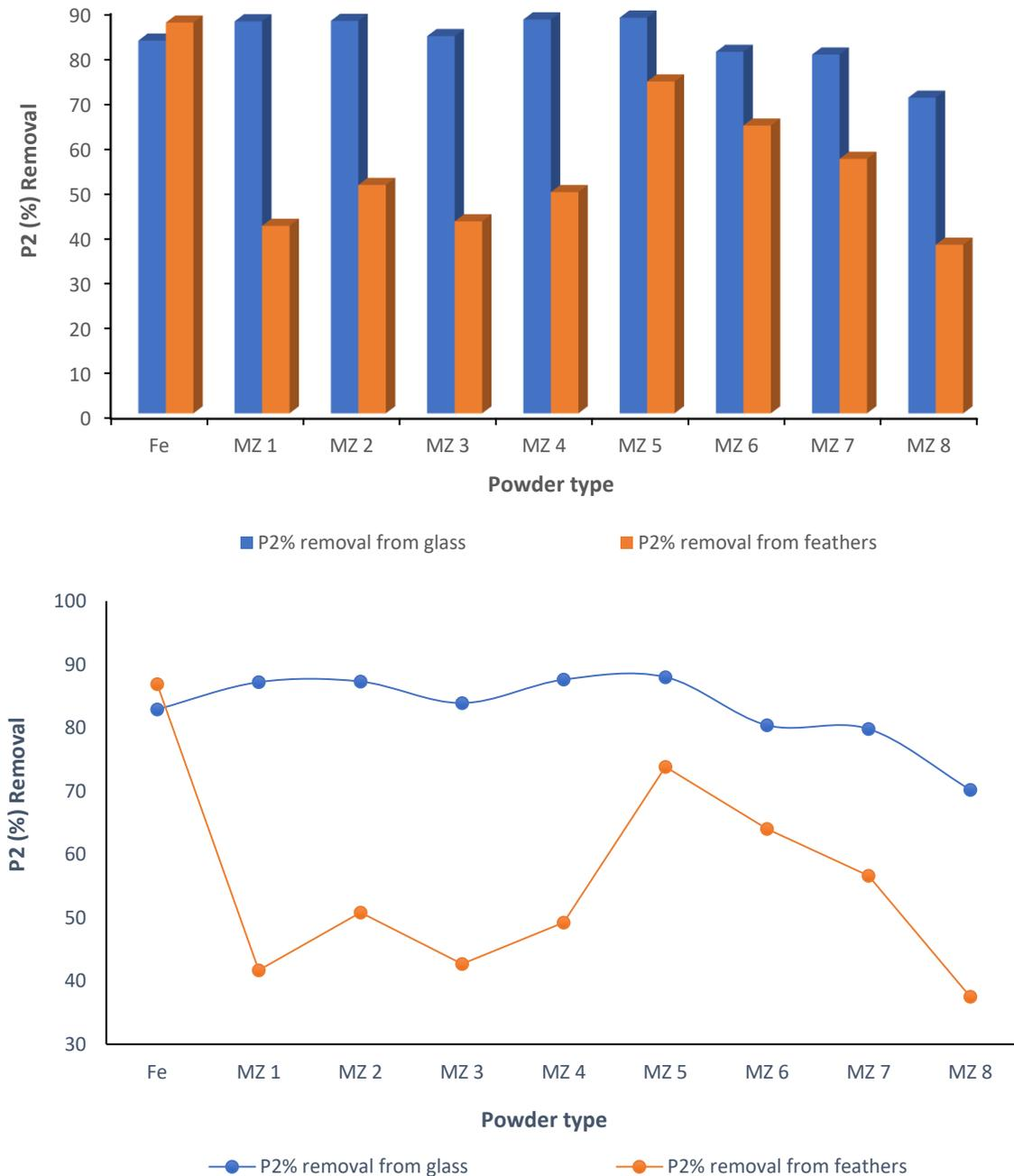
**Figure 3.22:** The P<sub>2</sub>% oil pick-up from glass and feathers for different powder compositions. The line representations of the histograms provided a clearer representation of the trends, especially as to where the maximums occur.
