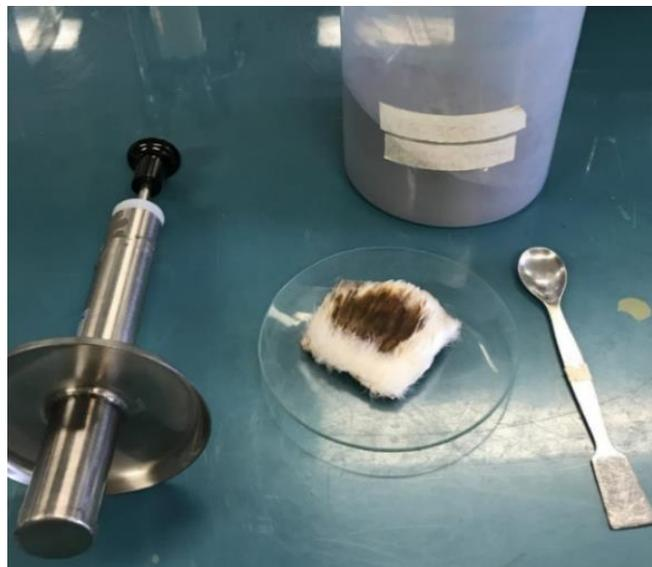
**Figure 4.7:** Magnetic Tester employed for performing MPT oil removal experiments.
