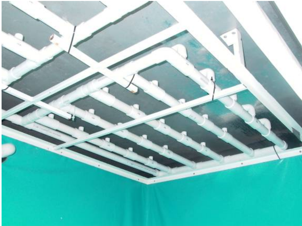
Figure 3.6. A view of the water distribution system from below. It is supported by a light metal frame.
